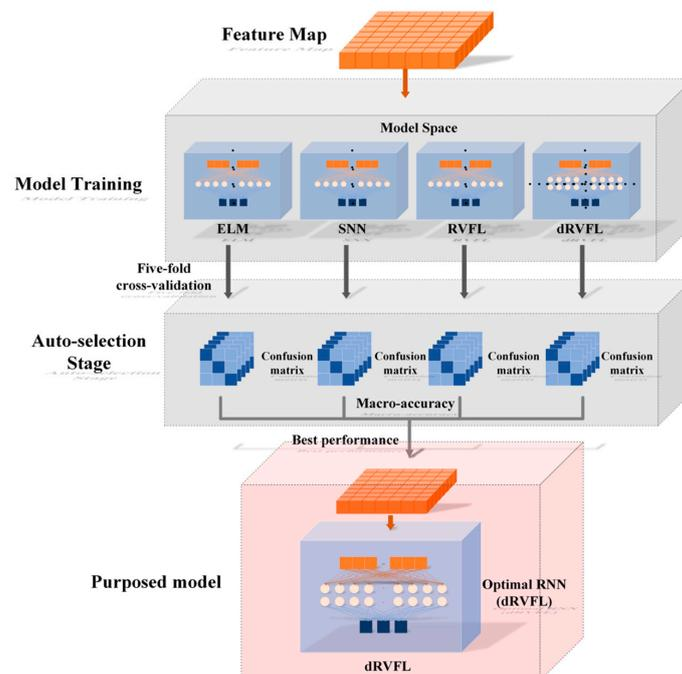
Figure 9. The structure of the feature-based RNN framework.
