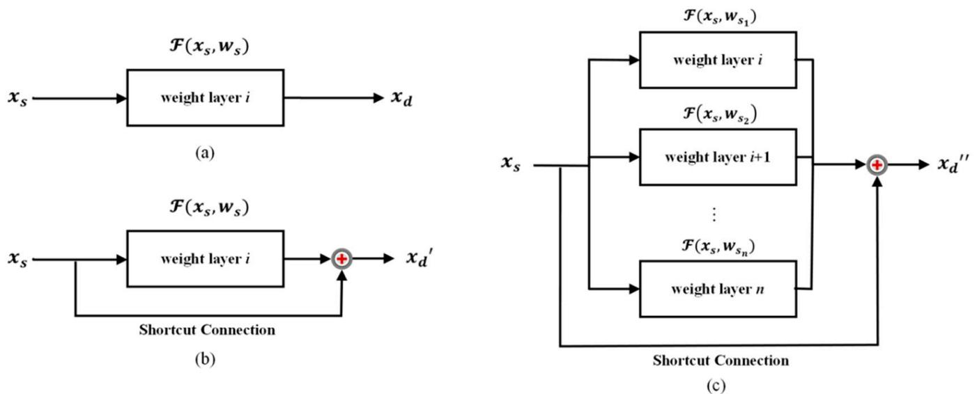
**Figure 2.** Comparison of residual learning with shortcut connections. Given the plain network (a), the single-block residual learning (b) is compared with the multi-block residual learning (c). In particular,  $x_s$  refers to the patterns in shallow layers and  $x_d$  refers to the deep layers. Notably,  $x_d'$  remains in line with  $x_{s+1}$  in Equation (1) and  $x_d''$  with  $x_d$  in Equation (2).
