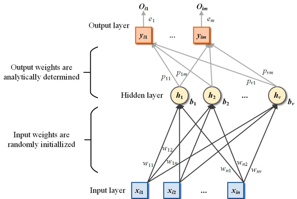
Figure 6. The structure of SNN.
