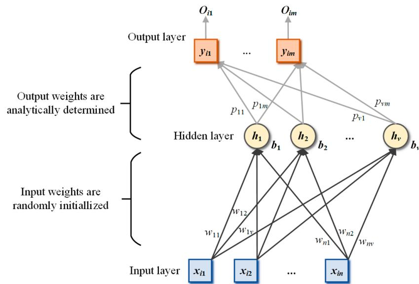
Figure 5. The structure of ELM.
