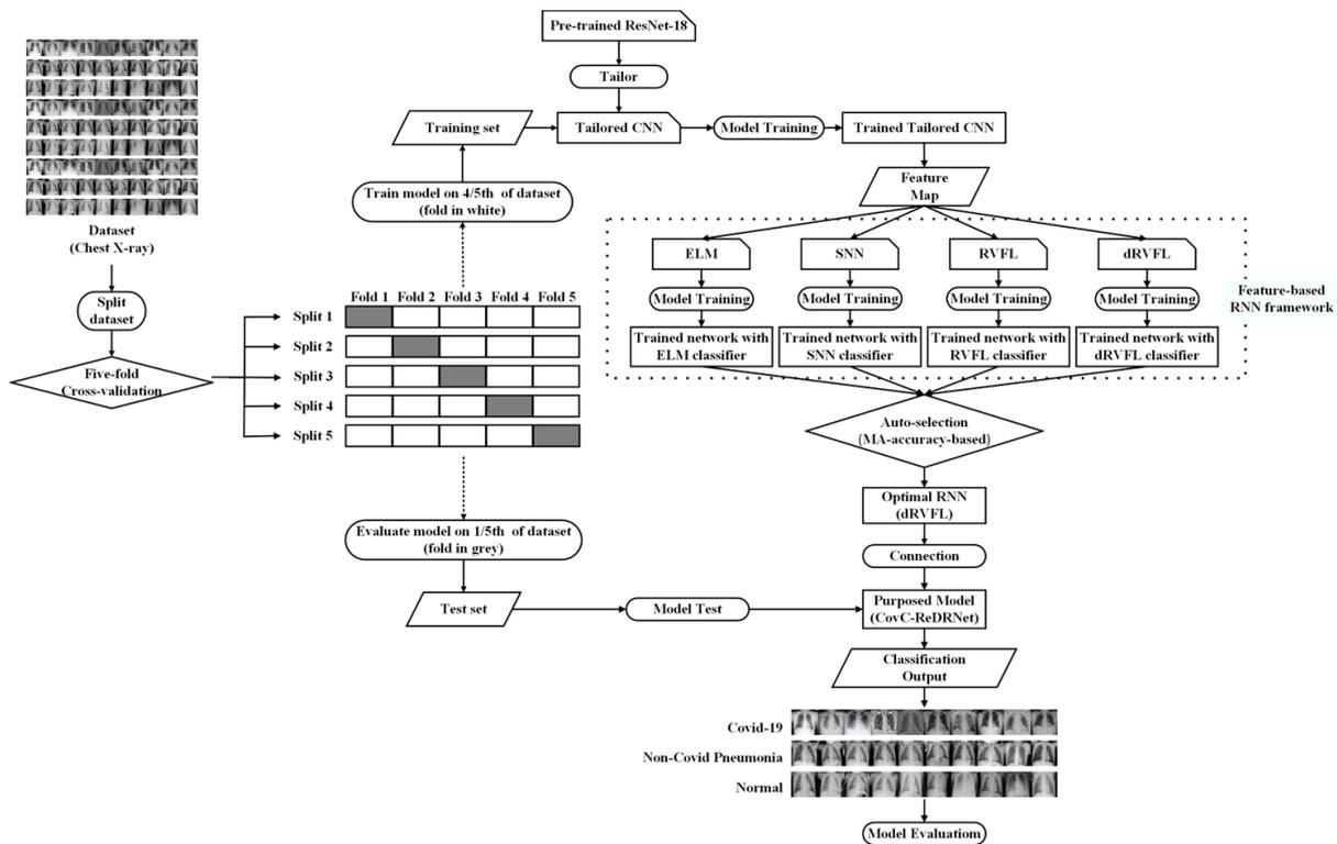
Figure 10. A diagram of the proposed CovC-ReDRNet model.
