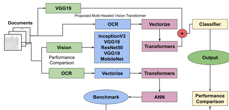
**Figure 1.** The framework workflow includes two key steps: document image classification using transfer learning, followed by OCR and Transformer-based text classification, ultimately integrating vision and OCR for robust classification.
