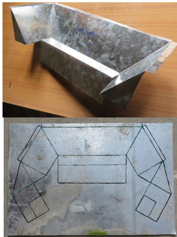
Figure 5. Finished Piece for Solar Cooker (top) and Parametric Sheet Metal Template (bottom).
