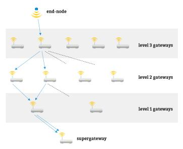
**Figure 3.** A representation of the proposed multilevel architecture in its correct operation. A direct consequence of the network's modus operandi is the redundancy highlighted at the supergateway level.
