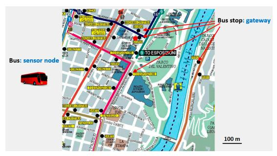
**Figure 1.** Example of tentative installations of gateways on the poles of bus stops for a portion of the city of Turin.
