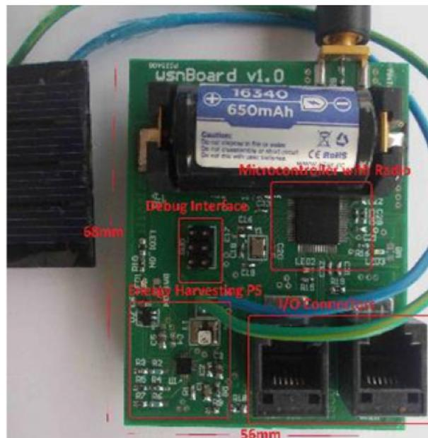
Figure 17. Physical Parts of the IoT node.
