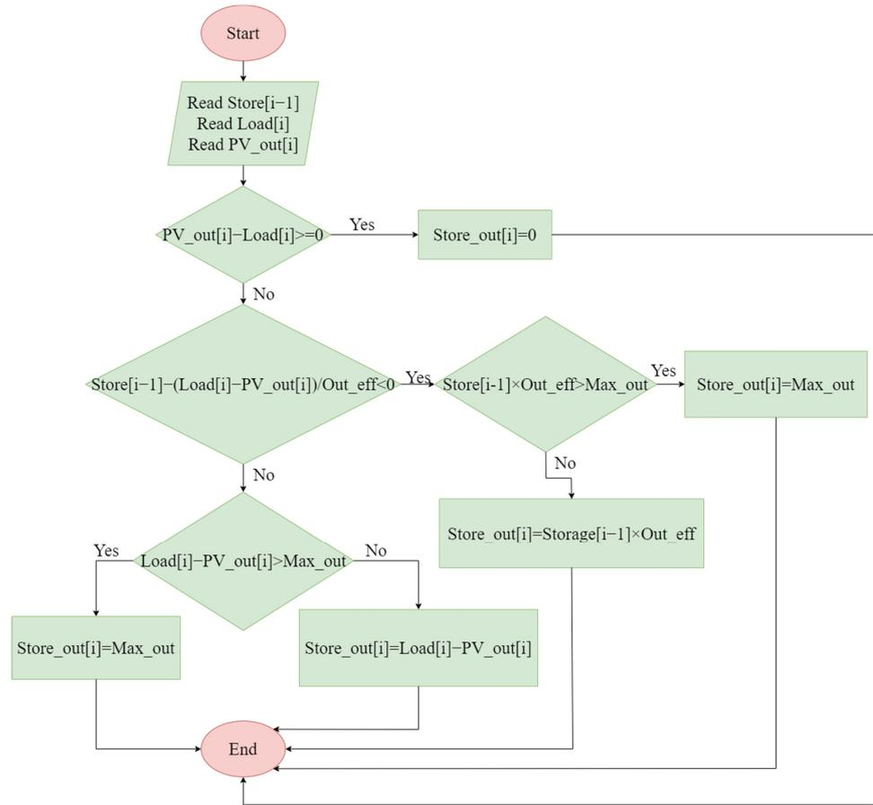
Figure 6. Computation of storage output after each hour.
