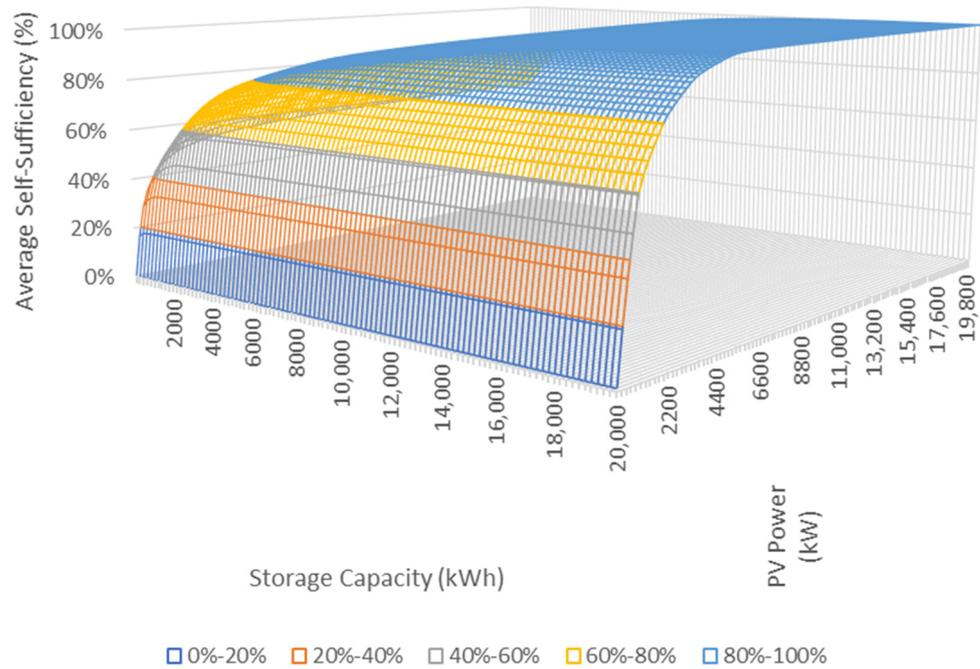
**Figure 13.** Three-dimensional scatter plot of the average annual self-sufficiency for a range of PV power and storage capacity values.
