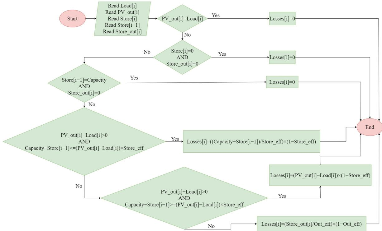
Figure 10. Computation of system losses after each hour.
