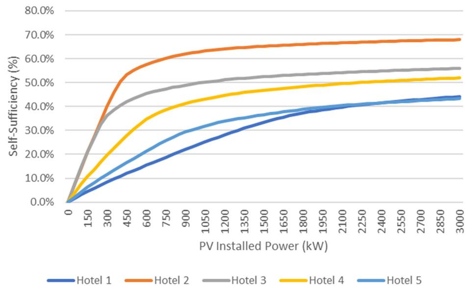
Figure 11. Dependency of self-sufficiency to PV power for the 5 hotels.
