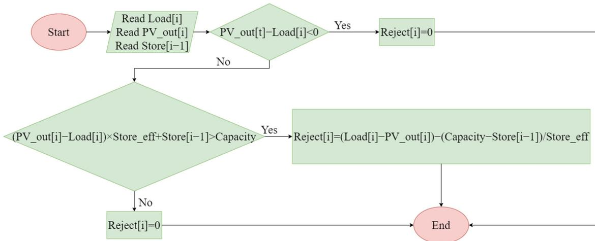
Figure 9. Computation of system rejections after each hour.
