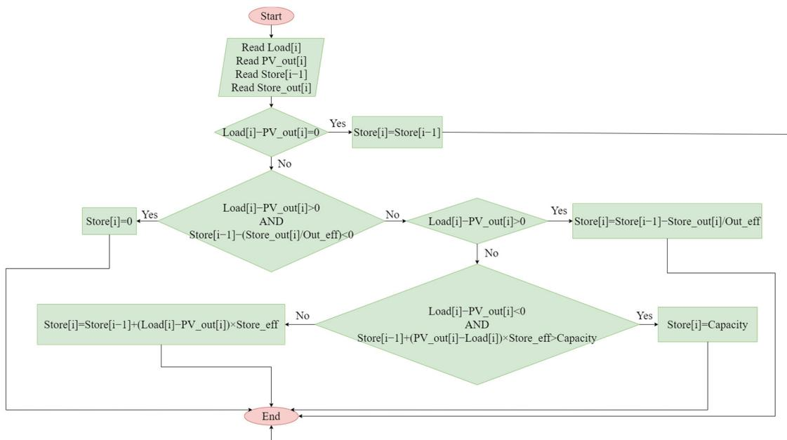
Figure 7. Computation of system storage for each hour.
