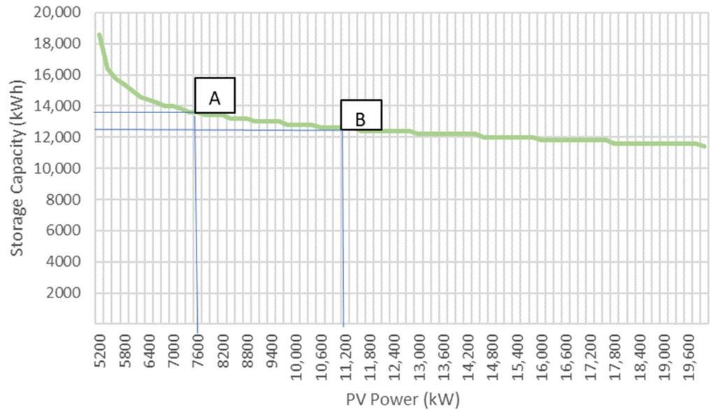
**Figure 14.** Approximation of the separating line between region where self-sufficiency < 99% and self-sufficiency > 99%.
