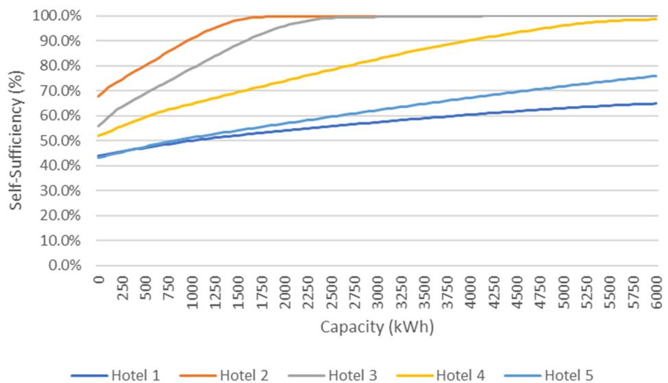
Figure 12. Dependency of self-sufficiency to storage capacity for a fixed PV power value.
