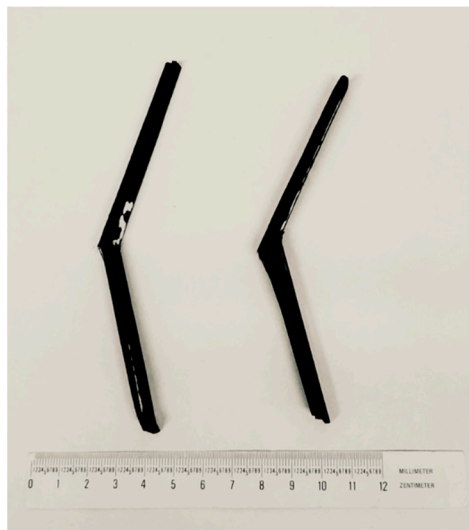
Figure 11. Tested CMC samples from: (left) untreated HM carbon fibers and (right) 3 wt. % SILRES ® MK coated HM carbon fibers.
