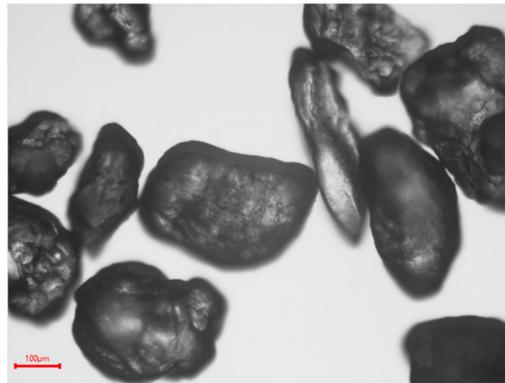
Figure 1. Micrograph of the sand particles used as projectiles impacts.
