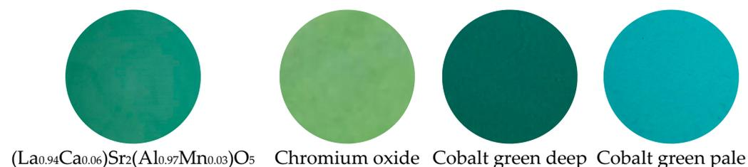
**Figure 10.** Photographs of the pellets of  $(\text{La}_{0.94}\text{Ca}_{0.06})\text{Sr}_2(\text{Al}_{0.97}\text{Mn}_{0.03})\text{O}_5$ , chromium oxide, cobalt green deep, and cobalt green pale powders.
