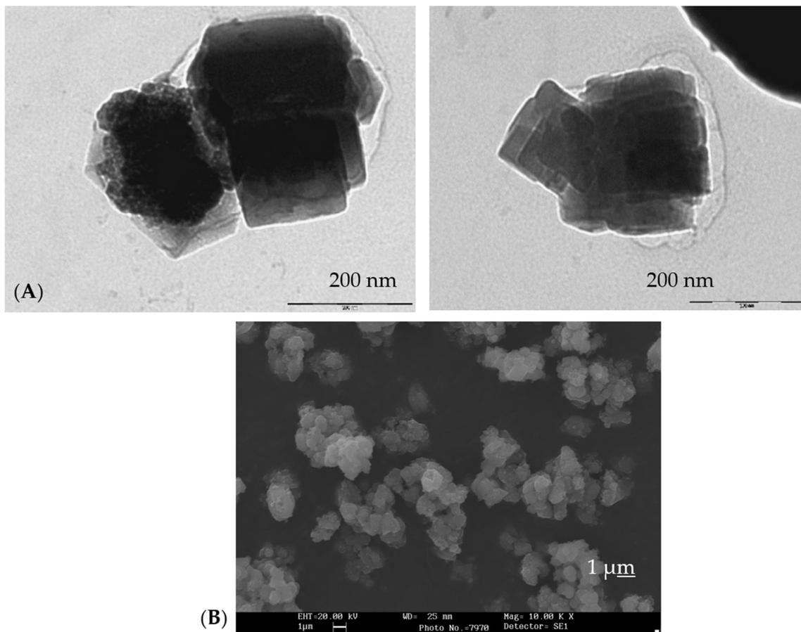
**Figure 13.** (A) TEM micrographs of raw gel nanoparticles of the optimal coprecipitated sample  $\text{Zn}(\text{Al}_{1.3}\text{Cr}_{0.5}\text{Fe}_{0.2})\text{O}_4$ ; (B) SEM micrograph of the same sample fired at  $1000\text{ }^\circ\text{C}$  for 1 h.
