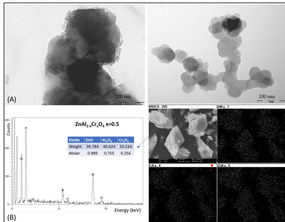
**Figure 9.** (A) TEM micrographs of raw gel of coprecipitated sample  $\text{Zn}(\text{Al}_{2-x}\text{Cr}_x)\text{O}_4$   $x = 0.5$ ; (B) SEM images and EDS composition of global particles and mapping, respectively, of the same sample fired at  $1000 \text{ }^\circ\text{C}$  for 1 h.
