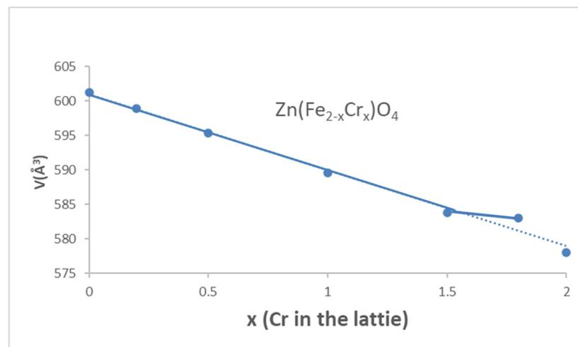
**Figure 3.** Evolution of the volume of the cubic cell of the corresponding spinel  $\text{Zn}(\text{Fe}_{2-x}\text{Cr}_x)\text{O}_4$  solid solution synthesised at 1000 °C for 1 h.
