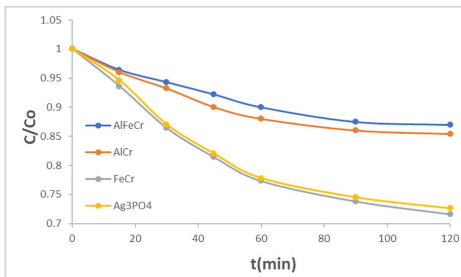
Figure 18. Photodegradation test of Orange II with the optimised powders.
