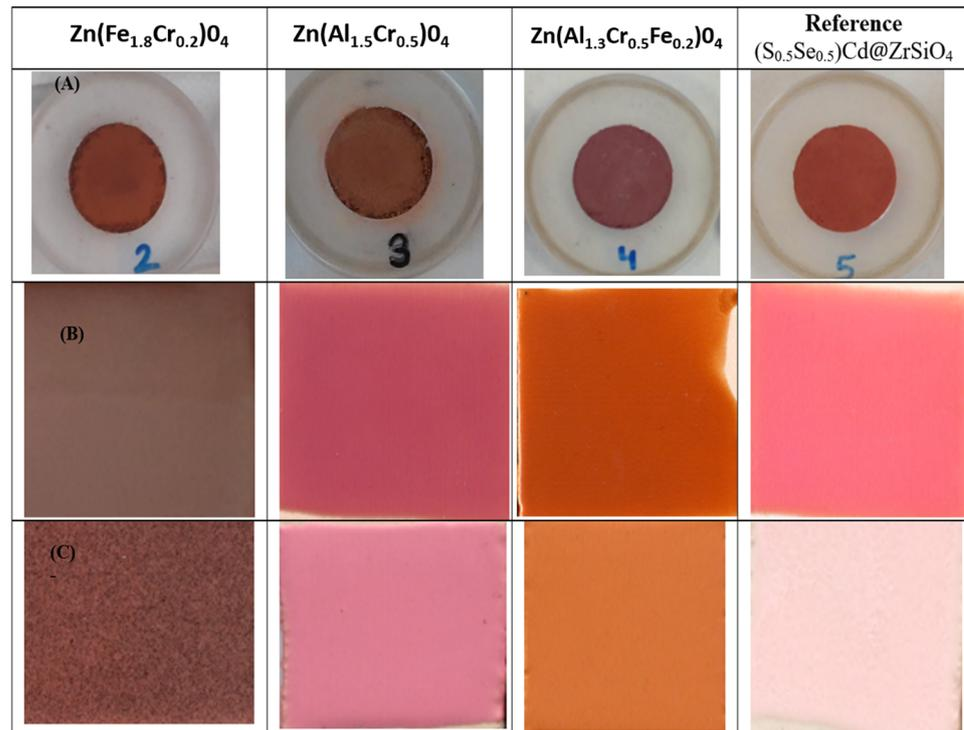
**Figure 14.** Summary of the three reddish optimised samples compared with a commercial cadmium sulfoselenide encapsulated in zircon ( $(S_{0.5}Se_{0.5})Cd@ZrSiO_4$ ): (A) powders, (B) 5 wt.% glazed in single firing frit at 1080 °C, (C) 5 wt.% glazed in porcelain single firing frit at 1200 °C.
