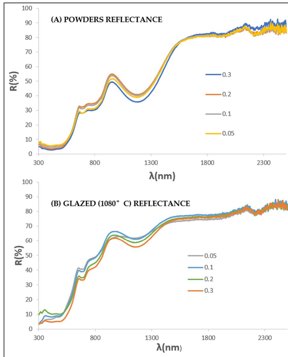
**Figure 12.** UV–Vis–NIR diffuse reflectance spectra of  $\text{Zn}(\text{Al}_{1.5-x}\text{Cr}_{0.5}\text{Fe}_x)\text{O}_4$  coprecipitated samples fired at  $1000\text{ }^\circ\text{C}$  for 1 h: (A) powder, (B) glazed samples in single firing frit at  $1080\text{ }^\circ\text{C}$ .
