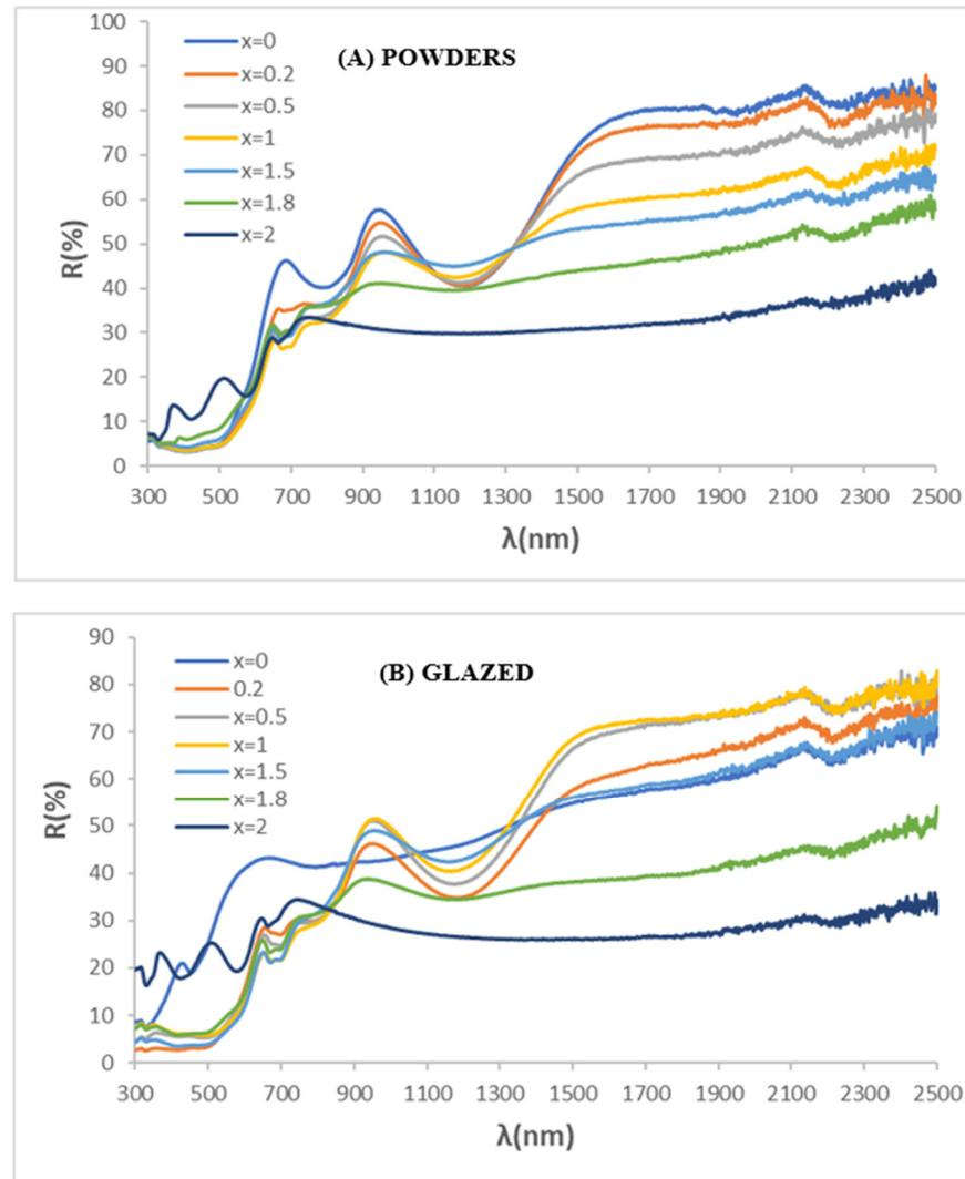
**Figure 4.** UV-Vis-NIR diffuse reflectance spectra of franklinite-zincchromite  $Zn(Fe_{2-x}Cr_x)O_4$  solid solutions: (A) fired powders at 1000 °C for 3 h; (B) 5 wt.% glazed in a single firing frit at 1080 °C.
