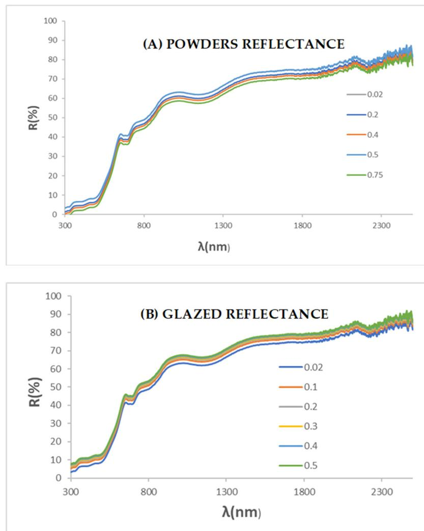
**Figure 8.** UV-Vis-NIR spectra of powders and glazed samples of gahnite-zincochromite  $\text{Zn}(\text{Al}_{2-x}\text{Cr}_x)\text{O}_4$  solid solutions synthesised by ammonia coprecipitation fired at  $1000\text{ }^\circ\text{C}$  for 1 h.
