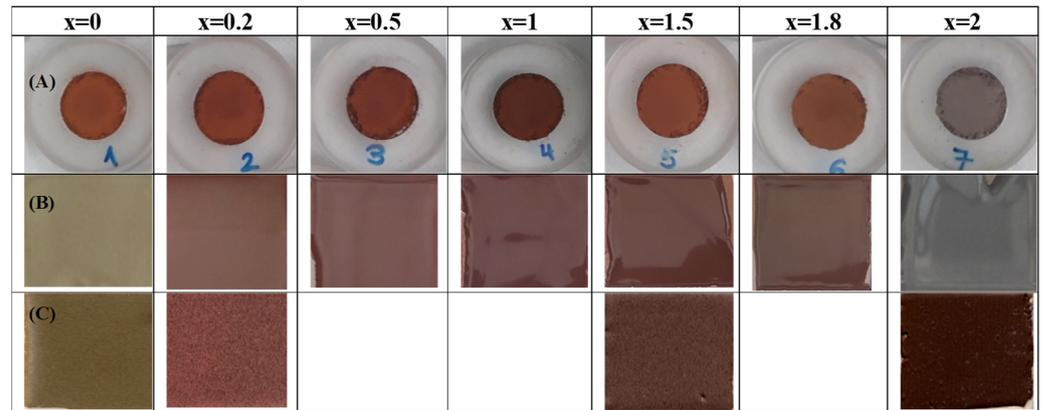
**Figure 1.** Franklinite-zincochromite  $\text{Zn}(\text{Fe}_{2-x}\text{Cr}_x)\text{O}_4$  solid solutions: (A) powders synthesised at 1000 °C for 3 h, (B) 5 wt.% glazed powders in a single firing frit 1080 °C, (C) 5 wt.% glazed powders in a single firing porcelain frit 1200 °C.
