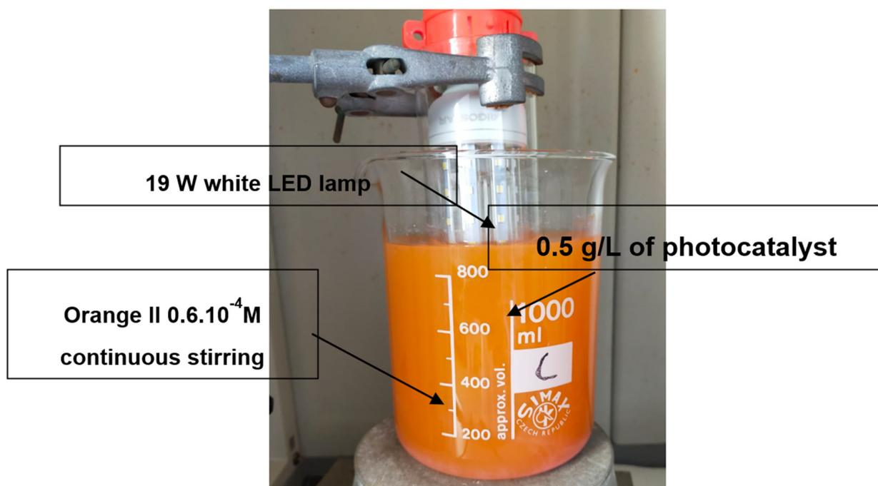
Figure 17. Image of the photoreactor employed and conditions of photodegradation test.
