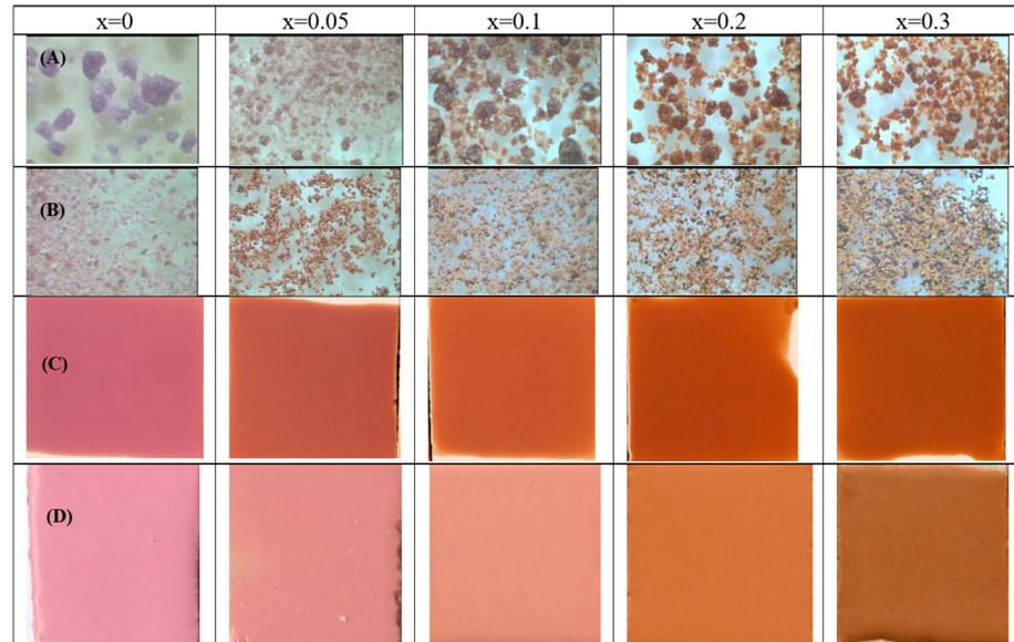
**Figure 10.** Effect of addition of Al and Cr ( $Zn(Al_{1.5-x}Cr_{0.5}Fe_x)O_4$ ): (A) raw dried gels, (B) fired powders at 1000 °C for 1 h, (C) 5 wt.% glazed samples in a single firing frit at 1080 °C, (D) 5 wt.% glazed samples in a porcelain single firing frit at 1200 °C.
