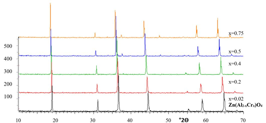
**Figure 6.** X-ray diffractograms (XRD) of gahnite-zincchromite  $\text{Zn}(\text{Al}_{2-x}\text{Cr}_x)\text{O}_4$  solid solutions synthesised at 1000 °C for 1 h with the evolution of the volume of the cubic cell of the corresponding spinel with x.
