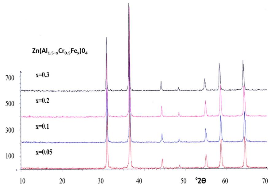
Figure 11. XRD of  $\text{Zn}(\text{Al}_{1.5-x}\text{Cr}_{0.5}\text{Fe}_x)\text{O}_4$  coprecipitated samples fired at 1000 °C for 1 h.
