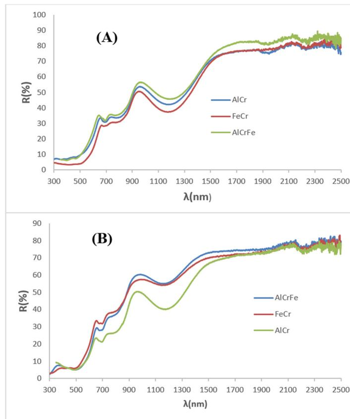
**Figure 15.** UV-Vis-NIR diffuse reflectance spectra of optimised samples: (A) powders; (B) glazed samples in single firing frit.
