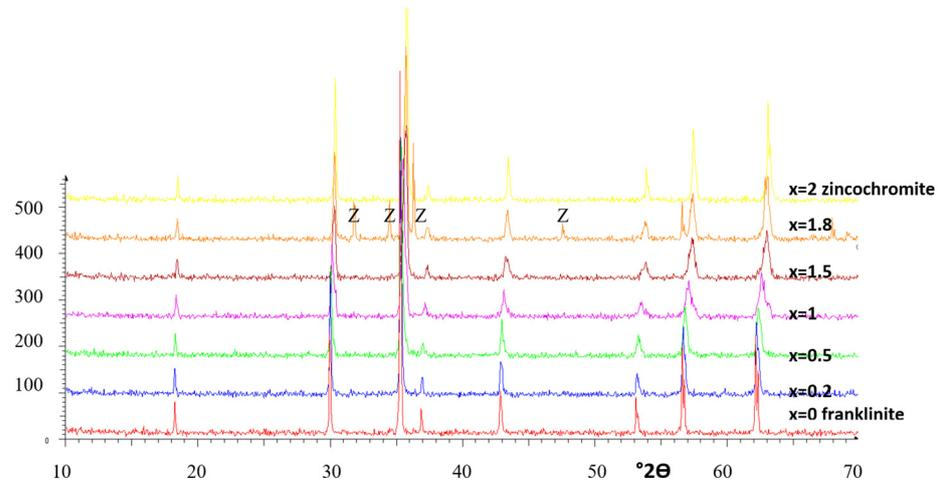
**Figure 2.** X-ray diffractograms (XRD) of franklinite-zincochromite  $\text{Zn}(\text{Fe}_{2-x}\text{Cr}_x)\text{O}_4$  solid solutions synthesised at 1000 °C for 3 h ( $\text{Z}=\text{ZnO}$ ).
