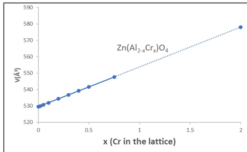
**Figure 7.** Evolution of the volume of the cubic cell of the corresponding spinel  $\text{Zn}(\text{Al}_{2-x}\text{Cr}_x)\text{O}_4$  solid solutions synthesised at  $1000\text{ }^\circ\text{C}$  for 1 h.
