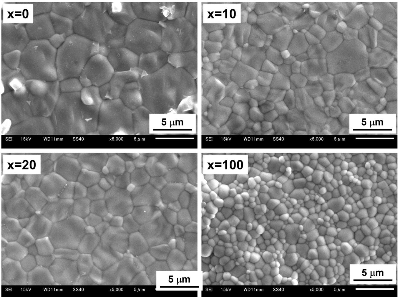
**Figure 4.** SEM images of the surfaces of the BCY-GDC pellets with GDC volume fractions,  $x$ , of 0, 10, 20, and 100 vol% sintered at 1400 °C.
