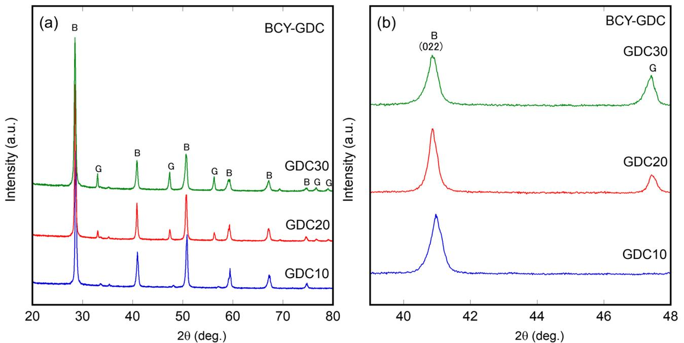
**Figure 2.** XRD patterns of the BCY–GDC pellets with different GDC volume fractions sintered at 1400 °C (a) Diffraction patterns scanned from  $2\theta = 20$  to  $80^\circ$  and (b) magnified images. The notations B and G denote the XRD peaks of the BCY and GDC phases.
