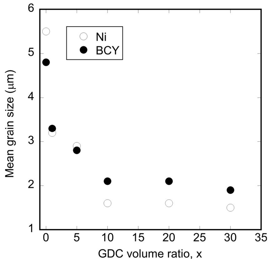
**Figure 8.** Relationship between the GDC volume ratio in Ni–BCY–GDC and the mean grain sizes of Ni and BCY. The grain size was evaluated using the EDS mappings of Ni and Ba collected from the surfaces of the Ni–BCY–GDC pellets.
