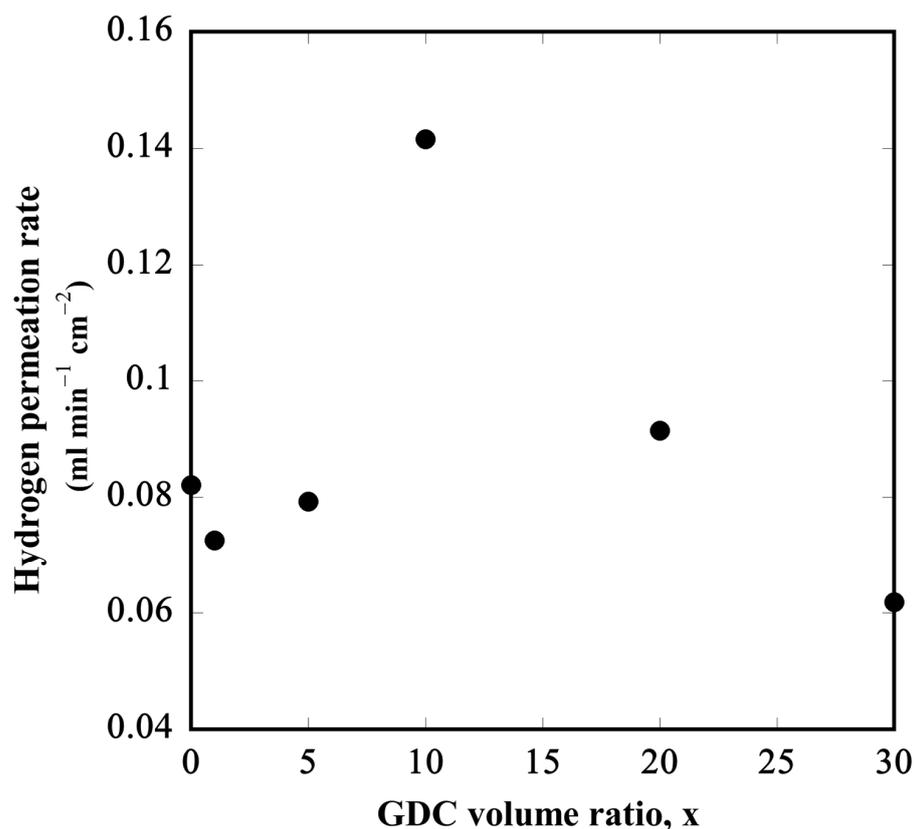
**Figure 12.** Hydrogen permeation fluxes of Ni–BCY–GDC sinters with different GDC volume fractions (x) at 700 °C.
