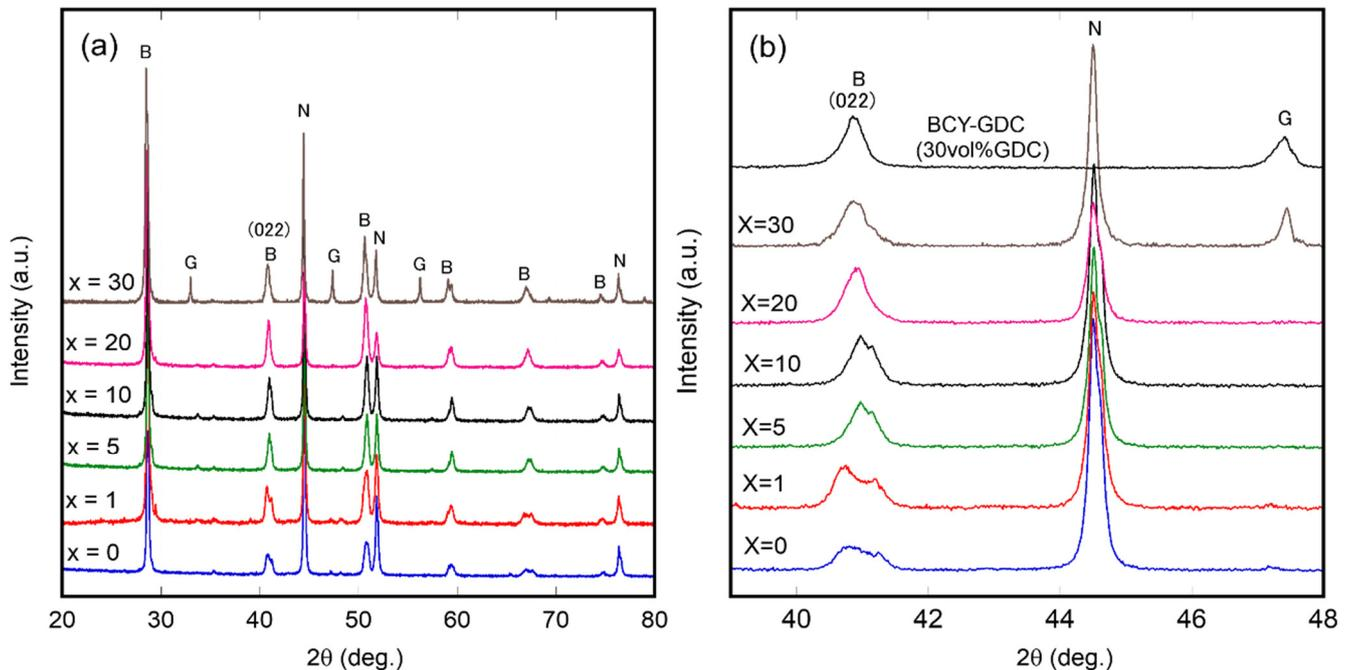
**Figure 3.** XRD patterns of the Ni–BCY–GDC pellets sintered at 1400 °C and reduced by 4% H<sub>2</sub> at 700 °C. (a) Diffraction patterns scanned from 2θ = 20 to 80° and (b) magnified images. The notations B, G, and N denote the XRD peaks of the BCY, GDC, and Ni phases.
