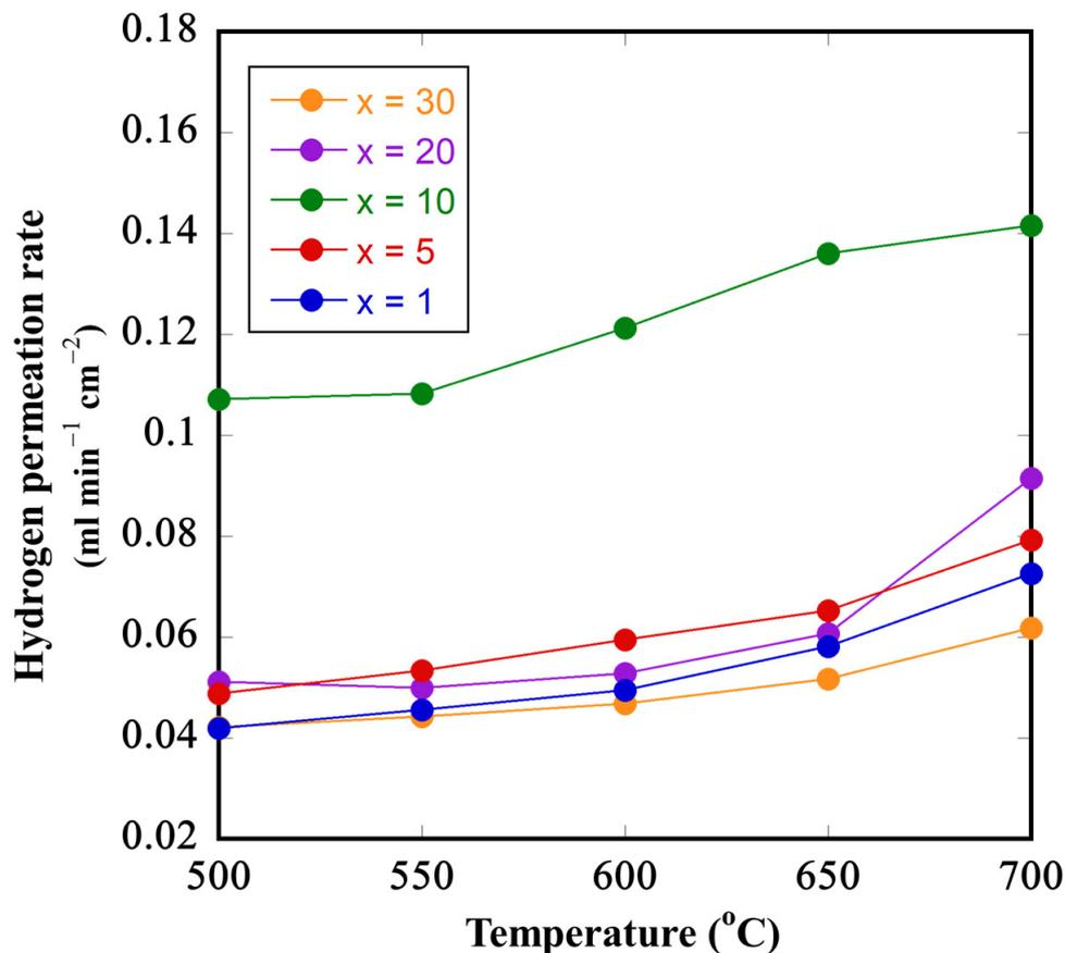
**Figure 11.** Hydrogen permeation fluxes of Ni-BCY-GDC cermets in the temperature range between 500 °C and 700 °C; humidified 4% H<sub>2</sub>/N<sub>2</sub> was fed on one side of the pellets, and humidified N<sub>2</sub>-balanced 100 ppm H<sub>2</sub> was supplied as a sweep gas on the other side.
