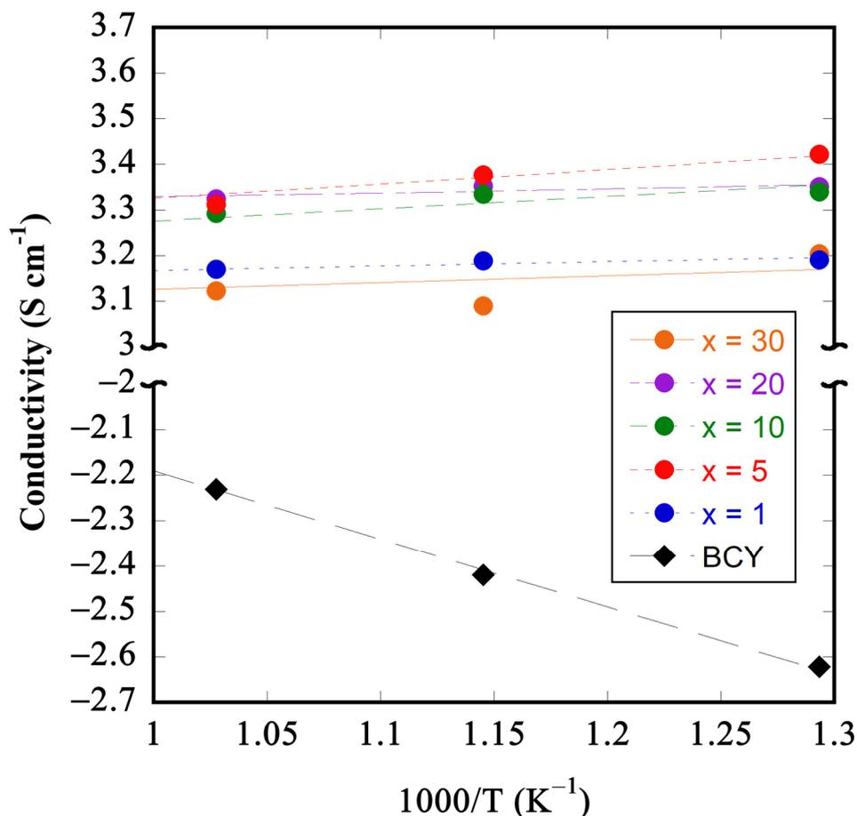
**Figure 10.** Electrical conductivities of sintered Ni-BCY-GDC cermet in 4% H<sub>2</sub>/N<sub>2</sub> were measured using the four-terminal DC method. For BCY, the conductivity was measured using the two-terminal AC method.
