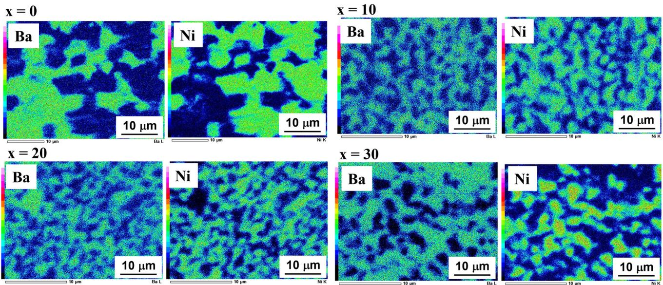
**Figure 7.** EDS elemental mappings of Ba and Ni collected from the surface of the Ni-BCY-GDC pellets ( $x = 0$ – $30$ ) sintered at  $1400\text{ }^{\circ}\text{C}$  and reduced in  $\text{H}_2$  at  $700\text{ }^{\circ}\text{C}$ .
