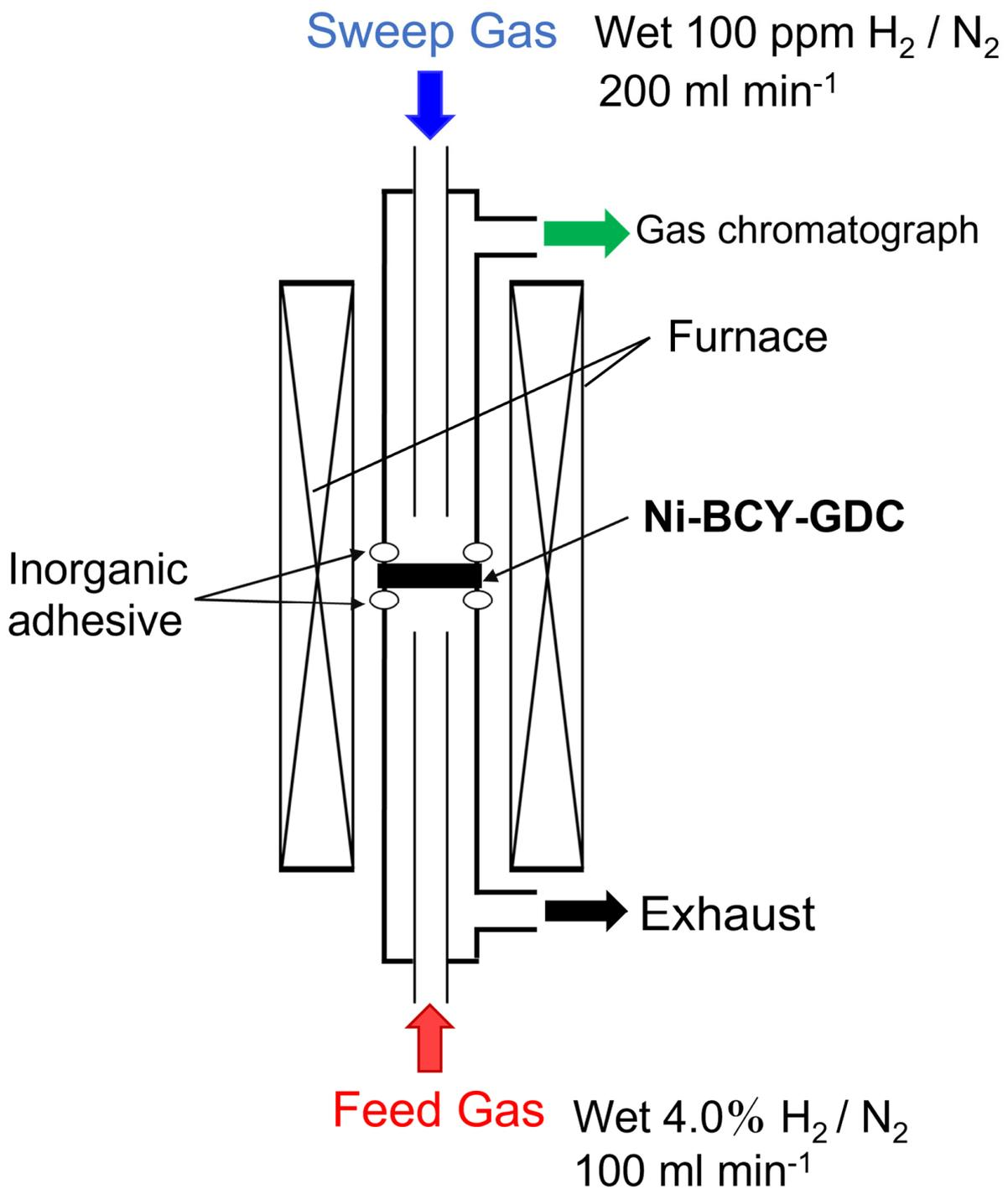
**Figure 1.** Experimental setup for hydrogen permeation tests.
