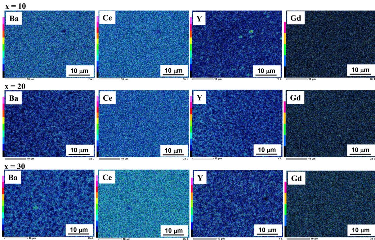
**Figure 5.** EDS elemental mappings of the surface of BCY-GDC pellets with GDC volume fractions,  $x$ , of 10, 20, and 30 vol% sintered at 1400 °C.
