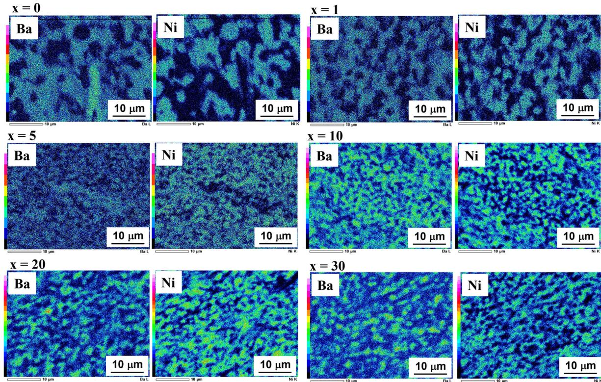
**Figure 6.** EDS elemental mappings of Ba and Ni collected from the cross-section of the Ni-BCY-GDC pellets ( $x = 0-30$ ) sintered at 1400 °C and reduced in  $H_2$  at 700 °C.
