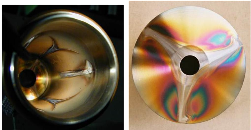
**Figure 3.** Erosion marks after some operating time. Left: Interior of the PC, showing the six loss lines and the region where the radial component of the hexapole field adds to the stray field of the mirror. Right: plasma electrode (plasma side) with extraction aperture, showing three of six loss lines. Note that these loss lines are generated by plasma losses.
