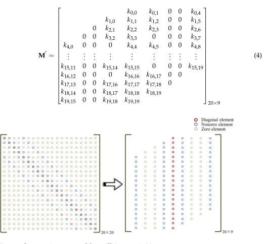
matrix  $\mathbf{M}$  is compressed into a new matrix  $\mathbf{M'}$  of 20 rows and 9 columns, as expressed in Equation (4).
