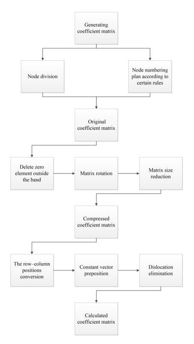
Figure 5. Flowchart of the compressed storage and solution method.
