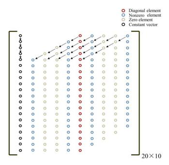
Figure 7. Elimination process of the augmented matrix A.
