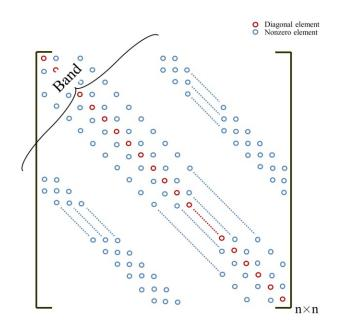
Figure 4. General form diagram of the coefficient matrix.
