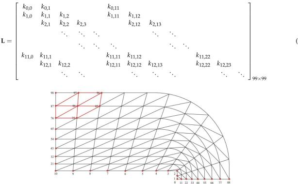
Figure 2. Mesh generation of the model of heat emitting from a surrounding rock at the drifting face.
