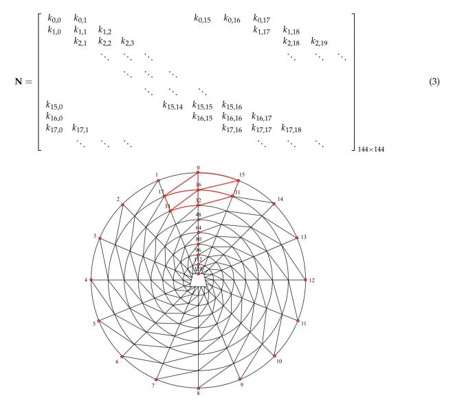
**Figure 3.** Mesh generation of the model of surrounding rock heat dissipation for trapezoid roadways in a coal mine.
