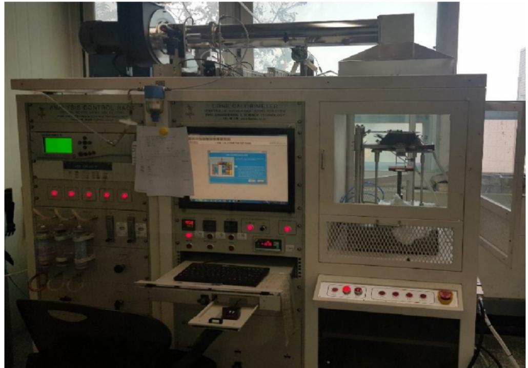
**Figure 2.** Setup of the cone calorimeter test.
