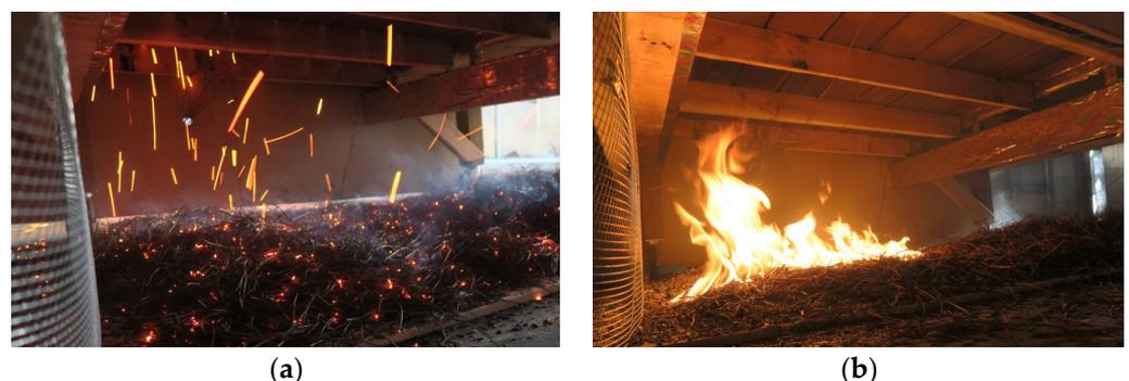
**Figure 12.** (a) Embers dropping between the boards gaps. (b) Embers igniting the pine needles and causing under-deck flame impingement.
