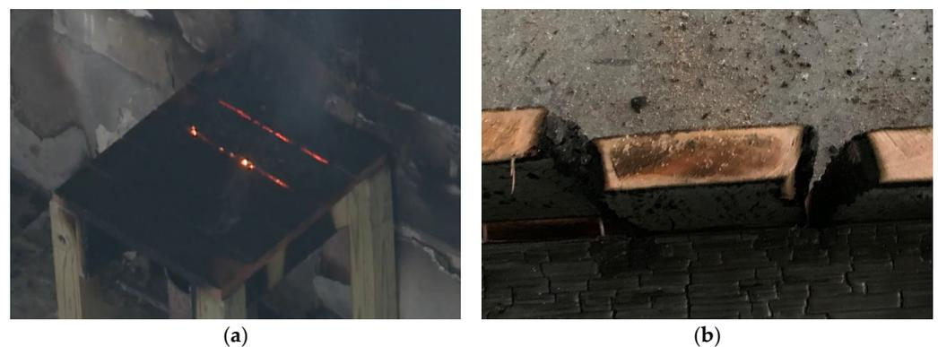
**Figure 13.** Replicating the current test method. (a) Fire intensity after 15 min (12 min after shutting off the gas burner). (b) Cross-section of the burned deck.
