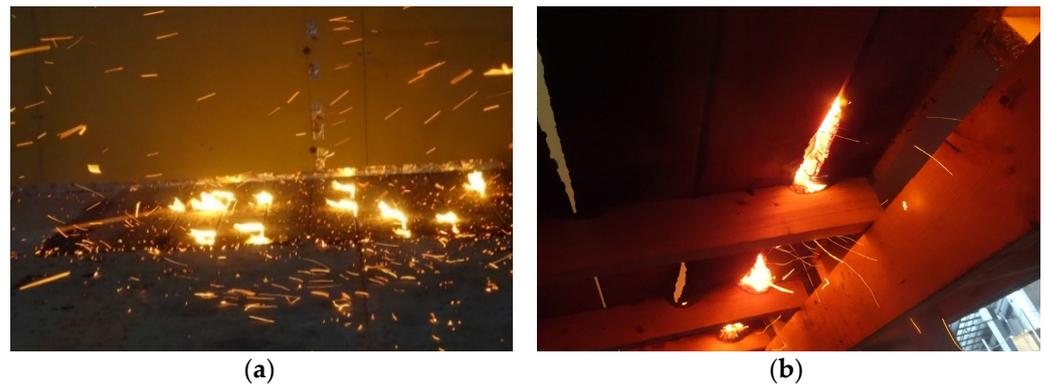
**Figure 9.** Flame height between the deck boards from (a) above and (b) below.
