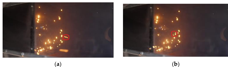
Figure 9. Shows splitting mechanism, (a) approaching firebrands, (b) firebrands split into three smaller glowing firebrands at approaching side of the screen (Stainless Steel Wire and Mesh Pty Ltd. [17]).
