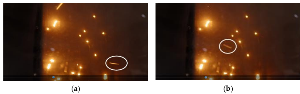
Figure 7. A firebrand passes through the mesh without any contact, (a) approaching firebrand, (b) firebrands after passing the mesh (Stainless Steel Wire and Mesh Pty Ltd. [17]).
