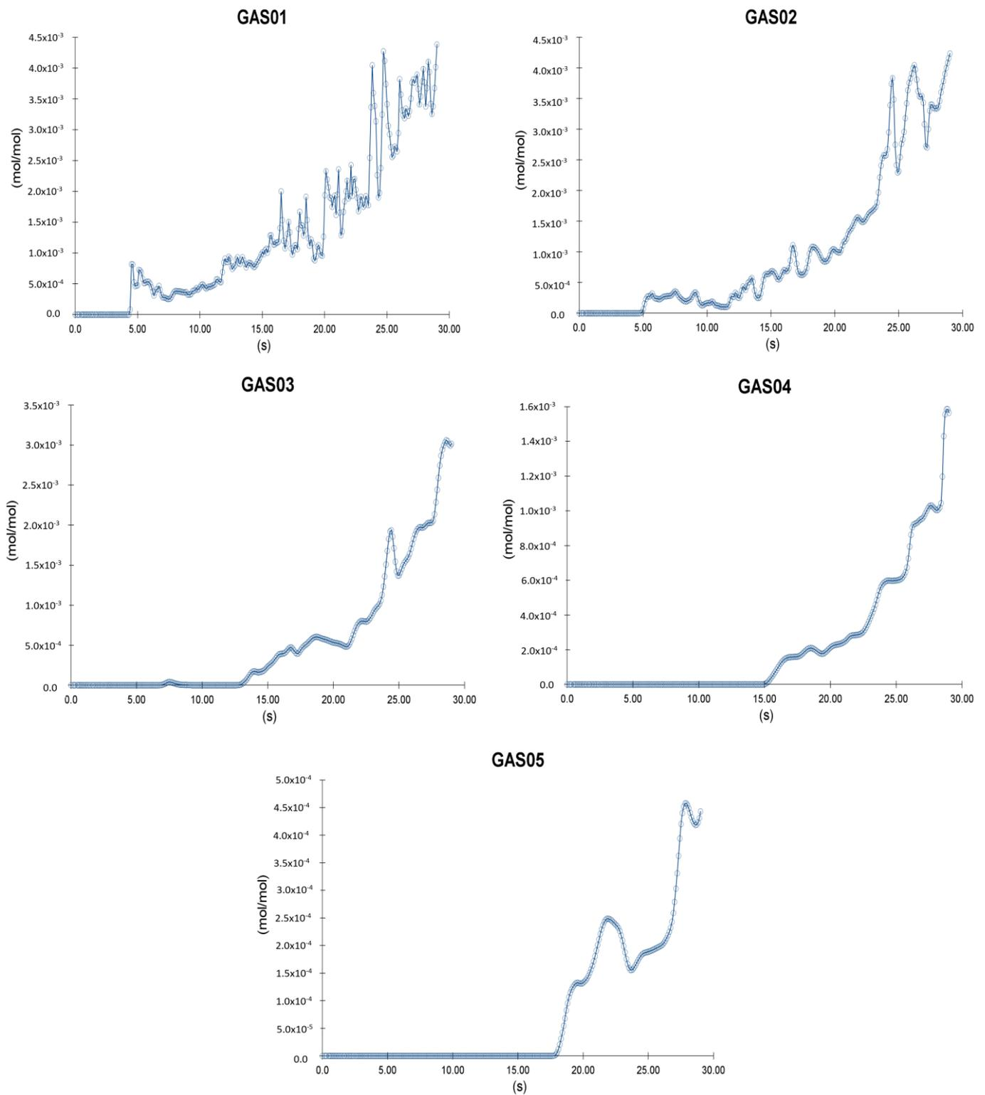
Figure 12. CO volume fraction diagrams.
