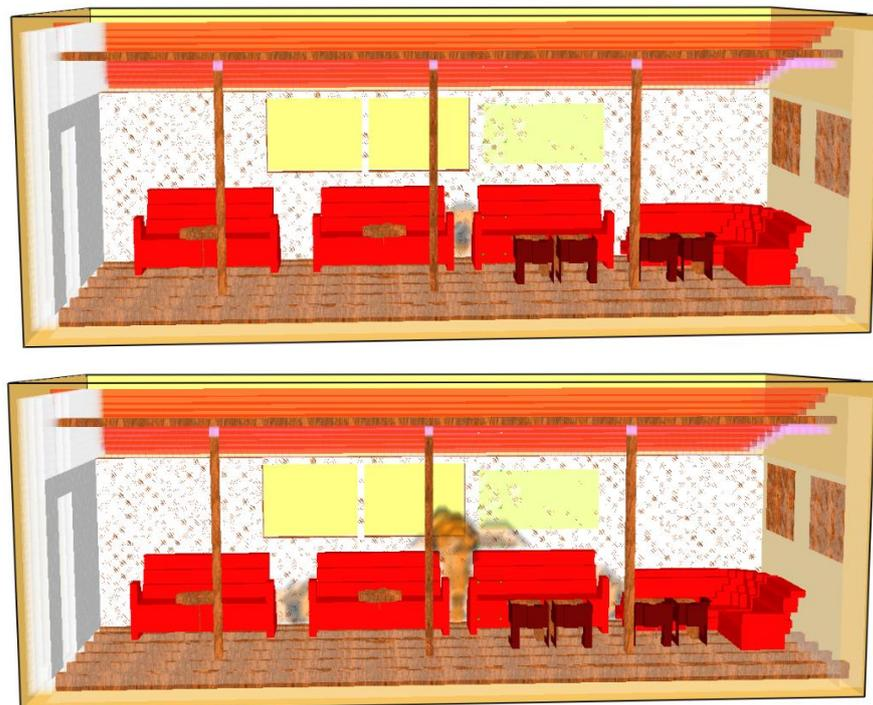
**Figure 6.** The fire ignites the floor's wooden support beam and spreads into the first level of the restaurant lounge.
