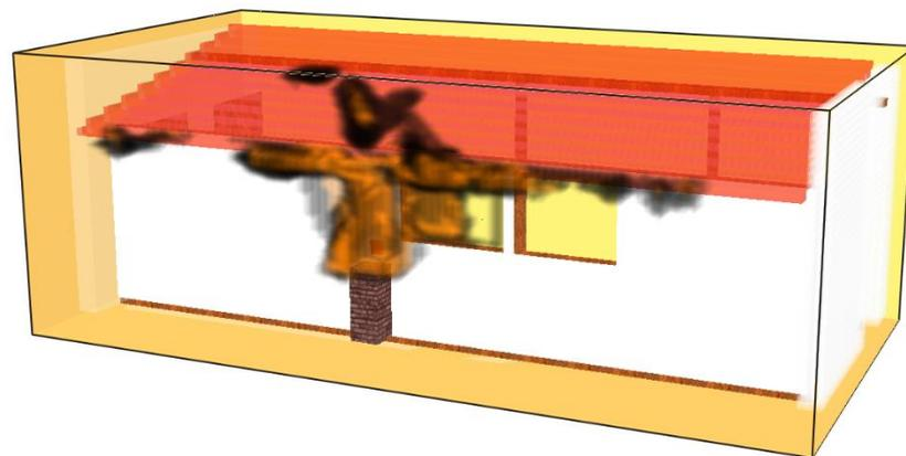
**Figure 14.** The spread of the fire on the outside of the eastern wall of the floor, favored by the combustible properties of the polystyrene insulation.
