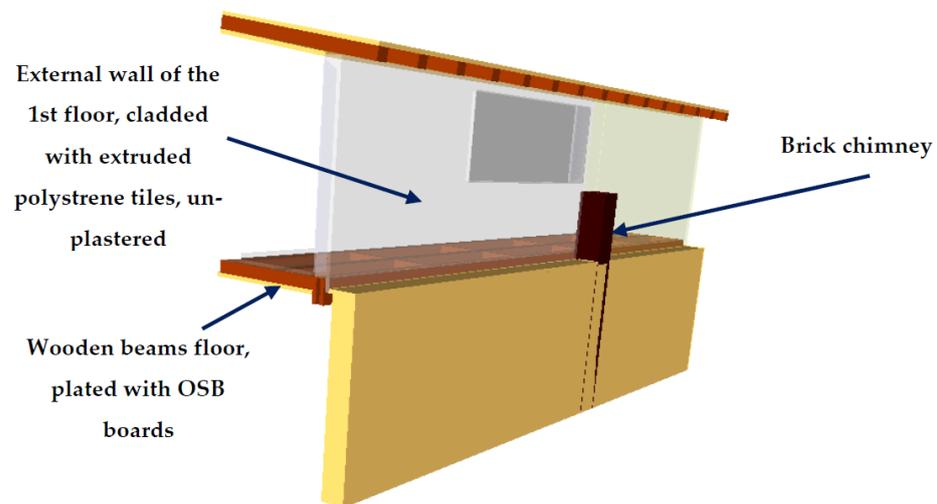
**Figure 4.** Building section (ground floor and first floor), eastern wall. Hypothesis (2).
