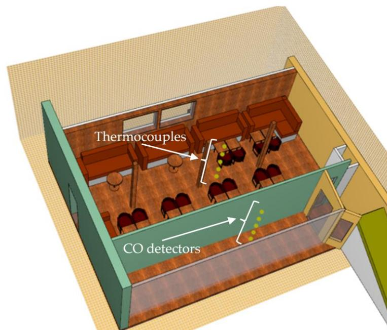
**Figure 5.** The virtual model of the geometry used for fire simulation (the 1st floor of the restaurant).
