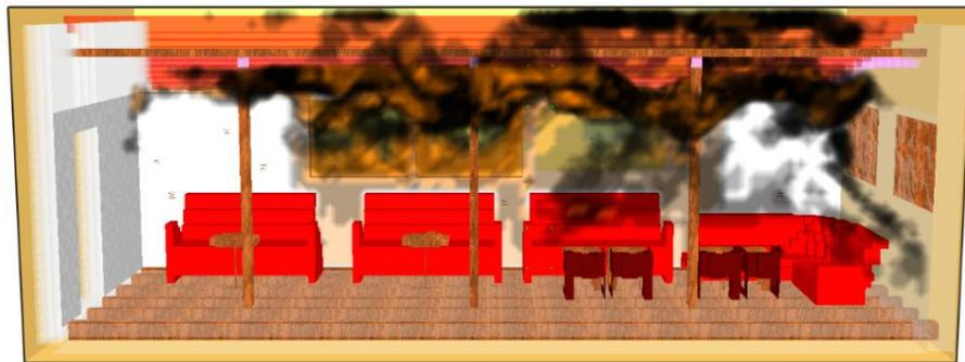
Figure 9. Combustion of furniture by thermal radiation and hot gases.
