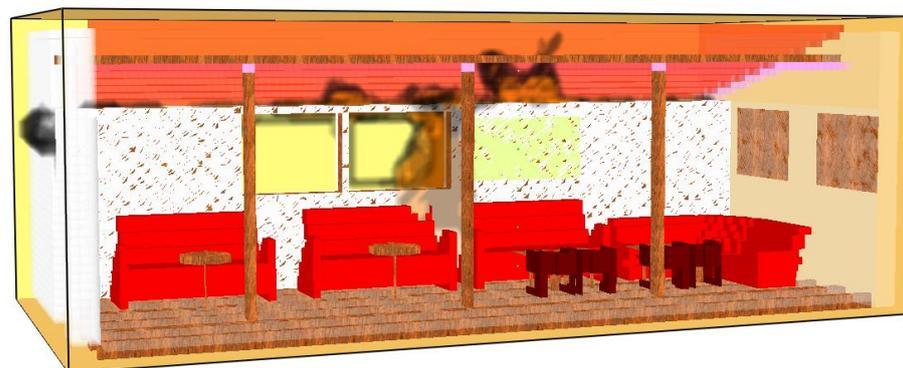
**Figure 15.** The spread of the fire inside the restaurant floor, through the window, and the ignition of the furniture in the room (sofas located nearby windows).
