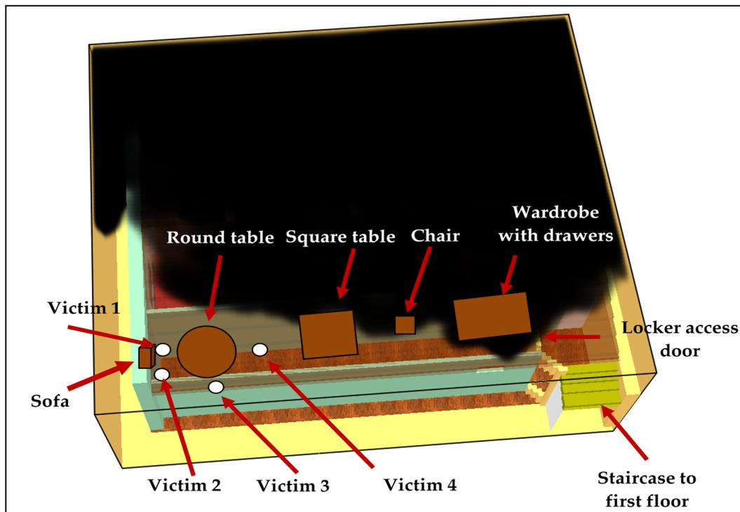
**Figure 19.** The advance of smoke and toxic gases from the wall with the fire source towards the locker room and the access staircase to the first floor.
