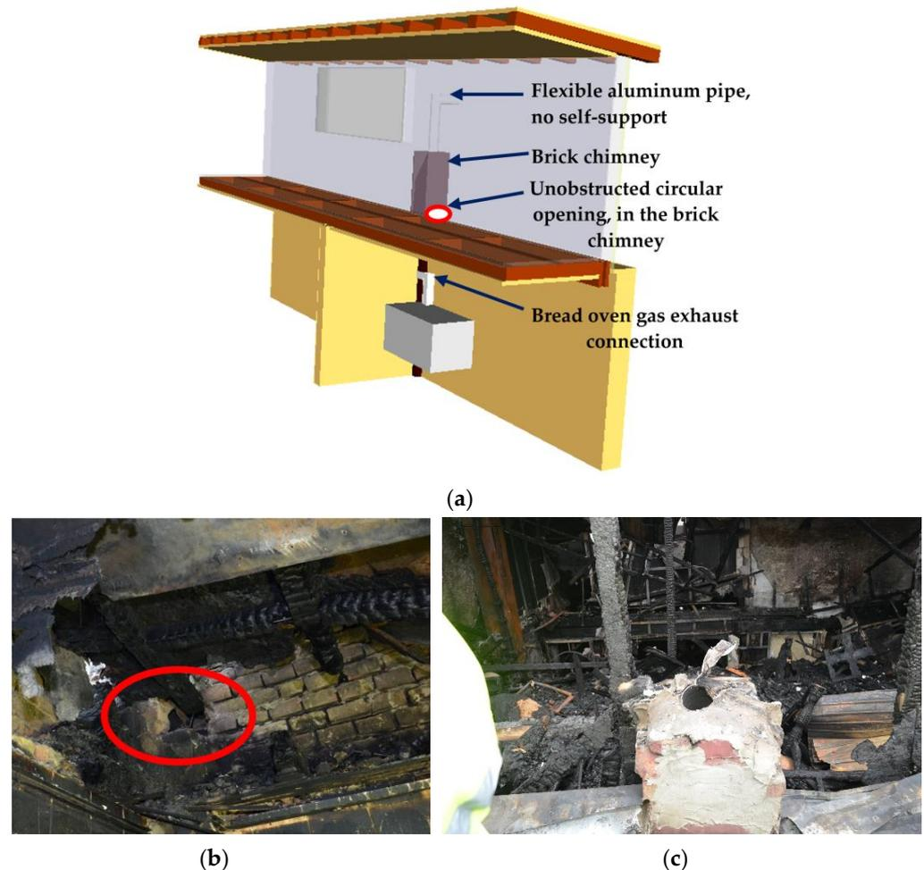
**Figure 3.** Hypothesis (1). Building section (ground and first floor), eastern wall (a); details of the unobstructed hole in the brick chimney (b); upper limit of the chimney with flexible aluminum tube extension (c).
