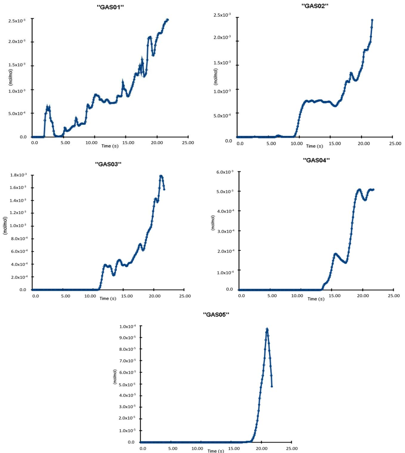
**Figure 18.** CO volume fraction diagrams (mol/mol).
