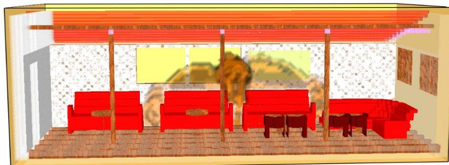
**Figure 7.** Fire developing on the inside of the eastern wall.
