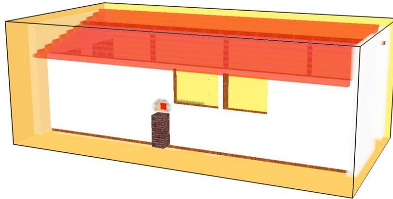
**Figure 13.** Ignition of the eastern wall cladding with extruded polystyrene due to the incandescent flour particles emitted through the flexible aluminum tube without self-support or extension of the brick chimney.
