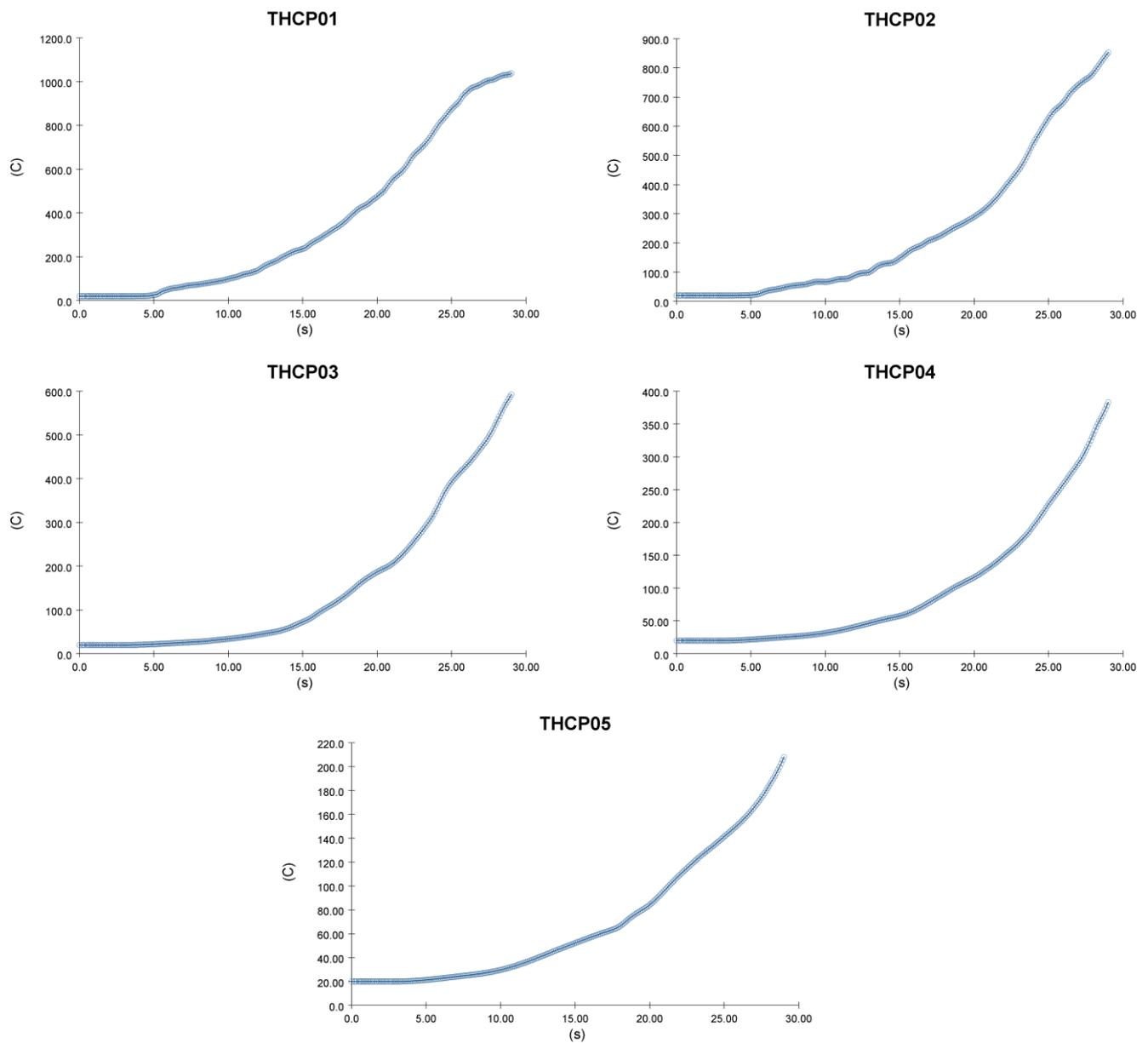
**Figure 11.** Room temperature evolution in time in the first 30 s of fire simulation (Hypothesis 1).
