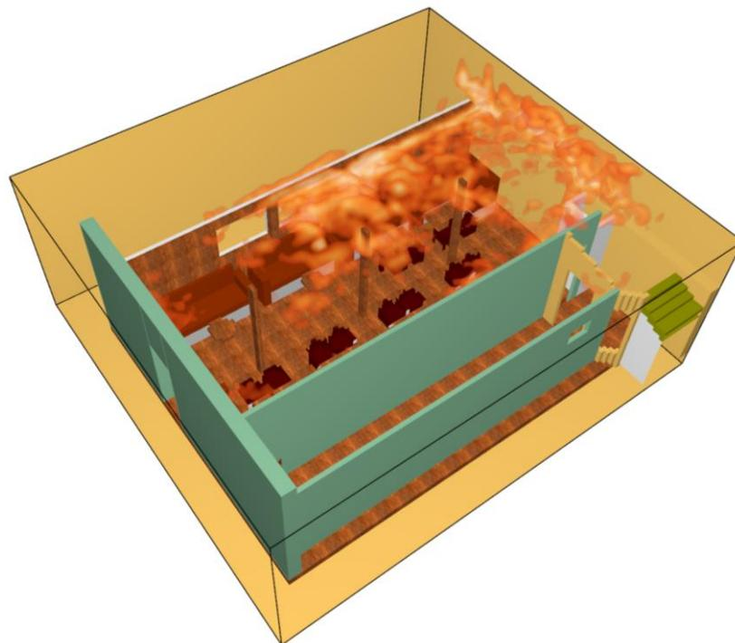
Figure 10. Generalization of the fire at the entire level of the 1st floor.
