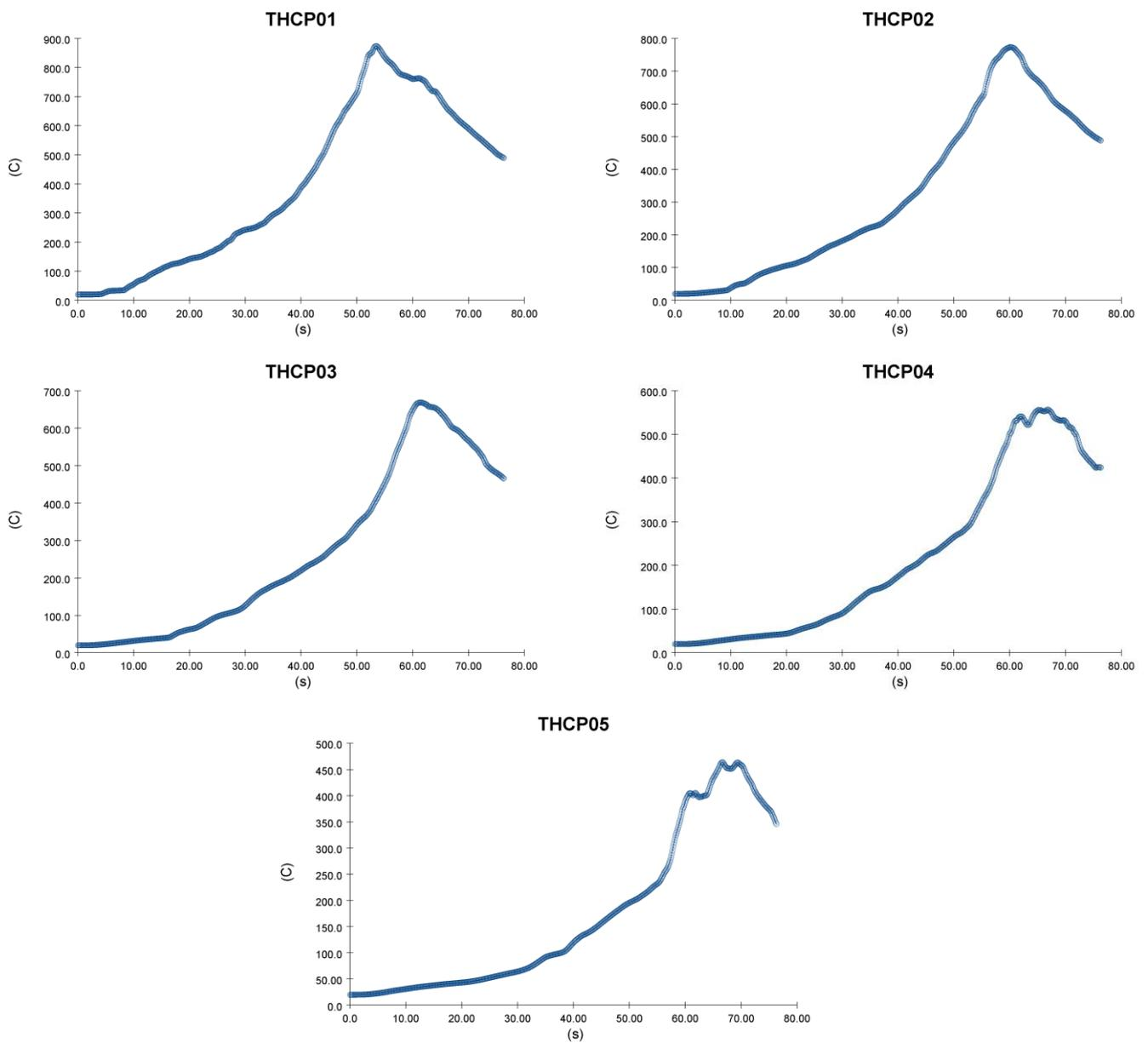
Figure 17. Room temperature evolution in time, in the first seconds of the fire simulation (Hypothesis 2).
