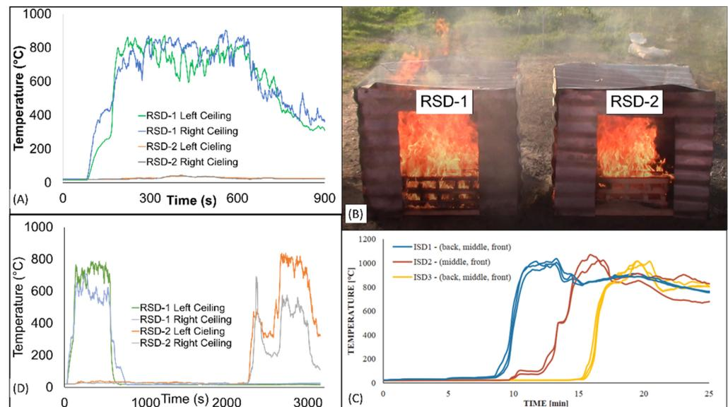
**Figure 6.** Longitudinal fire spread results. Left top clockwise—(A) Test 2: ceiling temperature on cross wind condition, (B) RSEs on steel-clad dwellings, (C) FSE results on steel-clad dwelling [7], (D) test 3: ceiling temperature on circular wind condition.
