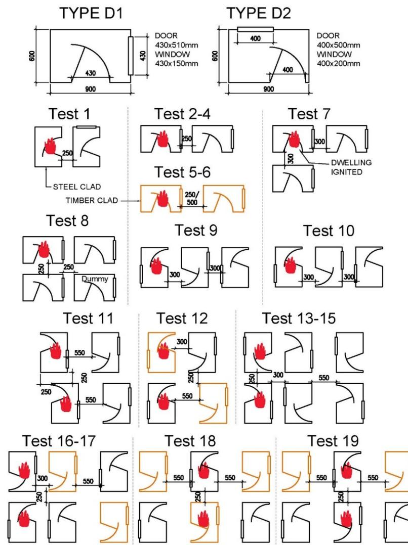
**Figure 4.** Pictorial representation of 19 test setups showing dwelling layouts (top) and test setups. Steel-clad dwellings are shown in black, timber-clad dwellings in brown and ignited dwellings with the fire symbol.
