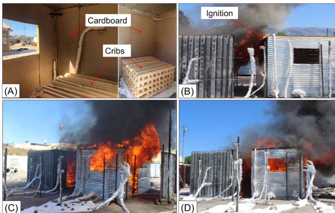
**Figure 1.** The effect of separation distance between informal dwellings on fire spread rates (A) Interior and wood crib arrangement; (B) ignition from ISD1 to ISD2; (C,D) fire spread between dwellings at 1 m and 1.75 m [9].
