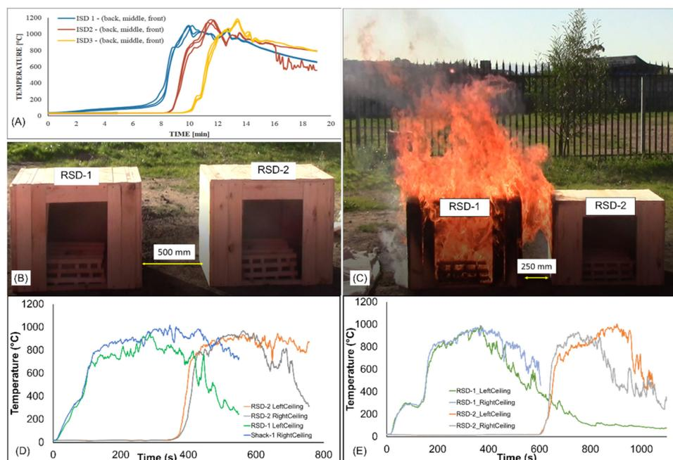
**Figure 7.** Results from various multi dwelling tests. Clockwise—(A) FSE results on timber-clad dwelling [7], (B) test 6: RSEs on timber-clad dwellings at 500 mm, (C) test 5: RSEs on timber-clad dwellings at 250 mm, (D) test 6: ceiling temperature in timber-clad dwelling placed at 500 mm, (E) test 5: ceiling temperature in timber-clad dwelling placed at 250 mm.
