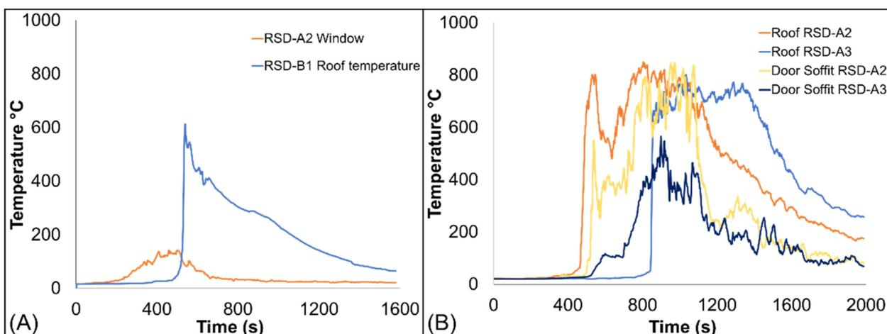
**Figure 9.** Three RSD experiment: (A) test 7: fire spread by RSD-01; (B) test 10: roof temperatures and door soffit temperatures.
