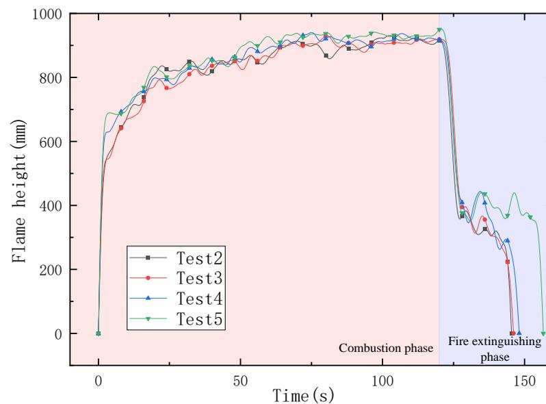
**Figure 4.** Average flame height under different nitrogen injection flow rates.
