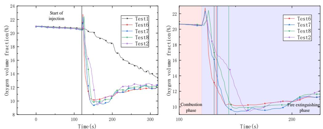
Figure 9. Comparison of oxygen volume fractions around the fire source.
