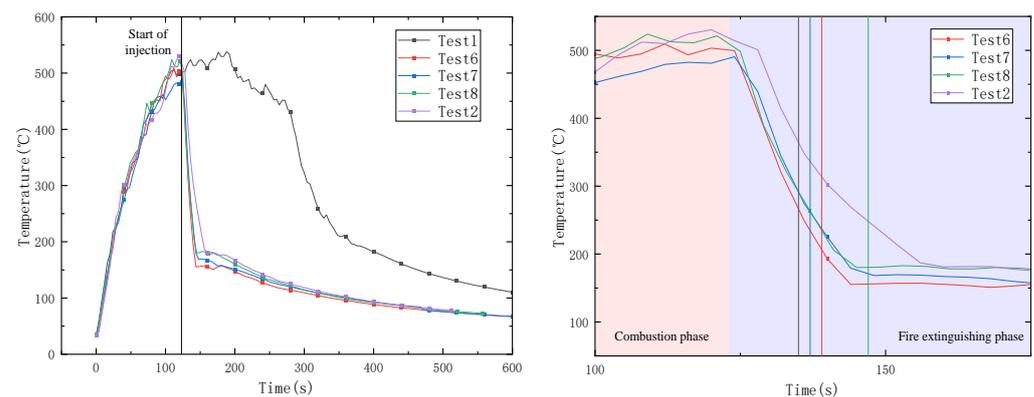
**Figure 8.** Temperatures above the fire source under different conditions.
