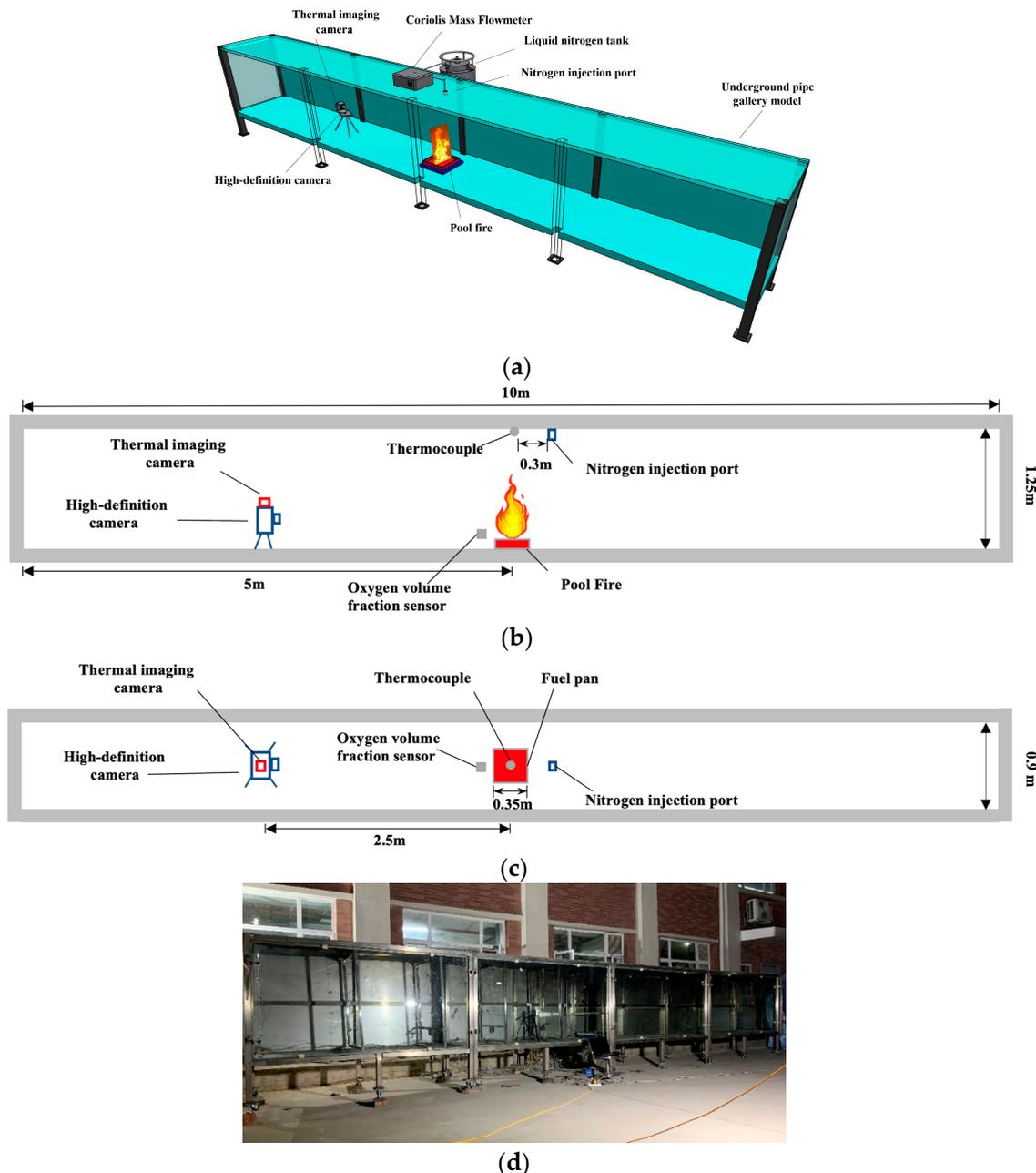
**Figure 1.** The liquid nitrogen fire extinguishing test system for the underground confined space. (a) Overall view; (b) front view; (c) overhead view; (d) photo of the underground pipe gallery model.
