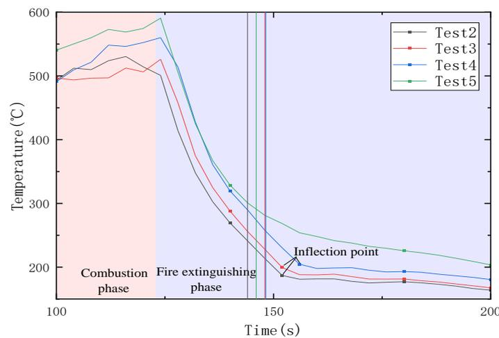
**Figure 5.** Temperature above the fire source under different nitrogen injection flow.
