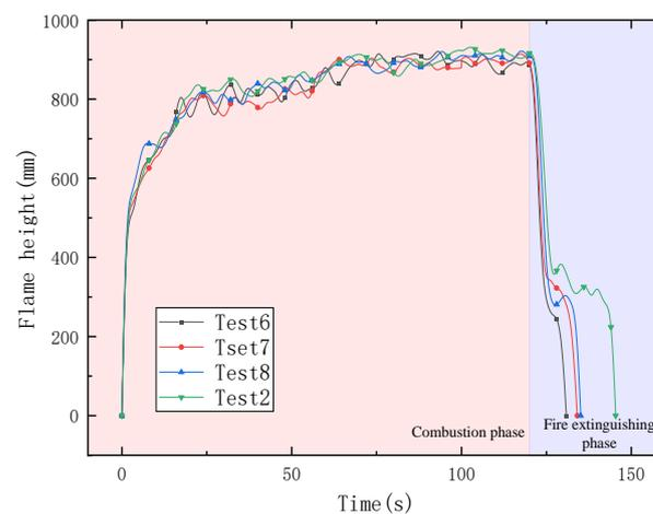
**Figure 7.** Average flame heights at different pipe diameters.
