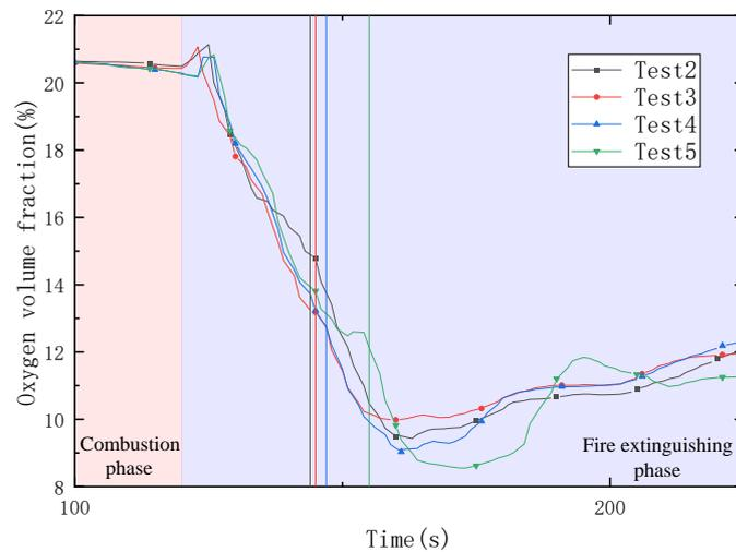
**Figure 6.** Oxygen volume fractions around the fire source under different flow rates.
