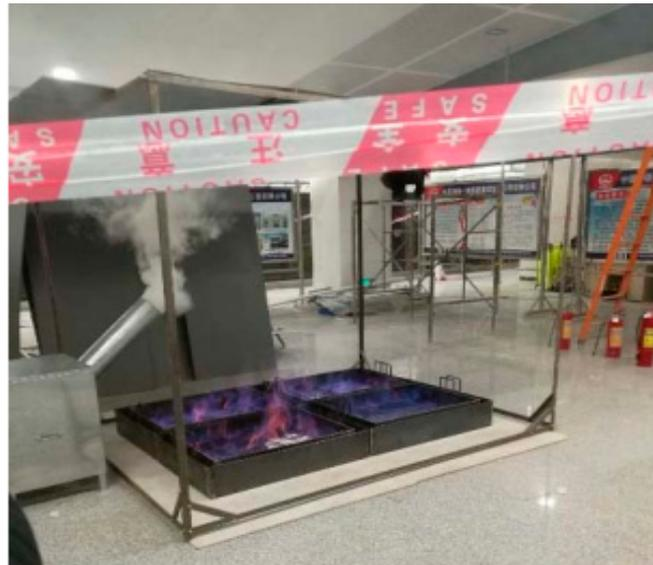
**Figure 11.** Diesel Pan of 1.82 m<sup>2</sup>.
