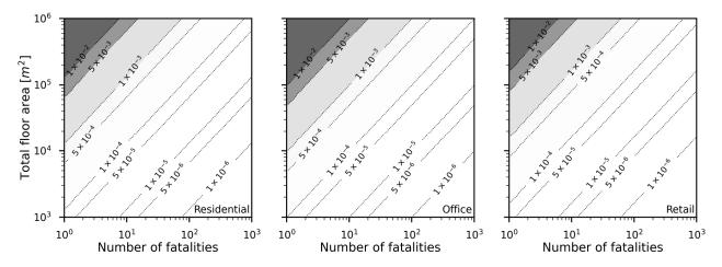
**Figure 5.** Acceptable failure probability in function of the number of fatalities and floor area, for residential, office and retail use.
