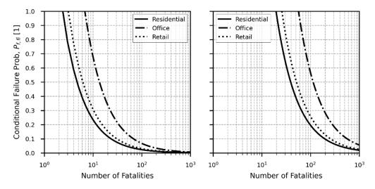
**Figure 6.** Conditional acceptable failure probability in the event of a structurally significant fire in function of the number of fatalities based on the principle of relative (marginal) lifesaving costs (**left**) without sprinklers, (**right**) with sprinklers.
