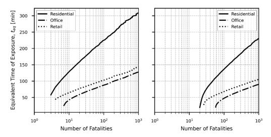
**Figure 7.** Minimum fire resistance in function of the number of fatalities based on the principle of relative (marginal) lifesaving costs (**left**) without sprinklers, (**right**) with sprinklers.
