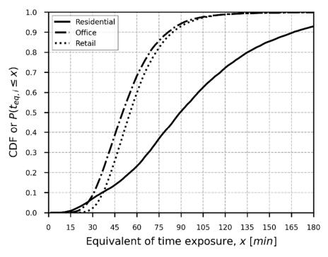
Figure 2. CDF of time equivalence solved from a MCS study using SFEPRAPY.
