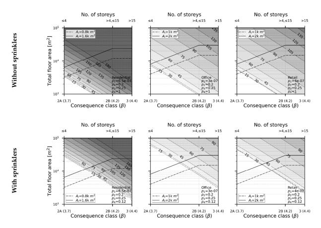
**Figure 3.** Contour plots of the solved structural fire-resistance rating at various building heights and total floor area (without and with sprinklers); A<sub>i</sub> denotes floor area per storey.
