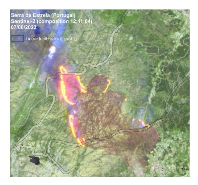
**Figure 4.** Linear fuel breaks (approximately 125 m wide) crossed by a large wildfire that occurred in August 2022 in Serra da Estrela, central Portugal.
