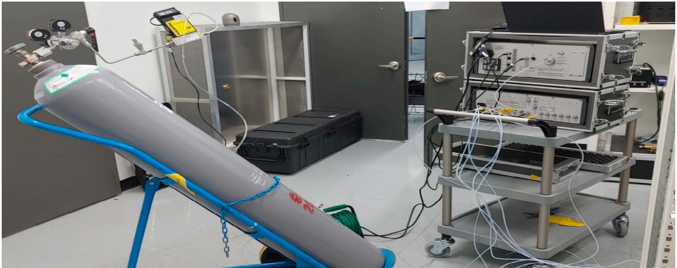
**Figure 2.** Tracer gas (SF<sub>6</sub> 1%, 99% N<sub>2</sub>) and photoacoustic gas monitor.
