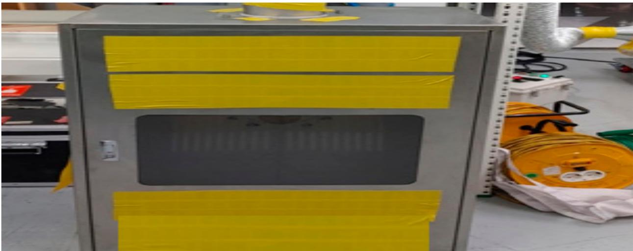
**Figure 5.** Gas box modeling with 0% opening area.
