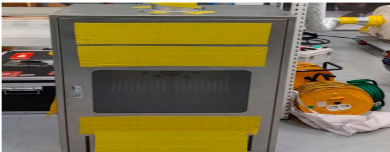
Figure 7. Gas box modeling with 57% opening area (both openings).
