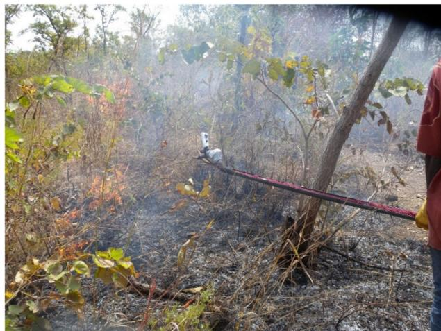
**Figure 7.** Collecting emissions data using a long nozzle on an IMR 1400 gas analyzer from a low-intensity backfire in the village of Tabou (Photograph by P. Laris).
