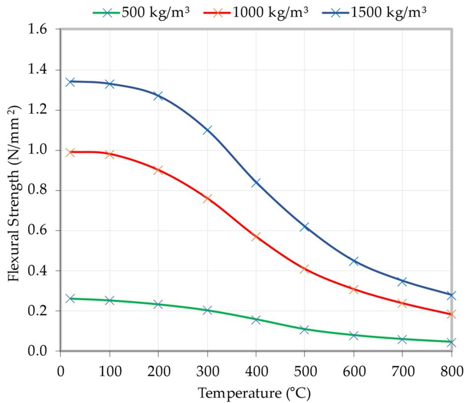
Figure 15. Influence of varying temperatures on the LFC flexural strength.
