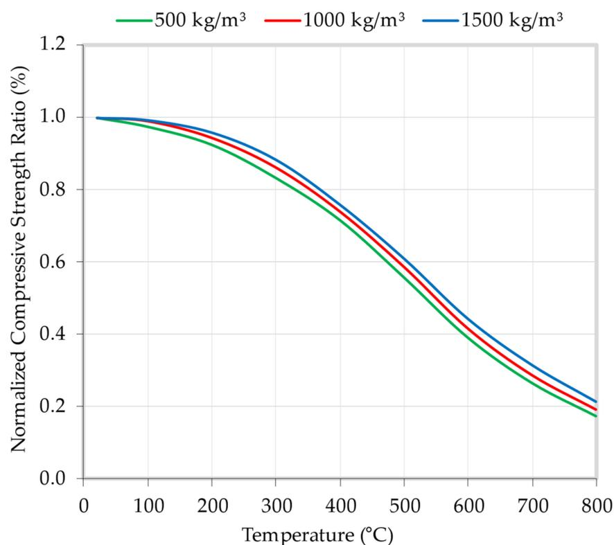
**Figure 9.** Influence of varying temperatures on the normalized LFC compressive strength.
