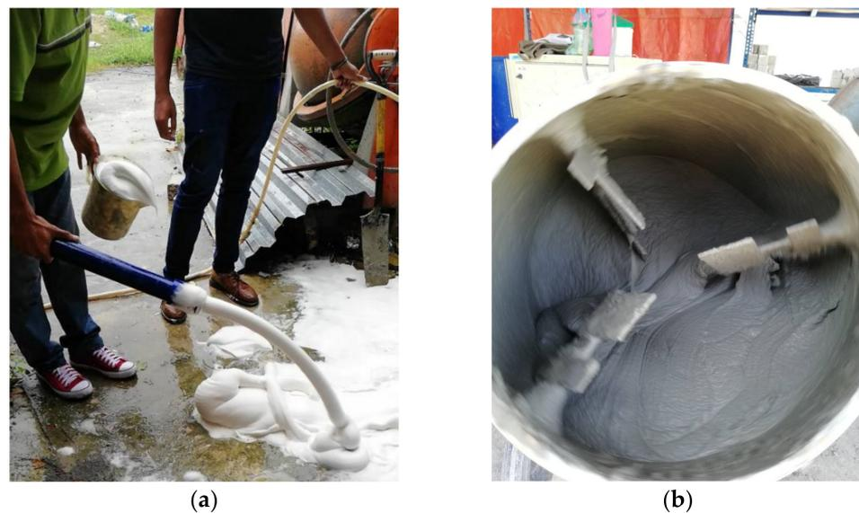
**Figure 1.** Preparation of LFC mixture. (a) stable foam; (b) uniform LFC mix.
