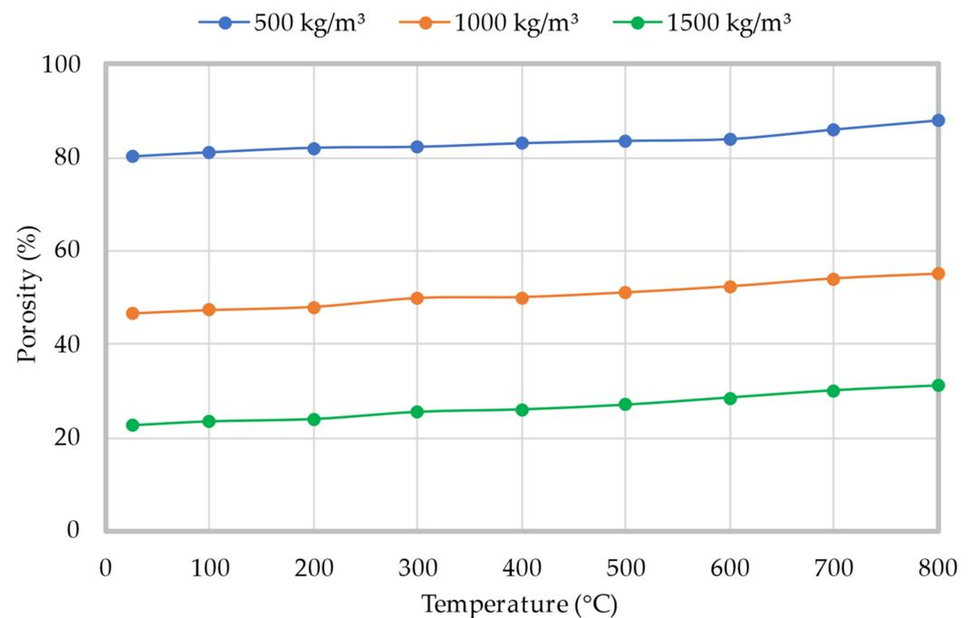
**Figure 6.** Influence of LFC density on its porosity value at varying temperatures.
