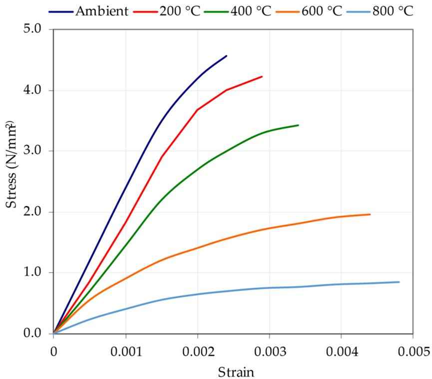
Figure 11. Stress–strain relationship for 1000 kg/m<sup>3</sup> density at varying temperatures.
