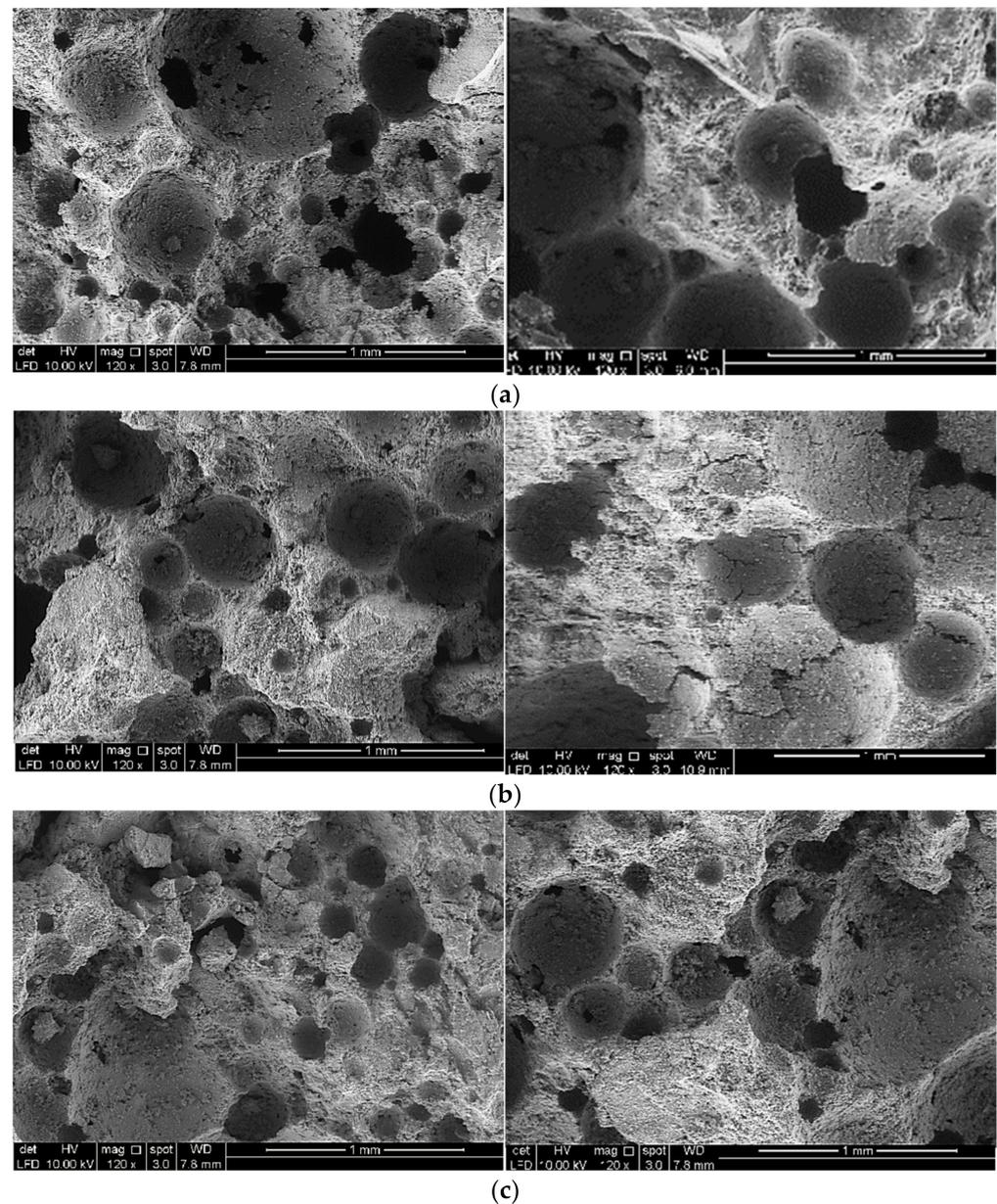
**Figure 7.** Comparison of SEM micrographs of varying densities at ambient temperature and after exposure to 600 °C. (a) 500 kg/m<sup>3</sup> density at 20 °C (left) and at 600 °C (right); (b) 1000 kg/m<sup>3</sup> density at 20 °C (left) and at 600 °C (right); (c) 1500 kg/m<sup>3</sup> density at 20 °C (left) and at 600 °C (right).
