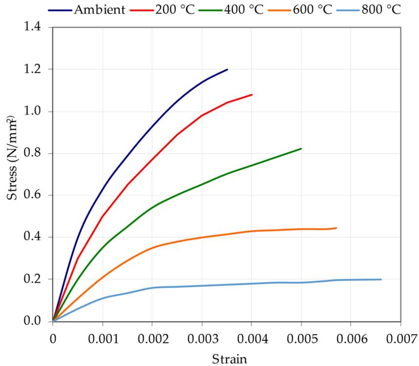
Figure 10. Stress–strain relationship for 500 kg/m<sup>3</sup> density at varying temperatures.
