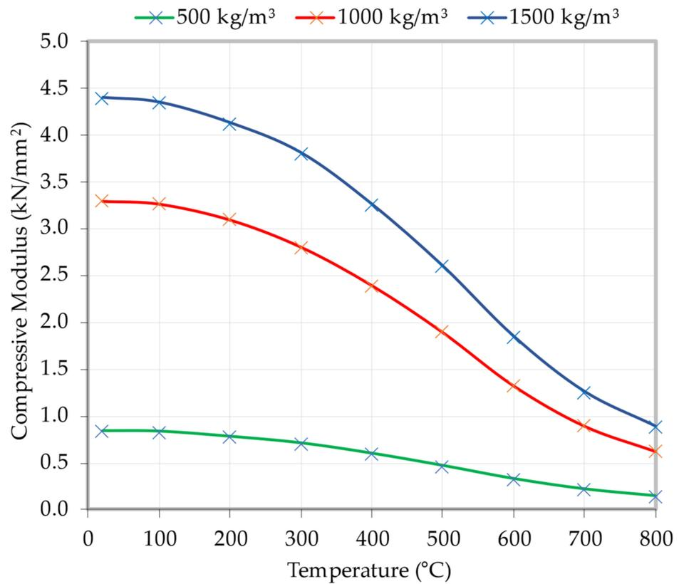
Figure 13. Influence of varying temperatures on the LFC compressive modulus.
