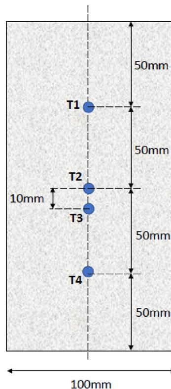
Figure 3. Typical LFC cylinder sample with thermocouples arrangement.
