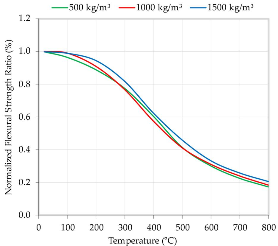
Figure 16. Influence of varying temperatures on the normalized LFC flexural strength.
