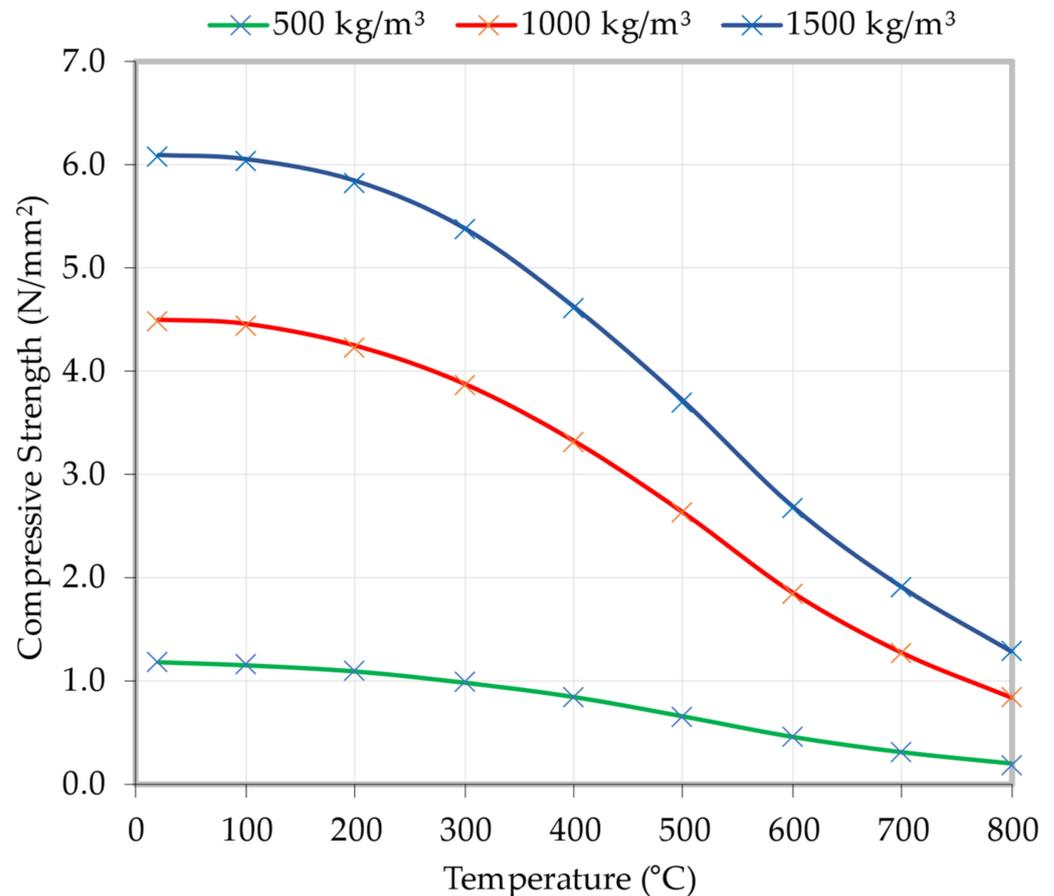
**Figure 8.** Influence of varying temperatures on the LFC compressive strength.
