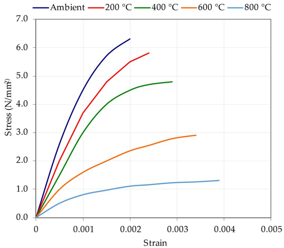
Figure 12. Stress–strain relationship for 1500 kg/m<sup>3</sup> density at varying temperatures.
