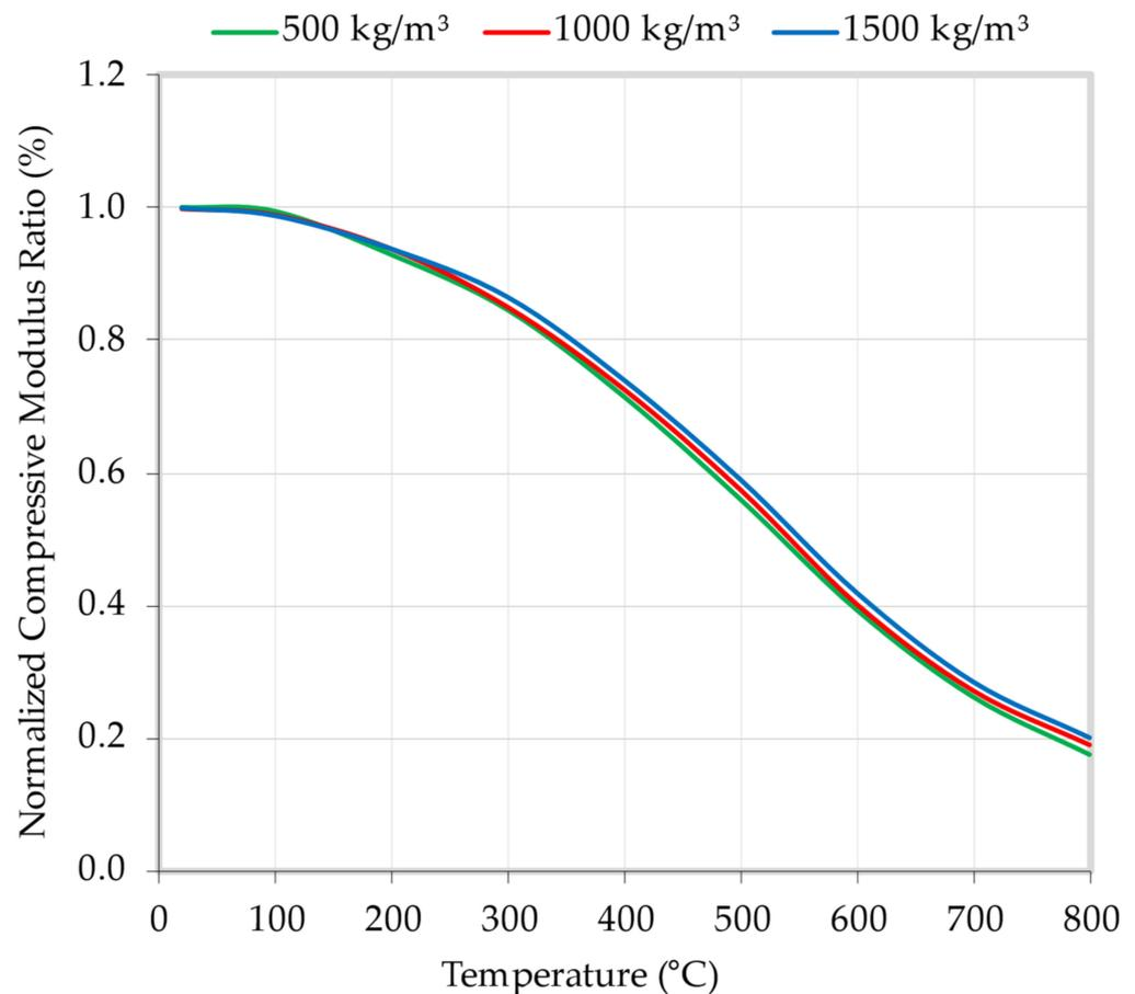
**Figure 14.** Influence of varying temperatures on the normalized LFC compressive modulus.
