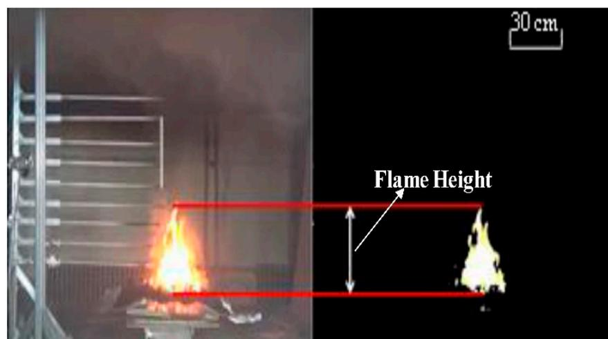
**Figure 5.** Comparison between pictures of flame height before and after processing.
