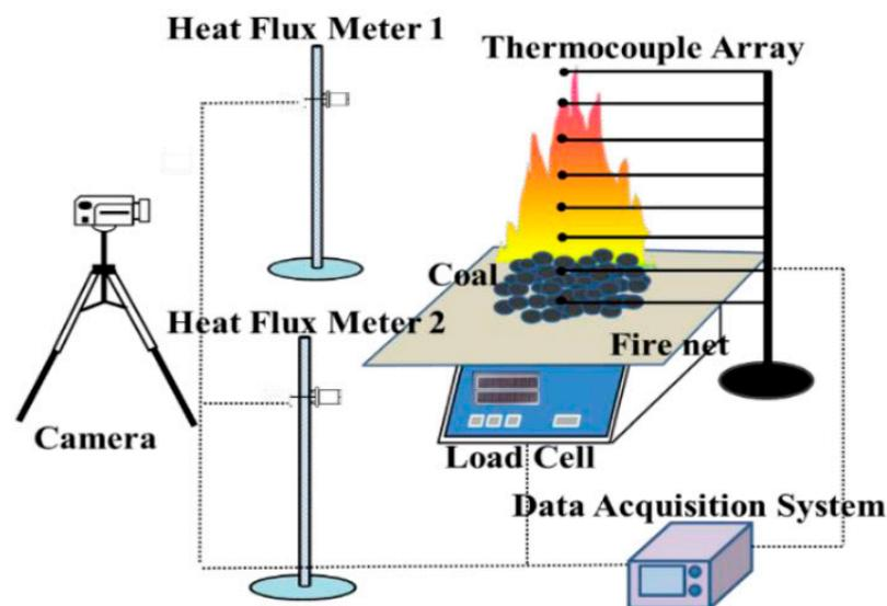
**Figure 1.** The testing apparatus for flame combustion of coal.
