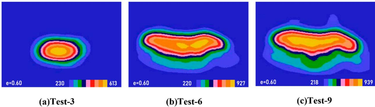
**Figure 10.** The surface temperature changes of Test-3, Test-6, and Test-9 in the smoldering stage (where (a) is a coal pile of 40 cm diameter and 6 cm thickness, (b) is a coal pile of 60 cm diameter and 6 cm thickness, (c) is a coal pile of 80 cm diameter and 6 cm thickness).
