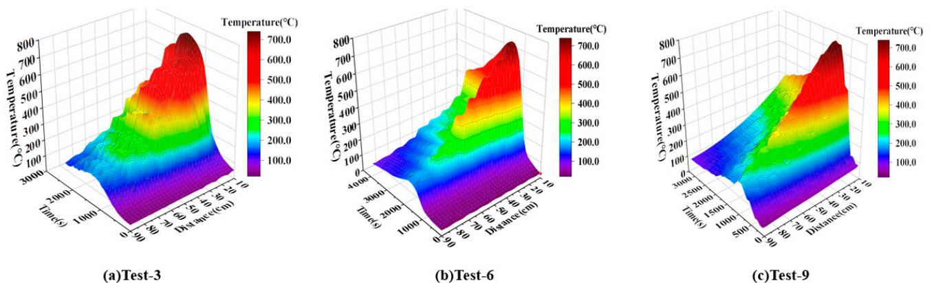
Figure 9. The flame temperature changes of Test-3, Test-6, and Test-9 (where (a) is a coal pile of 40 cm diameter and 6 cm thickness, (b) is a coal pile of 60 cm diameter and 6 cm thickness, (c) is a coal pile of 80 cm diameter and 6 cm thickness).
