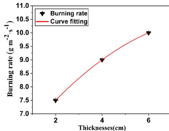
**Figure 4.** The burning rate fitting curve with different thicknesses.
