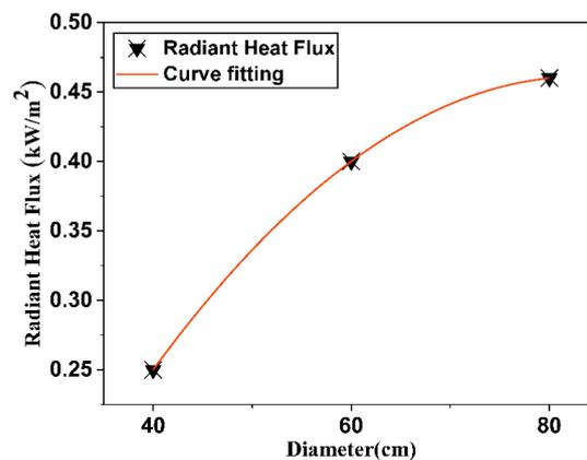
**Figure 13.** The radiant heat flux fitting curve with different diameters.
