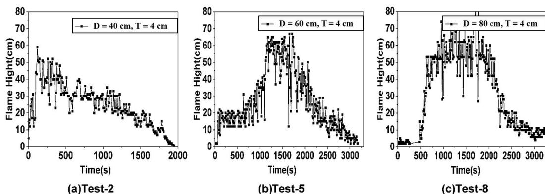
**Figure 7.** The flame height changes from Test-2, Test-5, and Test-8 (where (a) is a coal pile of 40 cm diameter and 4 cm thickness, (b) is a coal pile of 60 cm diameter and 4 cm thickness, (c) is a coal pile of 80 cm diameter and 4 cm thickness).
