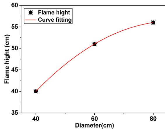
Figure 8. The flame height fitting curve with different diameters.
