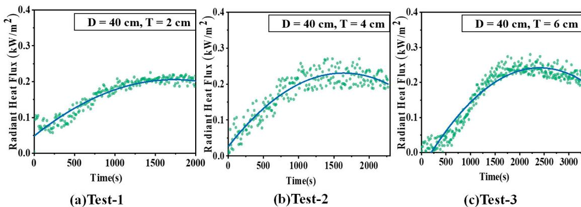
**Figure 11.** The radiant heat flux changes from Test-1 to Test-3 (where (a) is a coal pile of 40 cm diameter and 2 cm thickness, (b) is a coal pile of 40 cm diameter and 4 cm thickness, (c) is a coal pile of 40 cm diameter and 6 cm thickness).
