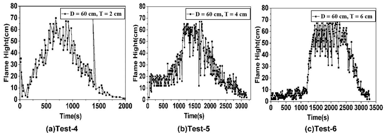
**Figure 6.** The flame height changes from Test-4 to Test-6 (where (a) is a coal pile of 60 cm diameter and 2 cm thickness, (b) is a coal pile of 60 cm diameter and 4 cm thickness, (c) is a coal pile of 60 cm diameter and 6 cm thickness).
