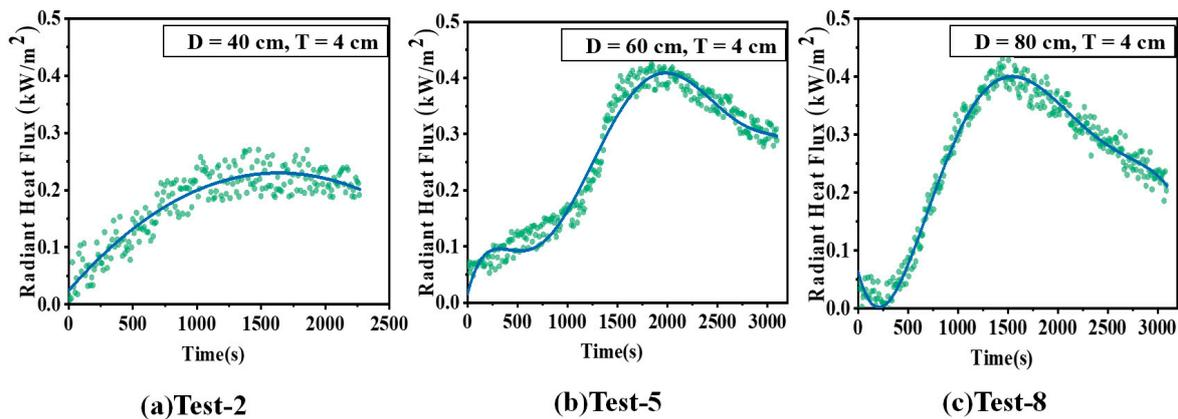
**Figure 12.** The radiant heat flux changes of Test-2, Test-5, and Test-8 (where (a) is a coal pile of 40 cm diameter and 4 cm thickness, (b) is a coal pile of 60 cm diameter and 4 cm thickness, (c) is a coal pile of 80 cm diameter and 4 cm thickness).
