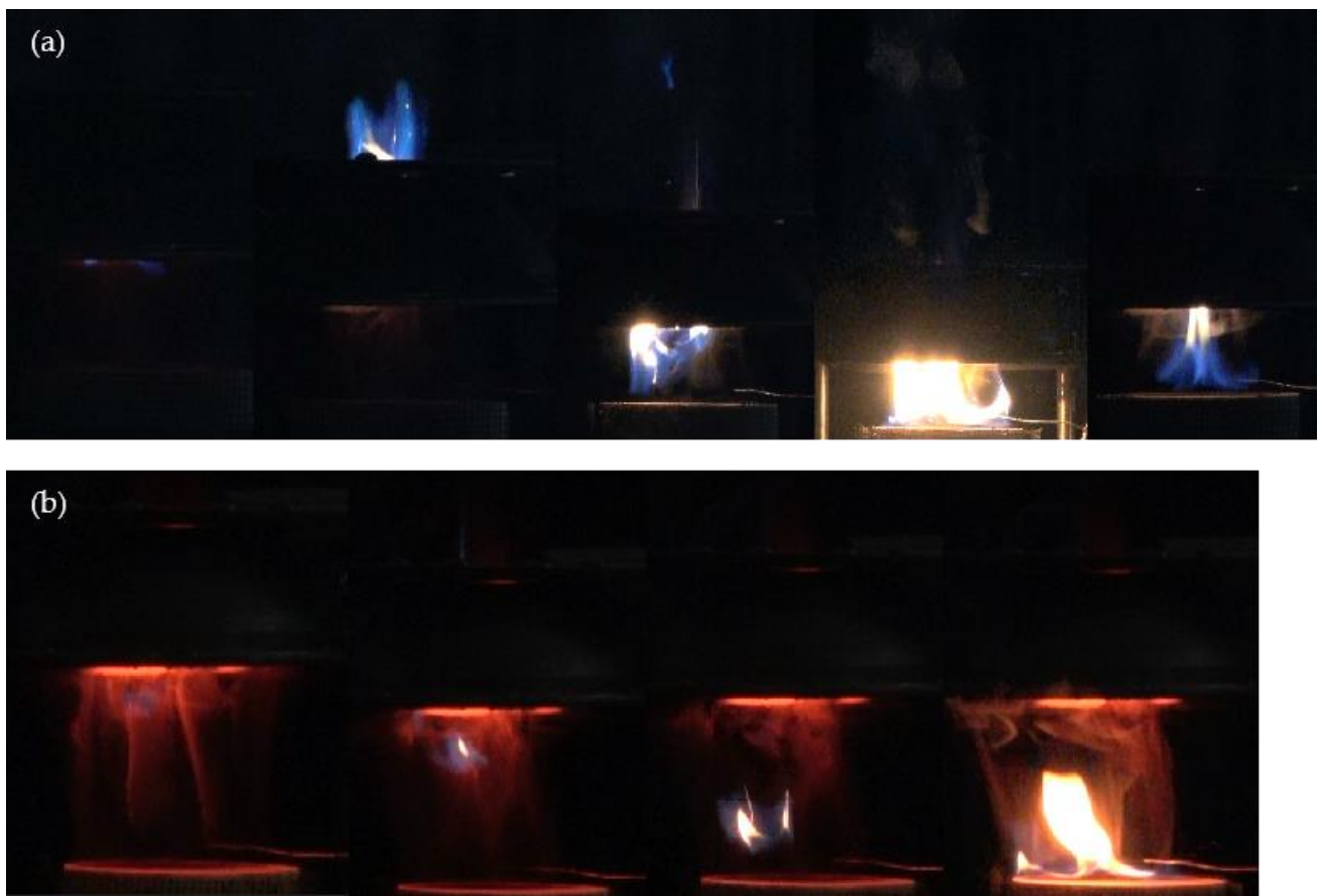
Figure 6. Timelapse images of ignition phenomena of pine wood: (a) D = 45 mm; (b) D = 80 mm.
