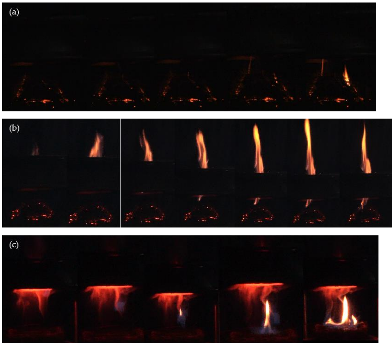
Figure 4. Timelapse images of ignition phenomena of pine needle: (a) D = 45 mm; (b) D = 50 mm; (c) D = 60 mm.
