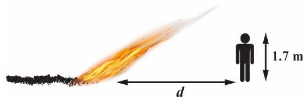
**Figure 3.** Configuration of the "human body" target with respect to the flame front position.
