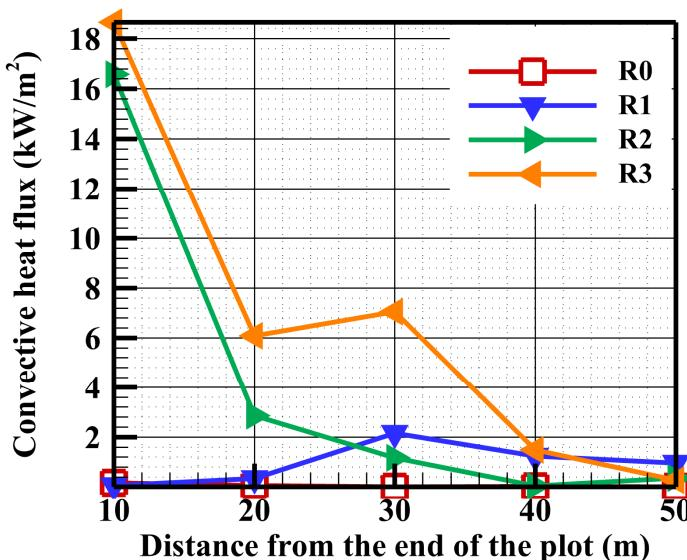
**Figure 11.** Variation of the convective heat fluxes received by each level with respect to the distance separating the building from the fire front.
