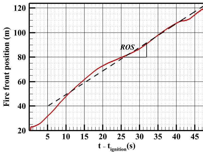
**Figure 6.** Variation with time of the furthermost point of the pyrolysis front at the fuel bed surface obtained by FireStar2D after ignition time.
