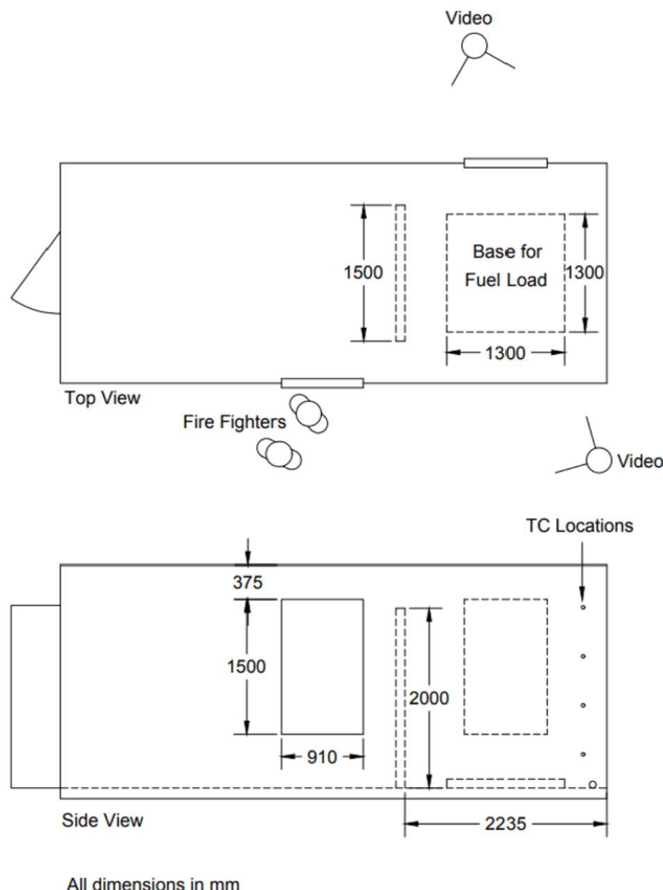
**Figure 1.** Floor plan and instrumentation.
