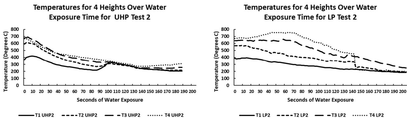
**Figure 3.** Temperature, in degrees Celsius over water exposure time, for each of the four thermocouples during a representative test for each of UHP and LP conditions. T1 represents the lowest thermocouple, while T4 represents the highest thermocouple in the array.
