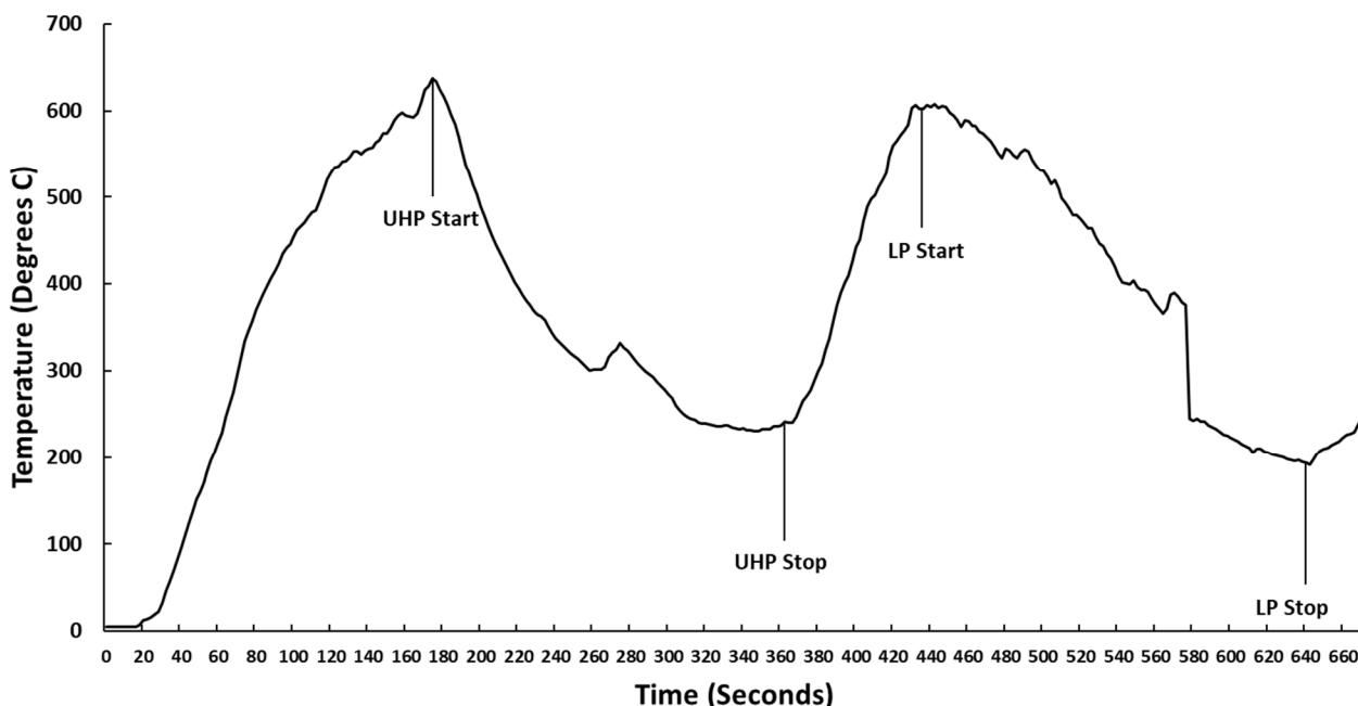
**Figure 4.** Median thermocouple array temperature over time with the start and stop of water flow for each of UHP trial 2 and LP trial 2 indicated.
