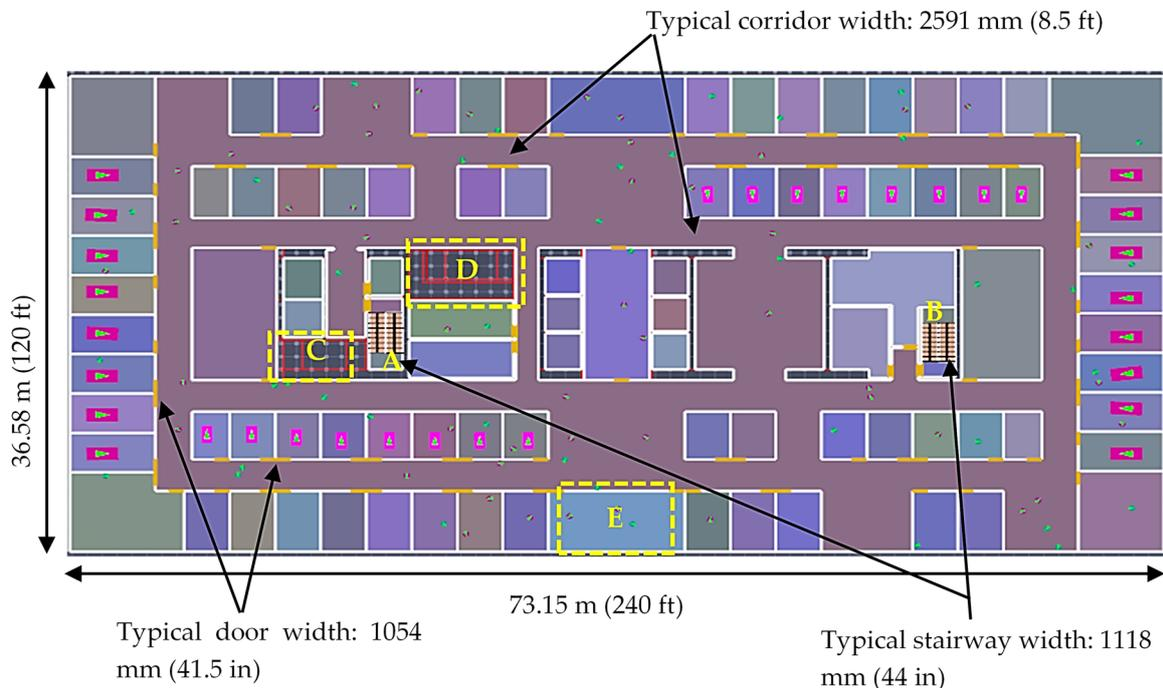
**Figure 3.** Dimensions of egress components as per IBC 2018 [4] and NFPA 101 [5].
