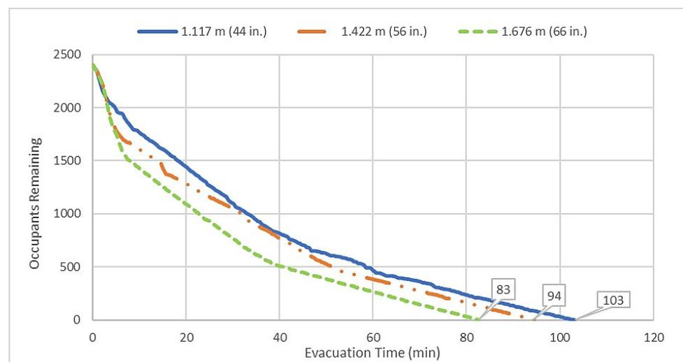
**Figure 7.** Evacuation time with different staircase widths.
