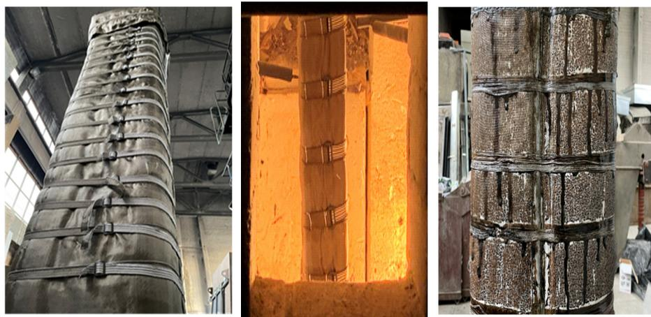
**Figure 9.** Specimen no. 5 before starting the test (**left**), during the test (**centre**) and after the test (**right**).
