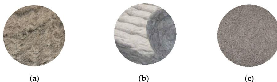
**Figure 2.** Basalt fibres: (a) basalt superfine fibres with fibre diameter 1–3 µm; (b) basalt ultrafine fibres with fibre diameter 0.6–1 µm; (c) basalt microfine fibres with fibre diameter less than 0.6 µm [48].
