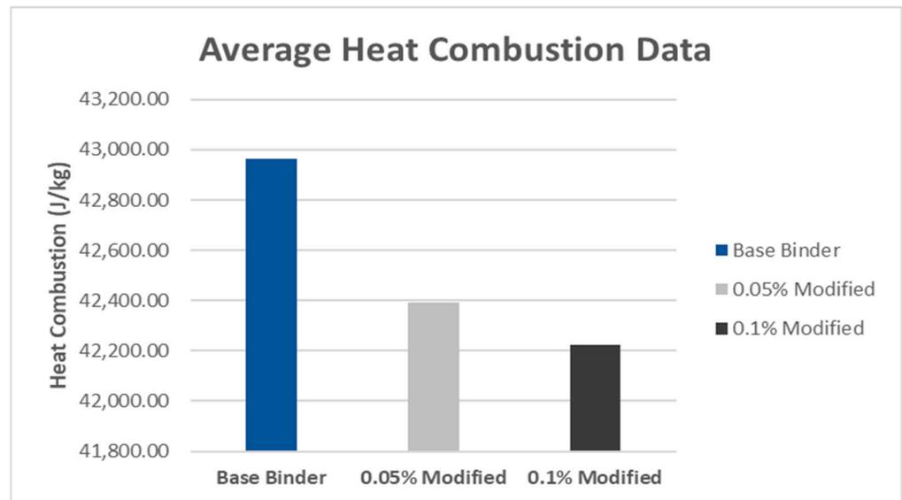
**Figure 6.** Average heat combustion results of base binders and Zychotherm-modified binders (reproduced).
