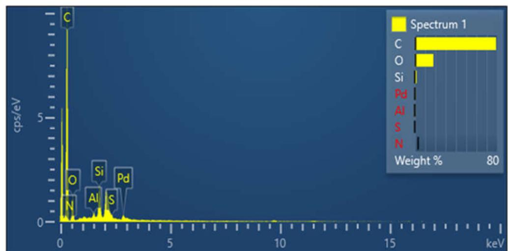
**Figure 9.** EDX spectrum of 0.1% Zychotherm-modified asphalt binder.
