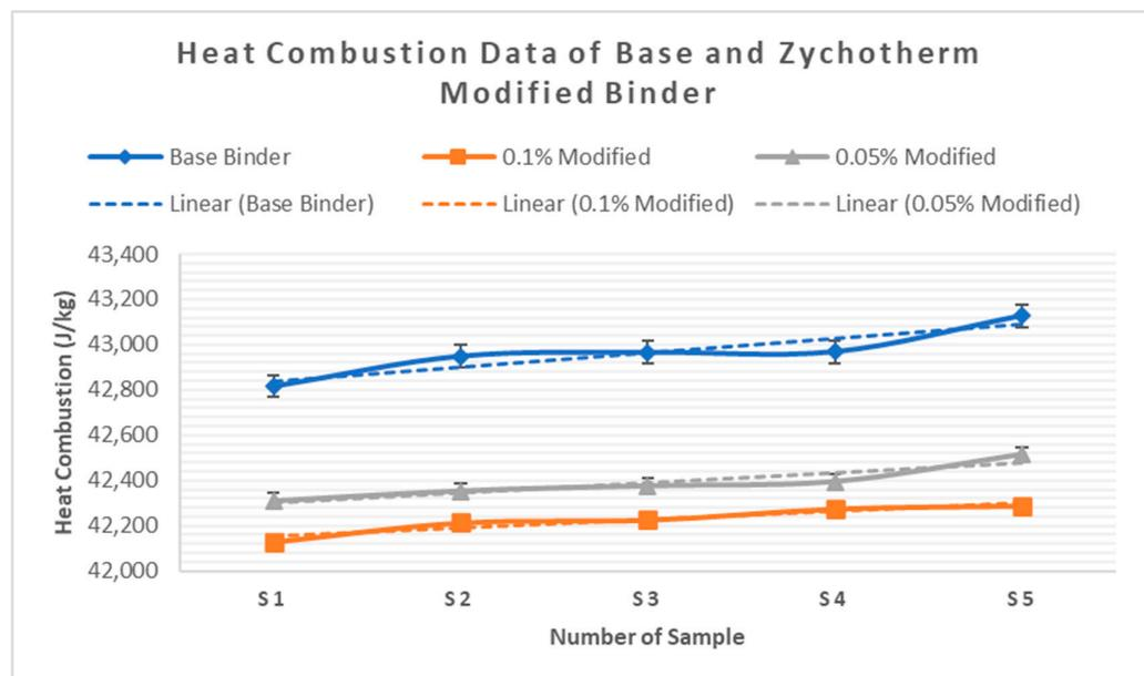
Figure 5. Heat combustion result of base binder and Zychotherm-modified binder (five repetitions for each sample) (reproduced).
