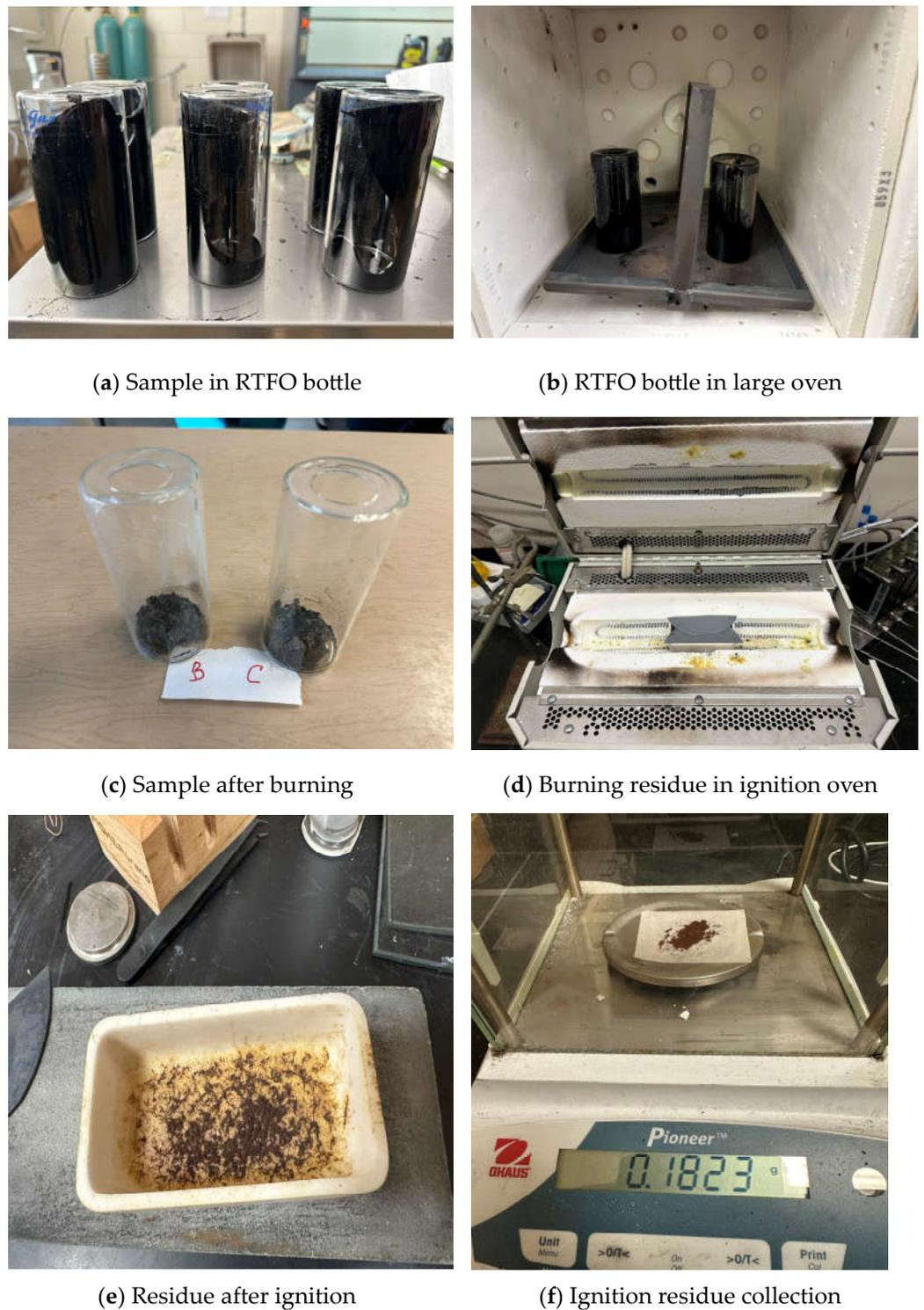
**Figure 3.** Burning and ignition of a large sample: (a) Weighed sample in RTFO bottle; (b) RTFO bottle placed in large oven for burning; (c) samples after burning; (d) burned sample placed in small oven for ignition; (e) residue after ignition; (f) ignition residue.
