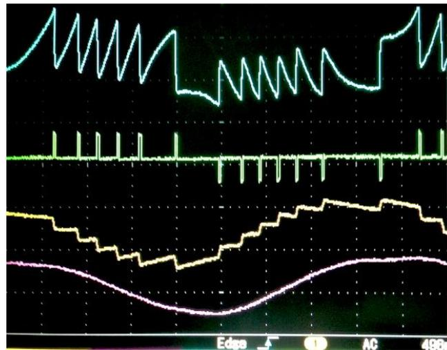
**Figure 13.** Waveforms obtained using SC processing. Traces from top to bottom: the SMI signal; the differentiated pulses; the switching removed; and the final reconstructed (low pass filtered) signal (from Ref. [40], ©SPIE; reprinted with permission).
