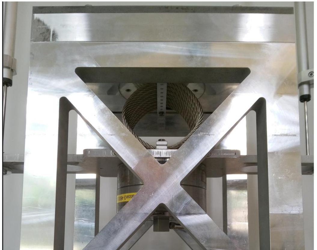
Figure 19. Picture of wire rope shockmount in tension configuration.
