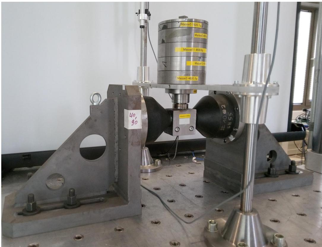
Figure 21. Picture of elastomer shockmounts in shear configuration.
