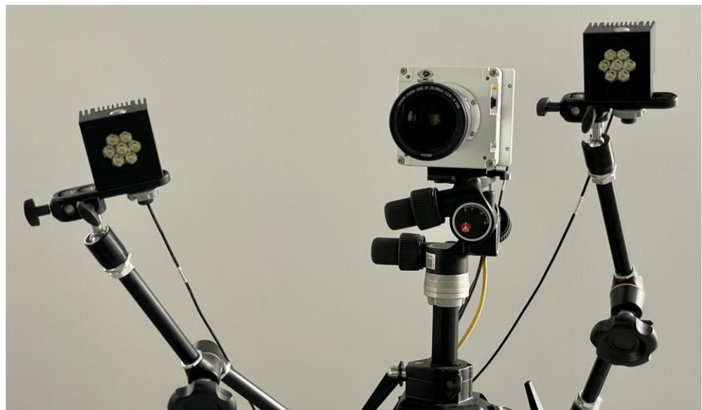
Figure 26. Highspeed camera with LED spots.
