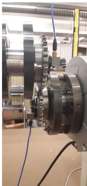
**Figure 9.** Triaxial accelerometers applied on the gears.
