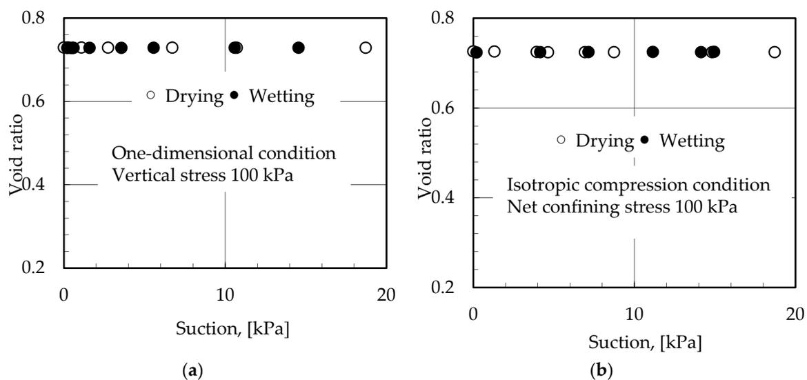
**Figure 7.** Relationship between suction and void ratio (a) Suction vs. void ratio in one dimensional stress condition; (b) Suction vs. void ratio in isotropic stress condition.
