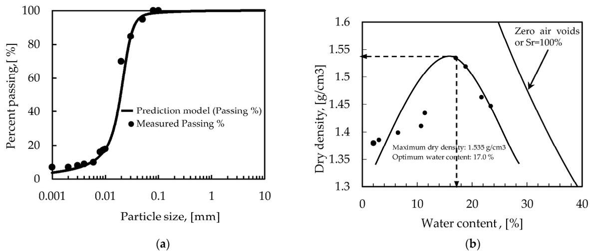
**Figure 1.** Grain size Distribution and compaction curve of silt (a) Grain size distribution for silt soil; (b) Compaction curve for silt soil.
