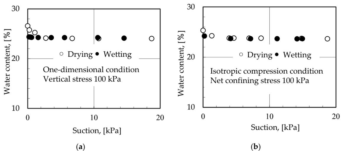
**Figure 5.** Relationship between suction and water content (a) Suction vs. water content in one dimensional stress condition; (b) Suction vs. water content in isotropic stress condition.
