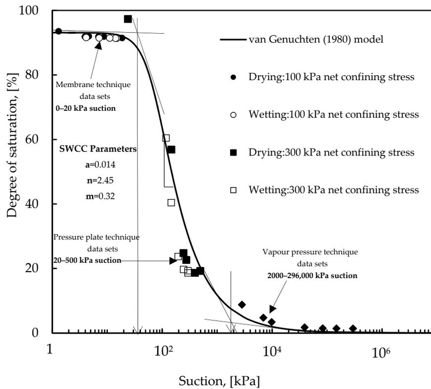
**Figure 11.** Curve fitting of soil–water characteristic curve data sets with different stress conditions.
