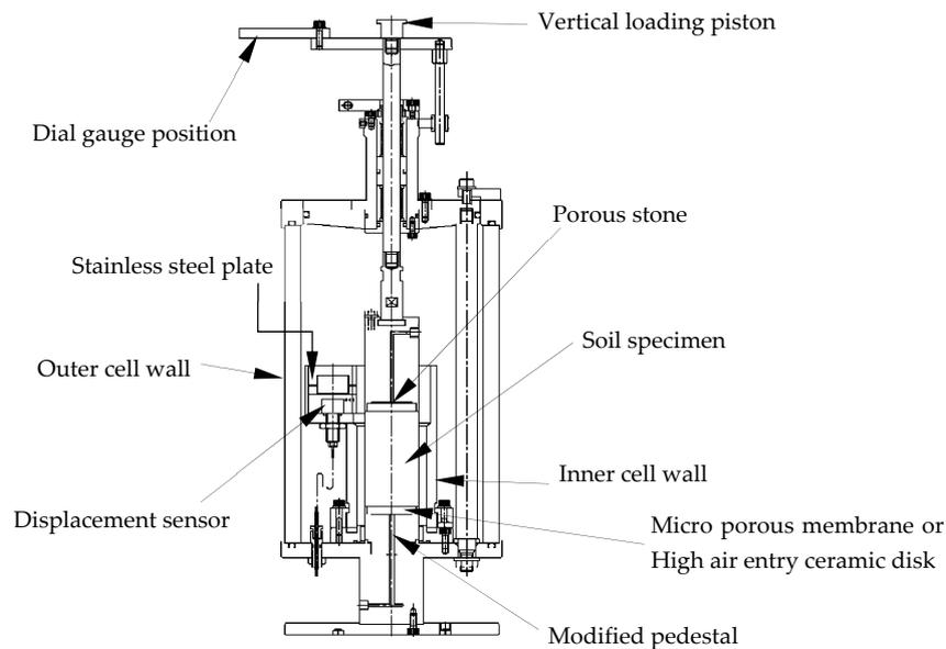
**Figure 3.** Schematic diagram of modified triaxial apparatus for isotropic stress condition.
