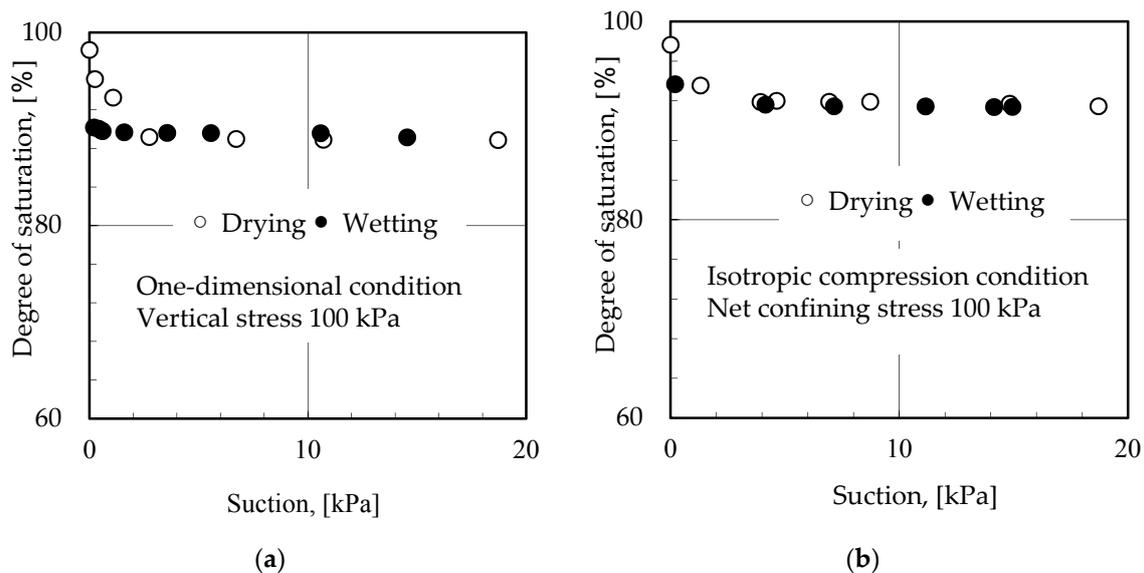
**Figure 6.** Relationship between suction and degree of saturation (a) Suction vs. degree of saturation in one dimensional stress condition; (b) Suction vs. degree of saturation in isotropic stress condition.
