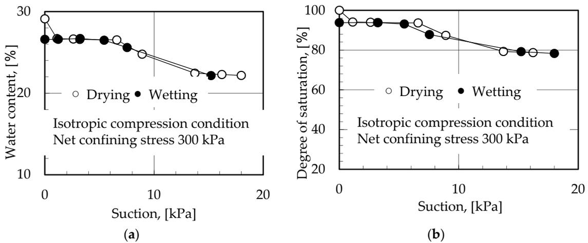
**Figure 8.** Soil–water characteristic curves at 300 kPa net confining stress (a) Suction vs. water content at 300 kPa net confining stress; (b) Suction vs. degree of saturation at 300 kPa net confining stress.
