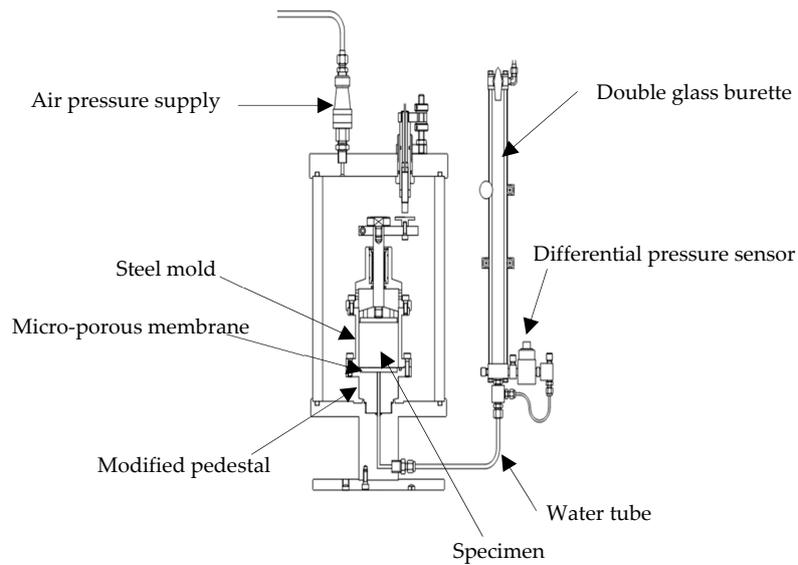
**Figure 2.** Schematic diagram of modified Soil Water Characteristic Curve apparatus for one-dimensional stress condition.
