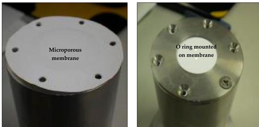
**Figure 4.** Illustration of Supor 450 saturated microporous membrane on porous stone.
