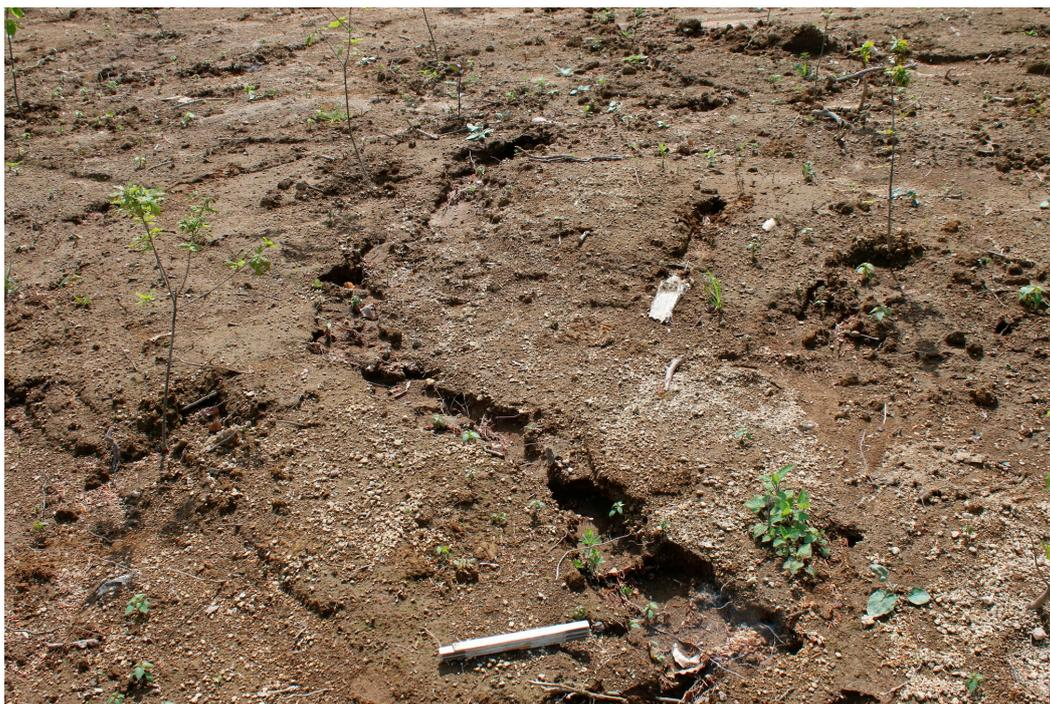
**Figure 17.** Example for an erosion rill on backfilled sub-area CUT, folding ruler for scale.
