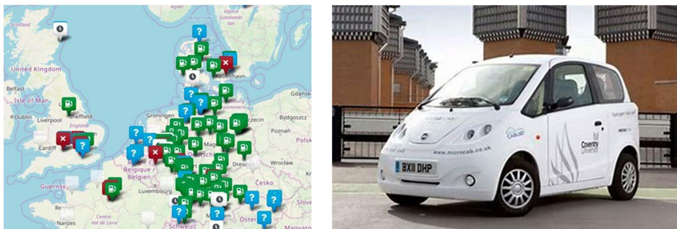
**Figure 6.** Left: 2021 hydrogen stations in the UK compared to the EU, showing that the UK has only 12 stations in 2021 with only 4 working, which is well behind Germany with 93; Right: Microcab HFCBEV taxi/van built in Birmingham.
