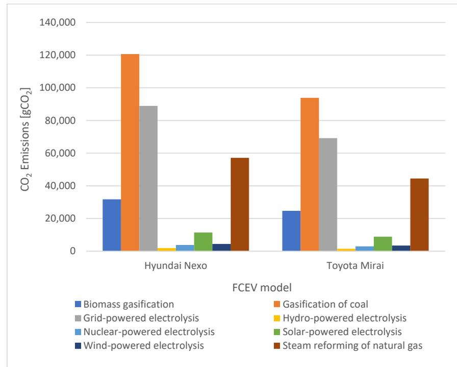
Figure 8. CO<sub>2</sub> emissions for FCEVs considering the driving range.
