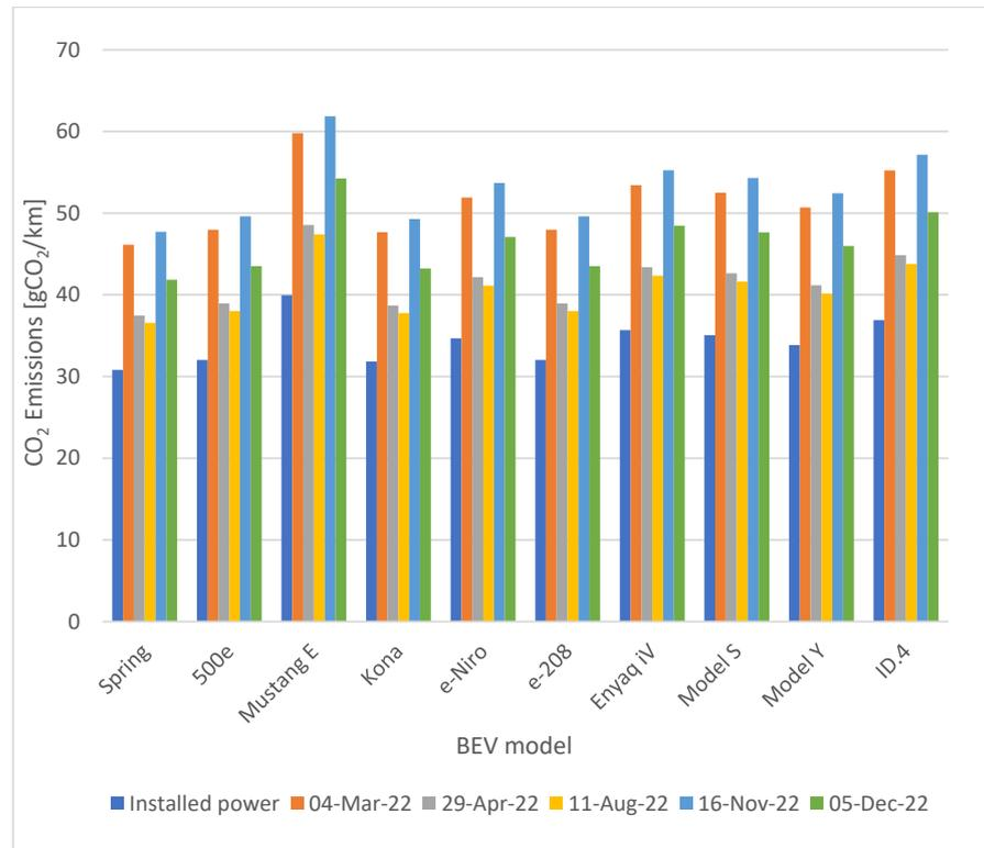
Figure 3. CO<sub>2</sub> emissions for BEVs considering fuel consumption.
