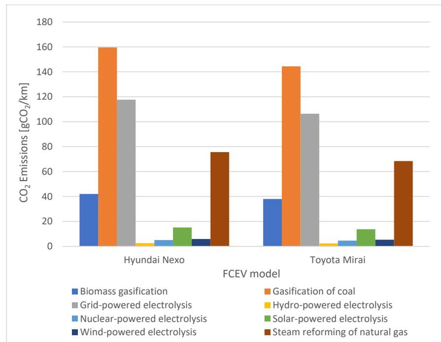
Figure 6. CO<sub>2</sub> emissions for FCEVs considering fuel consumption.
