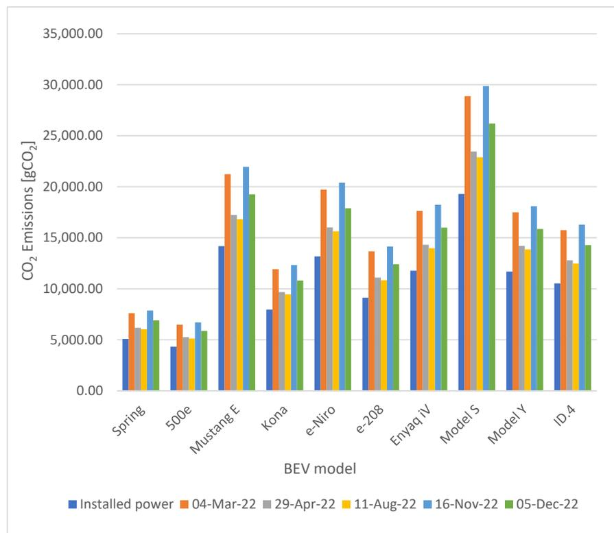
Figure 5. CO<sub>2</sub> emissions for BEVs considering the driving range.
