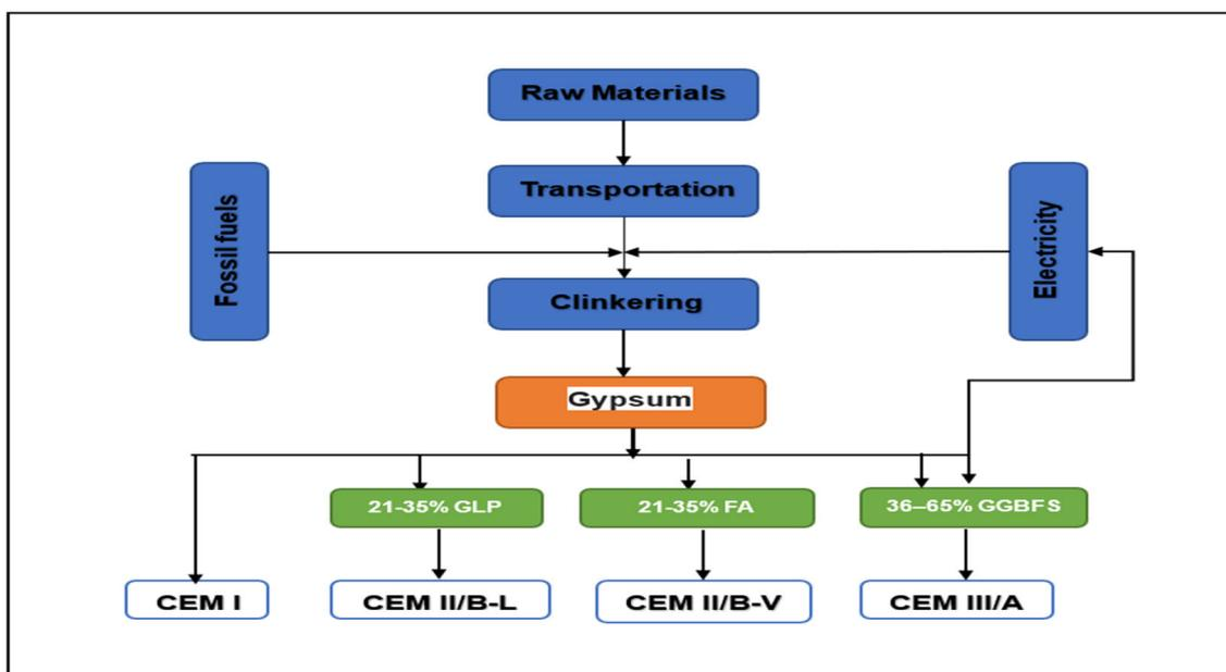
**Figure 1.** System boundary of cement production.
