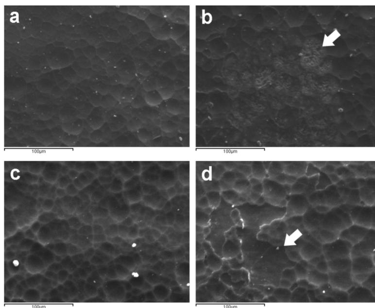
**Figure 5.** SEM images of PP: (a) control, (b) non-soiled sample, treated with chelate MGDA solution showing MGDA residues presence (indicated by the arrow), (c) carbon soiled sample after cleaning with ethyl lactate and (d) carbon soiled sample after cleaning with Plurafac<sup>®</sup>, showing deformations on the surface (indicated by the arrow).
