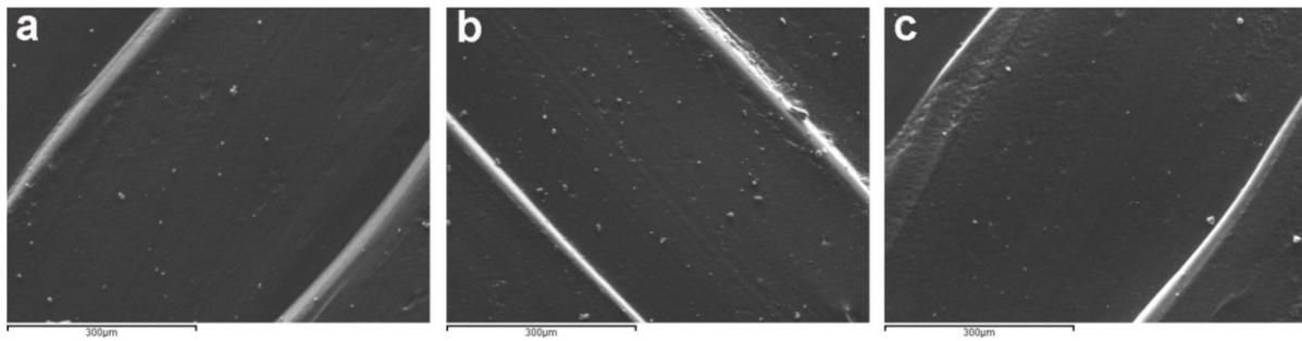
**Figure 6.** SEM images of PLA (a) control, (b) carbon soiled sample cleaned with Plurafac<sup>®</sup> solution, where no soil residues are evidenced, and after water clearance and wiping with dry Evolon<sup>®</sup> CR, which left no cleaning residues either and (c) carbon soiled sample cleaned with limonene with very good cleaning result.
