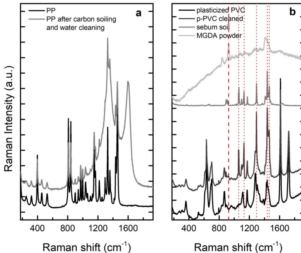
**Figure 2.** Raman spectra of (a) Polypropylene control and water cleaned sample, where the remaining carbon soil residues were evident (broad peaks at  $\sim 1340\text{ cm}^{-1}$  and  $\sim 1590\text{ cm}^{-1}$ ) and (b) Plasticized PVC control and sebum soiled sample after cleaning with chelate MGDA, where residues of the agent and the soil were evident. The peaks attributed to the surface residues of the soil and of the cleaning agent are indicated with dotted and dashed lines respectively.
