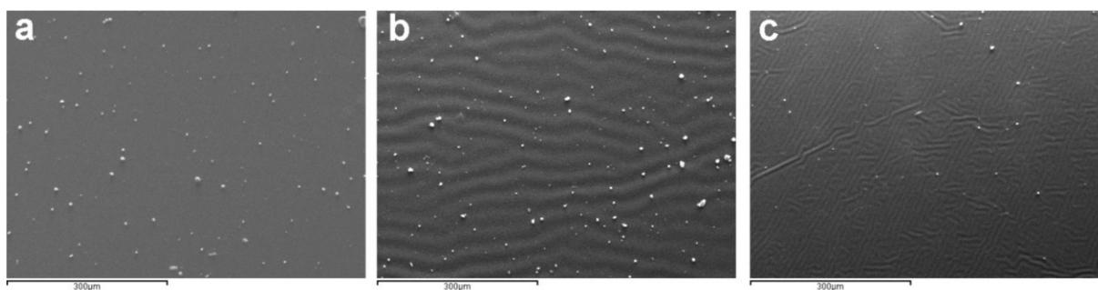
**Figure 3.** SEM images of plasticized PVC: (a) control sample, (b) observed wrinkled pattern in the control sample and (c) non-soiled sample treated with limonene.
