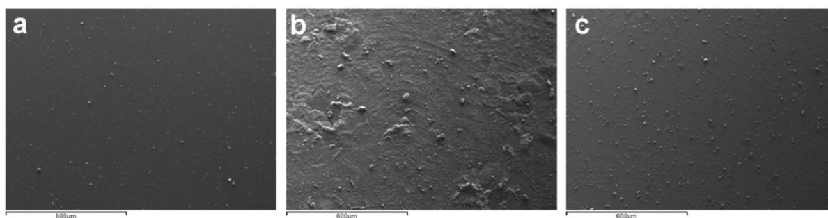
**Figure 7.** SEM images of PMMA: (a) control (non-soiled), (b) sebum soiled sample cleaned with agar gel film and (c) sebum soiled sample cleaned with limonene.
