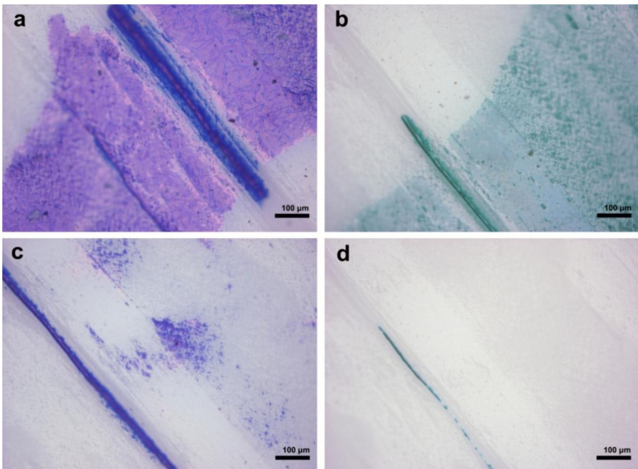
**Figure 9.** Optical Microscopy images of PLA (a,b) before and (c,d) after blue and green ink removal with Plurafac<sup>®</sup> solution.
