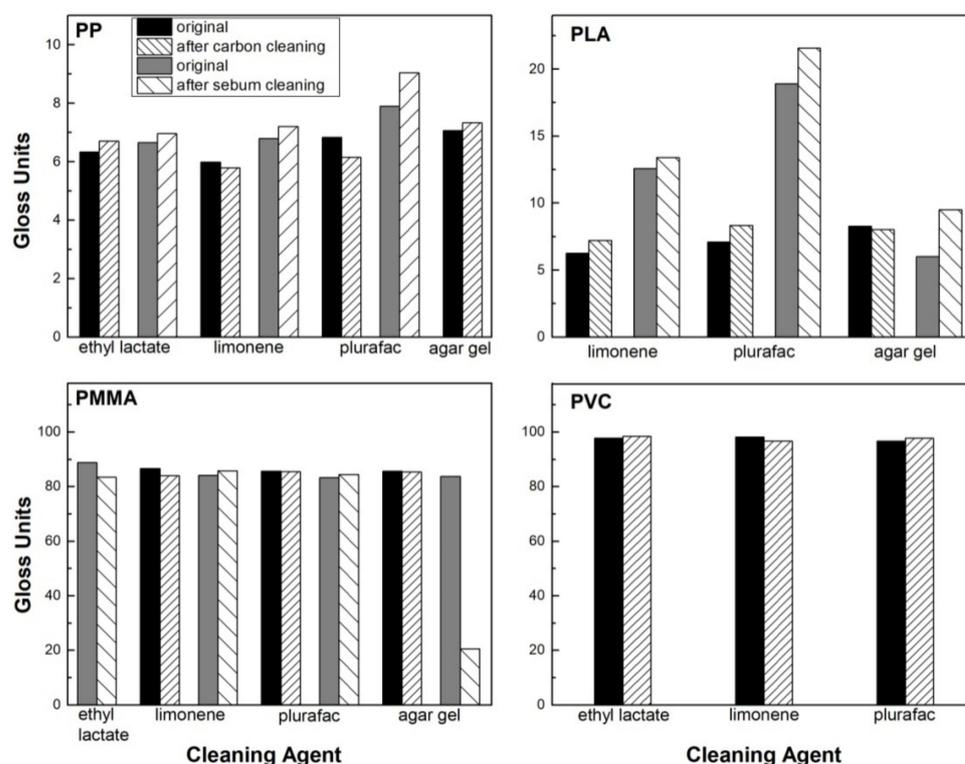
**Figure 8.** Gloss values of untreated PP, PLA, PMMA and PVC surfaces and after soil removal using biodegradable cleaning agents.
