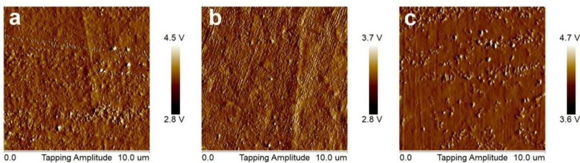
**Figure 4.** AFM tapping amplitude images of plasticized PVC: (a) control, (b) non-soiled sample treated with water and (c) non-soiled sample treated with limonene.
