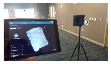
Figure 4. Test field surveying by the Matterport Pro camera.
