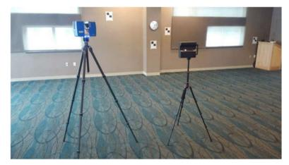
Figure 2. Test field scanning by FARO Scanner.
