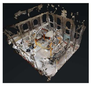
Figure 33. The whole data set obtained by Matterport Pro with places of the camera set up.
