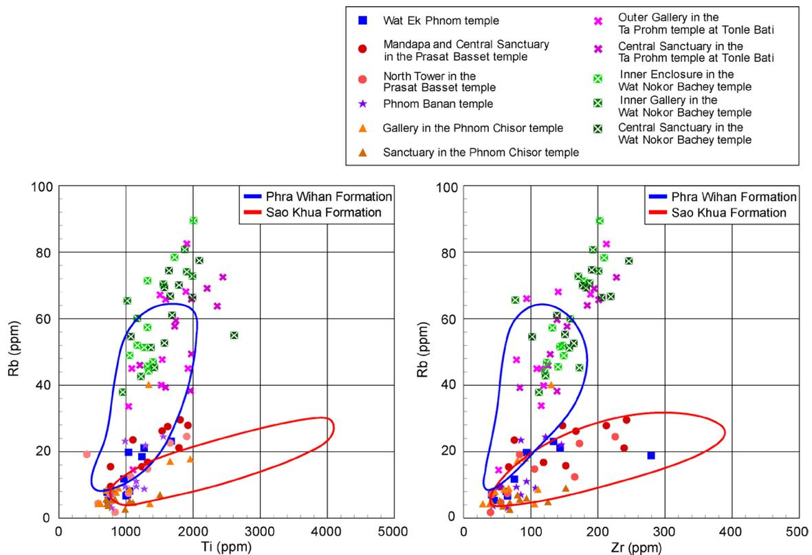
**Figure 8.** Relationships between minor element (Rb, Ti, and Zr) contents in pale brown siliceous sandstones used in the investigated temples.
