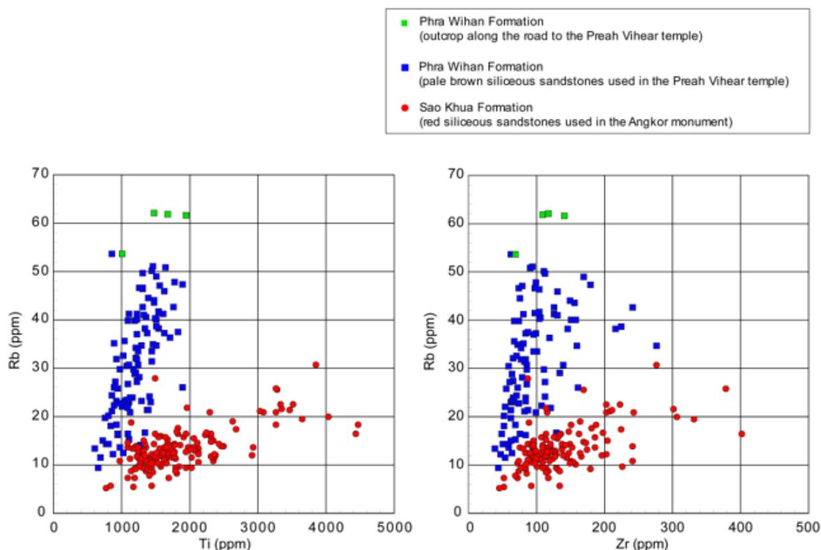
**Figure 6.** Relationships between minor element (Rb, Ti, and Zr) contents in sandstones from the Phra Wihan [6] and Sao Khua [5] formations, determined using pXRF.
