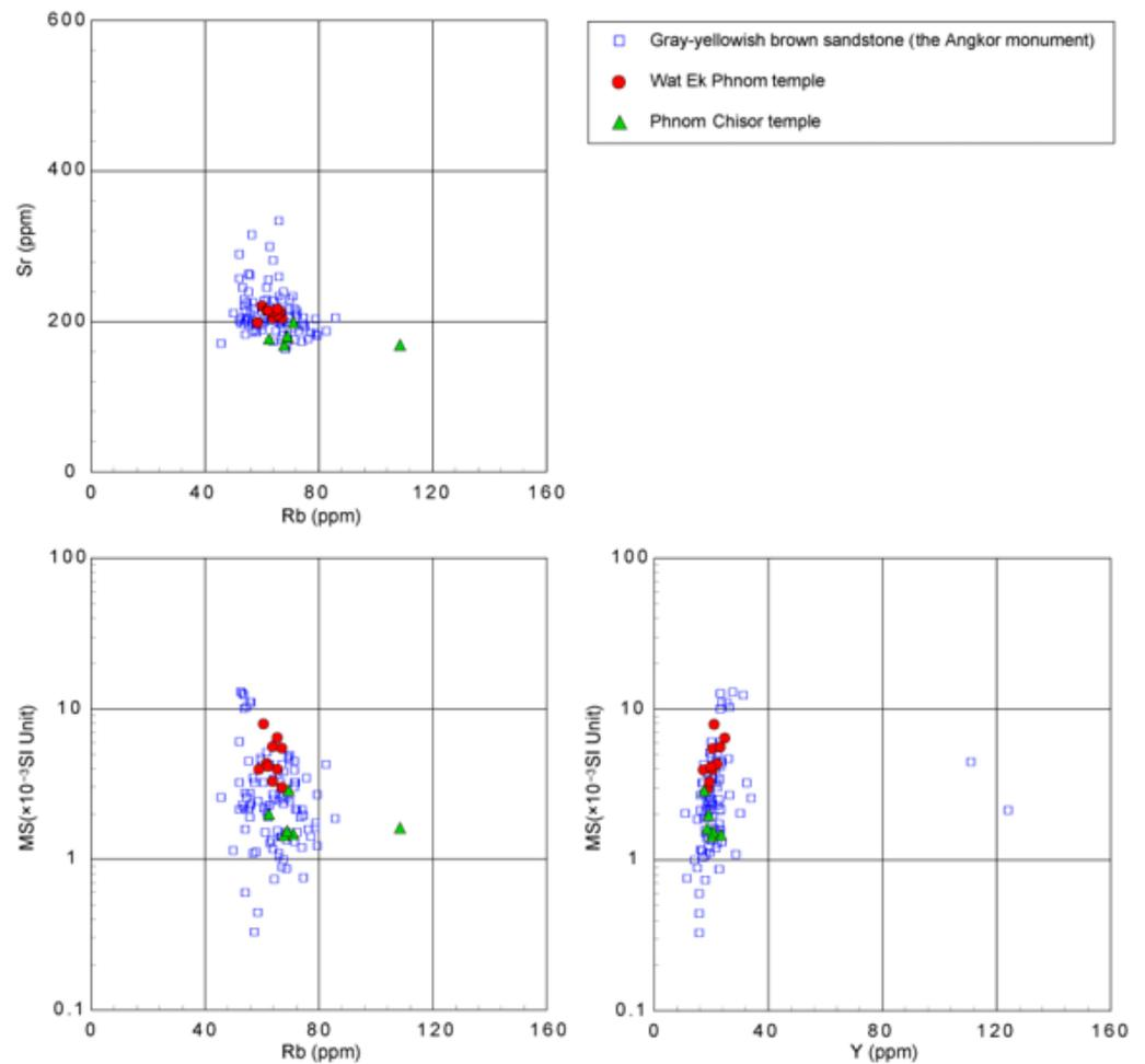
Figure 10. Relationships between magnetic susceptibility and minor element (Sr, Rb, and Y) contents in gray sandstones used in the investigated temples and the Angkor monument.
