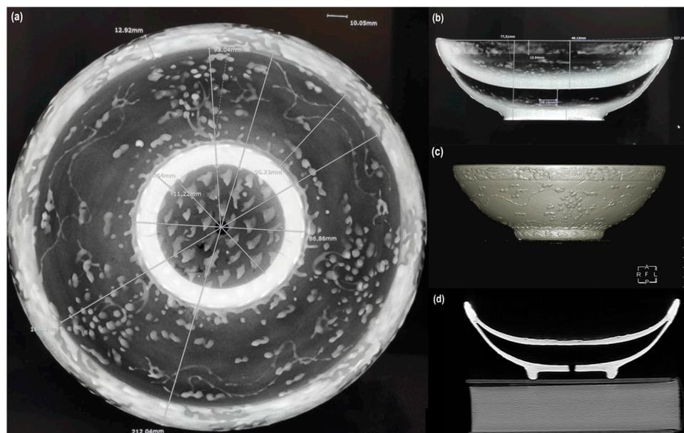
**Figure 2.** Warming bowl ceramic: (a–c) X-ray images: frontal and horizontal views; (d) CT horizontal images of the bowl. The reconstructions were performed in the two planes of space and in 3D with rotation on both on the  $x$ - and  $y$ -axes.
