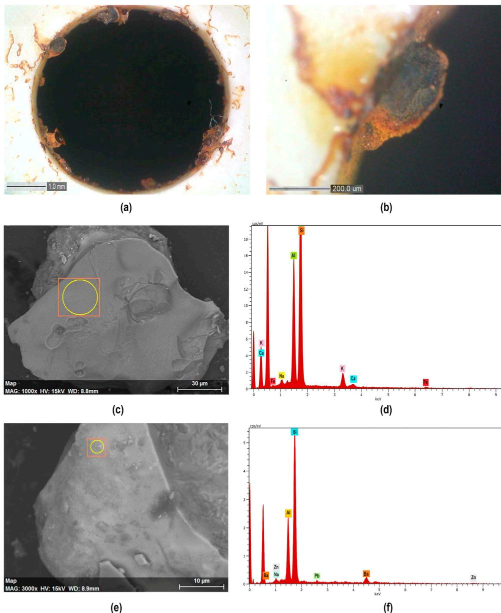
**Figure 5.** Base of the warming bowl: (a) Hole with irregular glaze edges, digital micrograph; (b) detail of the sampled area (sample CDF1); (c) SEM micrograph and (d) EDS microanalysis of the body; (e) SEM micrograph and (f) EDS microanalysis of the glaze edge. The investigated areas are indicated with a circle inside a square.
