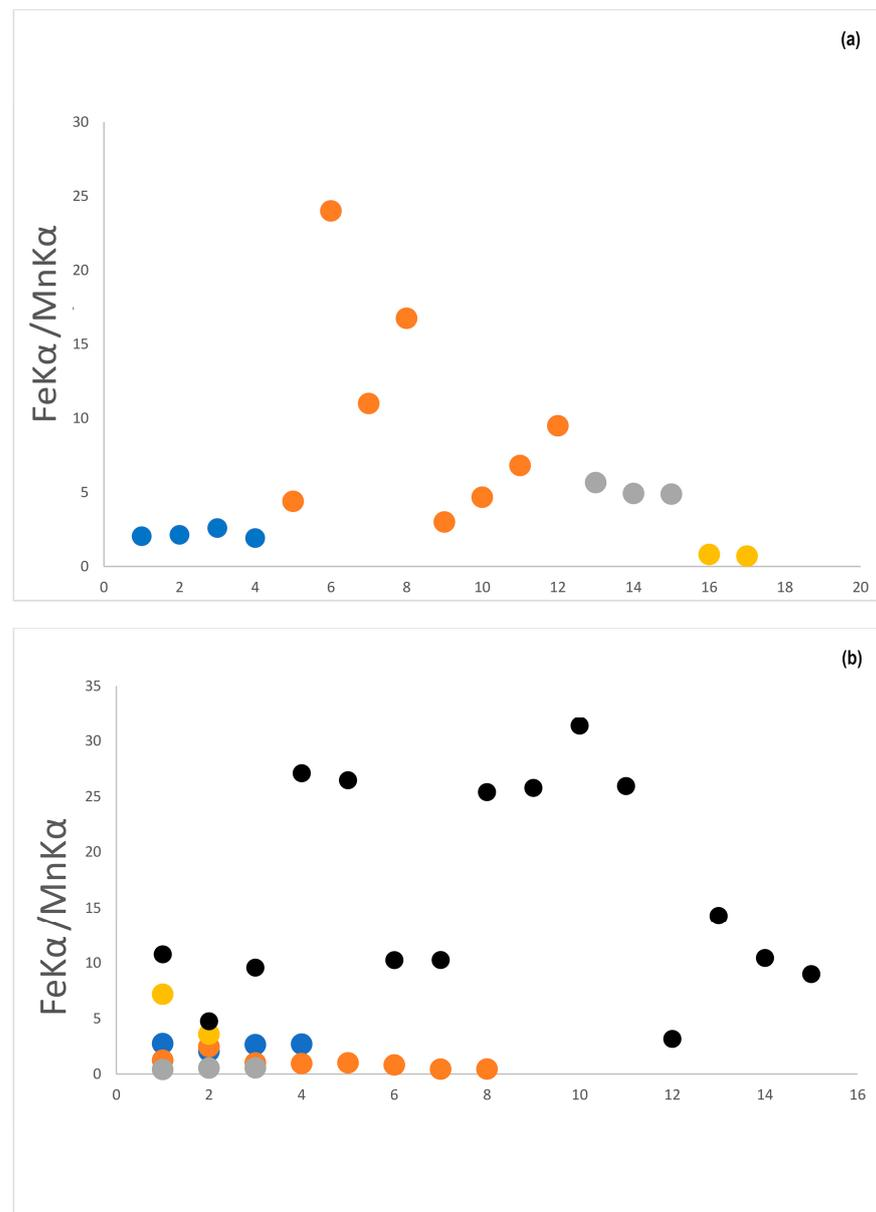
**Figure 4.** Ratios between the intensities of (a) MnK $\alpha$  and CoK $\alpha$  lines; (b) FeK $\alpha$  and MnK $\alpha$  lines for the blue mark of warming bowl (solid blue circle) obtained by ED-XRF analysis, compared with the data of You and Miao [9] (solid black circles), Wood [13] (solid yellow circles), Wen et al. [14] (solid orange circles), Feng and BaoRu [15] (solid grey circles).
