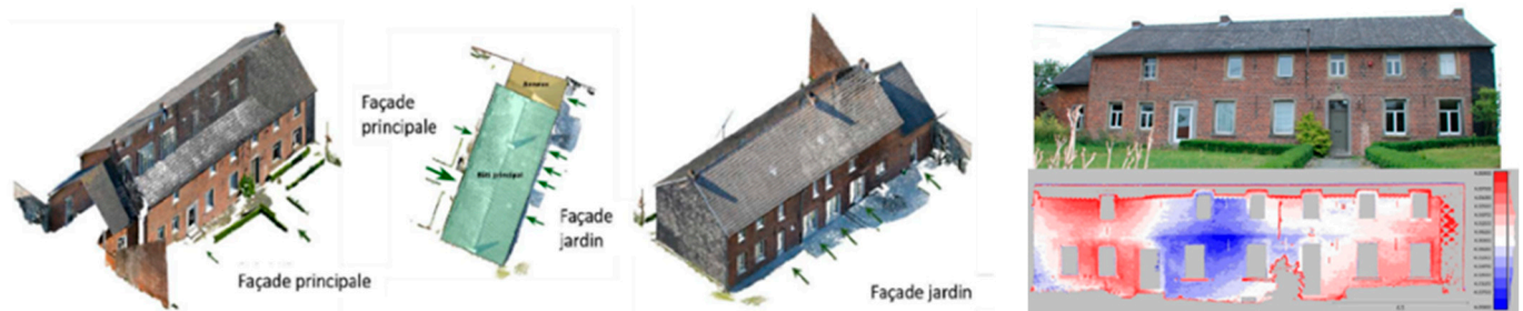
Figure 4. 3D surveying techniques allowed the collection of a large quantity of technical data. Source: Unit Building Performances & Renovation, Buildwise—S. Dubois [72,82].
