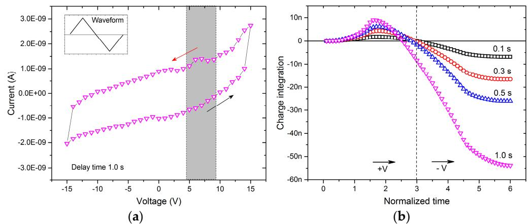
**Figure 5.** Current–voltage characteristic of the sample, arrows indicate the direction of voltage application, delay time 0.1 s (a). Dependence of the integral charge, normalized by time, measured with different delay times 0.1, 0.3, 0.5, 1.0 s (b).
