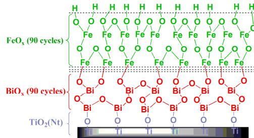
**Figure 1.** Scheme of atomic layer deposition of a heterostructure in the  $\text{BiO}_x/\text{FeO}_x/\text{TiO}_2(\text{Nt})/\text{Ti}$  system.
