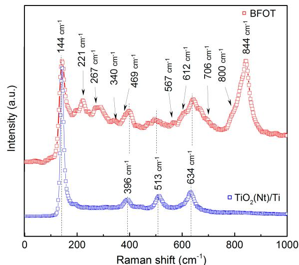
**Figure 4.** Raman spectra of the nanotube substrate (bottom) and the BFO film (top).
