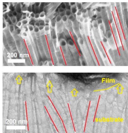
**Figure 6.** SEM image of nanotubes before (**top**) and after (**bottom**) deposition of the BFO film, the lines show how the  $\text{TiO}_2$ (Nt) nanotubes are deformed.
