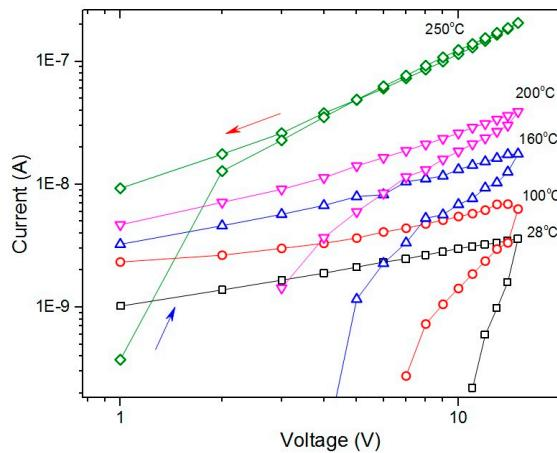
**Figure 8.** Current-voltage characteristics on a logarithmic scale at various temperatures, delay time  $t = 0.1$  s.
