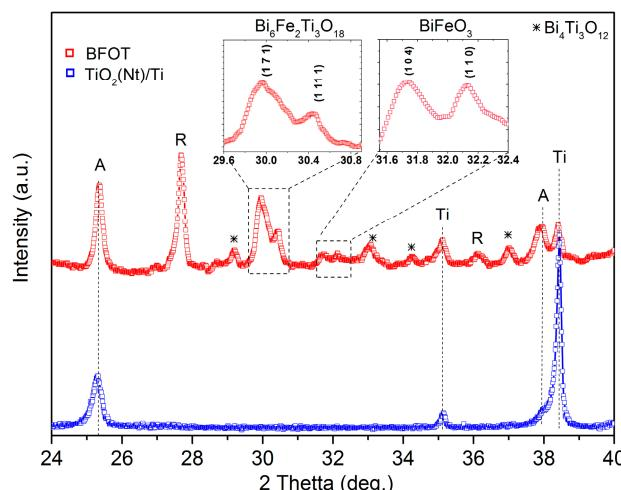
**Figure 3.** XRD patterns of  $\text{TiO}_2(\text{Nt})/\text{Ti}$  (**bottom**) and BFOT (**top**). A—anatase; R—rutile; Ti—titanium; \*— $\text{Bi}_4\text{Ti}_3\text{O}_{12}$ ; the tabs show the phases  $\text{Bi}_6\text{Fe}_2\text{Ti}_3\text{O}_{18}$  and  $\text{BiFeO}_3$ .
