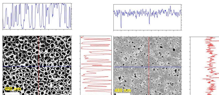
**Figure 2.** SEM of surfaces before and after application of BFO film, vertical and horizontal profile along a line showing the closure of almost all pores.
