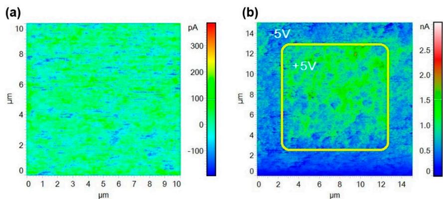
**Figure 7.** PFM of the film surface without applying voltage (a). When applying voltage 5V and  $-5\text{V}$  (b).
