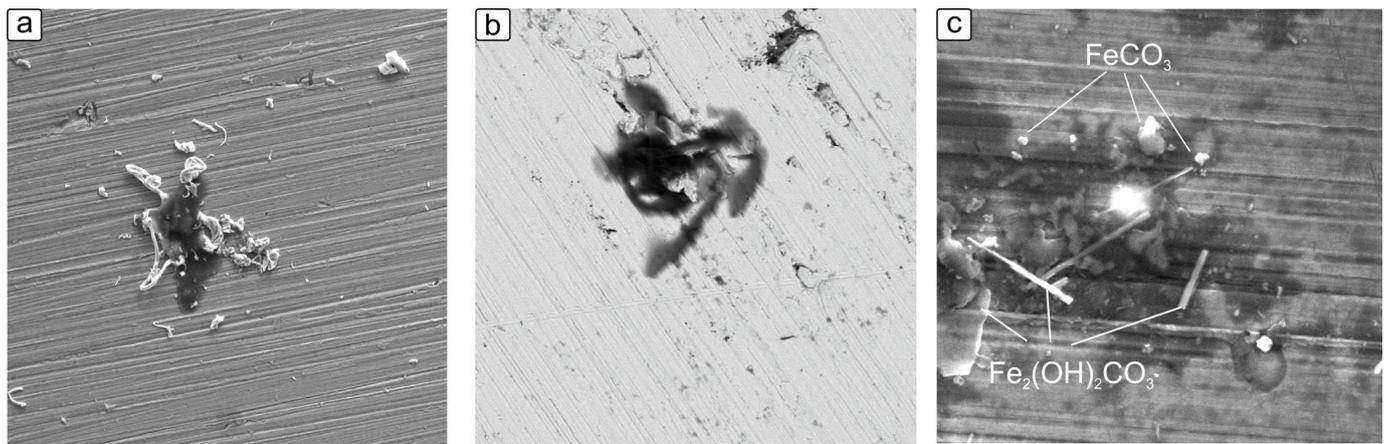
**Figure 11.** Indicative SEM images for (a) salt precipitation, (b)  $\text{FeCO}_3$  nodules and (c) plate-like corrosion products ascribed to  $\text{Fe}_2(\text{OH})_2\text{CO}_3$  phase.
