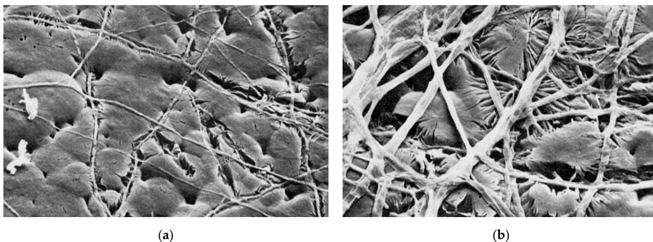
**Figure 4.** SEM image of *Penicillium funiculosum* mycelium degrading polycaprolactones (a) biodegradation of amorphous regions, (b) complete degradation of amorphous regions and partial degradation of crystalline phase. Adapted from [54] with permission from John Wiley and Sons.
