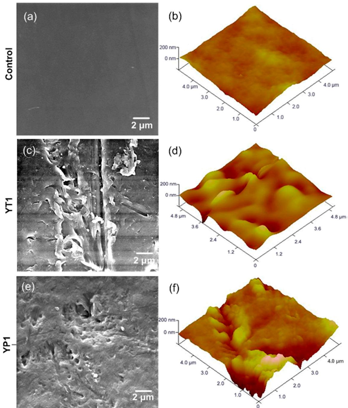
**Figure 5.** Combined SEM and AFM techniques for characterization of the biodeterioration of polyethylene sheets after 28 days, (a,b) SEM and AFM images of the sterile control sample, (c,d) SEM and AFM images of the specimens degraded by *Bacillus* strain YT1, (e,f) SEM and AFM images of the specimens degraded by *Bacillus* strain YP1. Adapted with permission from [47] the American Chemical Society, copyright 2014.
