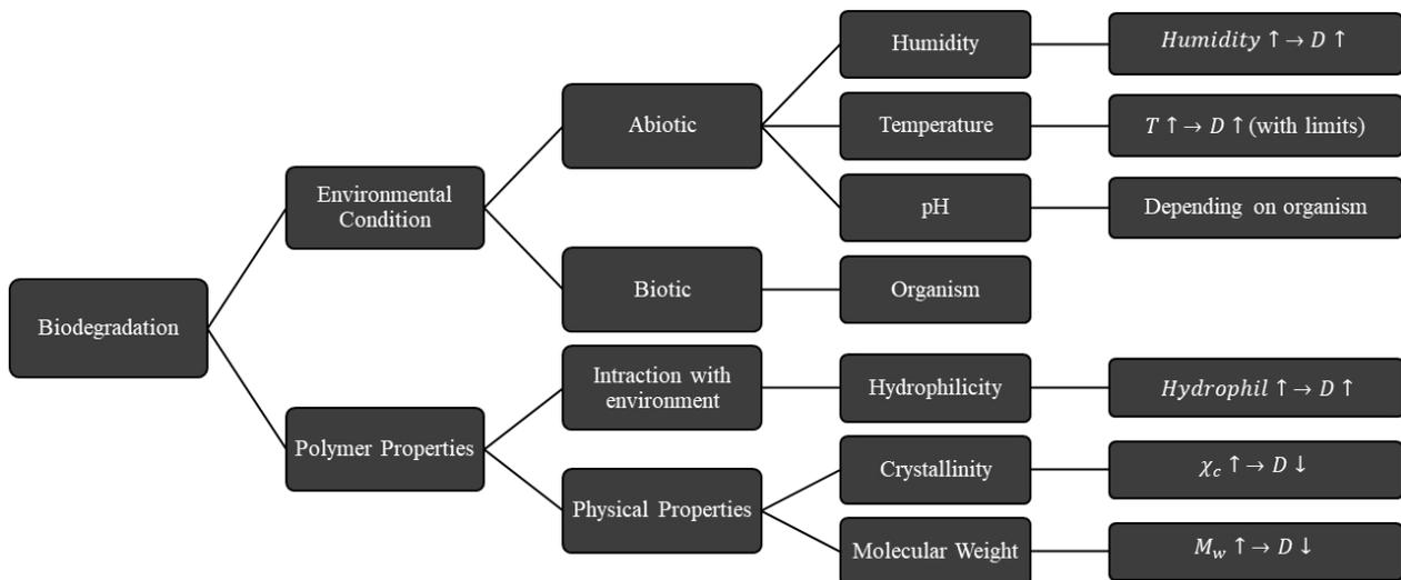
**Figure 2.** Factors affecting biodegradation of polymers, *D*: degradation,  $\chi_c$ : crystallinity,  $M_w$ : molecular weight.
