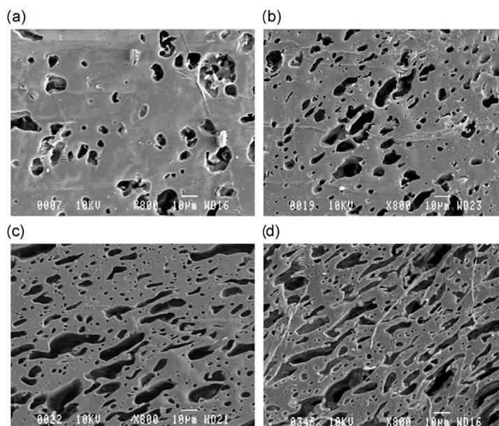
**Figure 6.** SEM image of PLA/TPS blends after 14 weeks incubation: (a) 80/20, (b) 70/30, (c) 60/40, and (d) 50/50. Adapted with permission from [52] John Wiley and Sons, copyright 2011.
