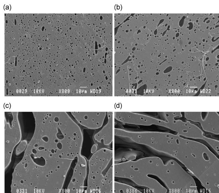
**Figure 7.** SEM image of LDPE/TPS blends after 14 weeks incubation: (a) 80/20, (b) 70/30, (c) 60/40, and (d) 50/50. Adapted with permission from [52] John Wiley and Sons, copyright 2011.
