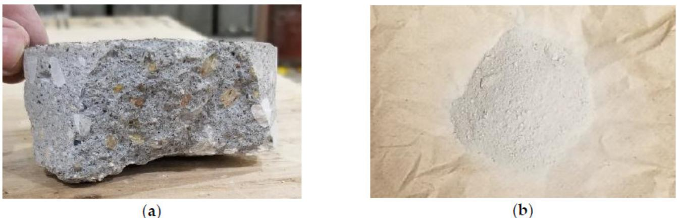
**Figure 4.** (a) Extracted core from the concrete specimen; (b) Concrete sample in pulverized form.
