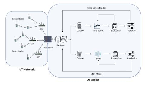
Figure 3. Overall DXN showing the "AI Engine" and the "IoT Network" blocks.
