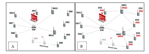
**Figure 2.** (**A**) The implemented IoT network deployment, (**B**) The same deployment with the bridging algorithm.
